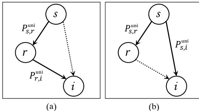
**Figure 4.2:** Possible connection available to communicate with node  $i$ : (a) unicast solution; (b) multicast solution.
