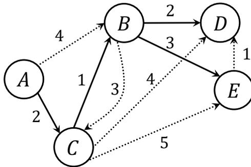
**Figure 3.2:** Dijkstra's algorithm application: non-dashed edges represent the shortest-path tree.
