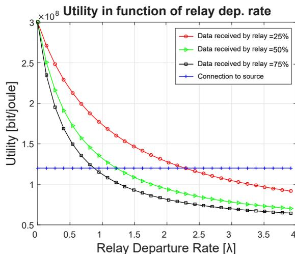
**Figure 4.13:** Utility that the new node  $i$  would get in function the departure rate of the relay node  $r$ . The straight line represents the utility that the child node  $i$  would get by selecting the source  $s$  as its parent node.
