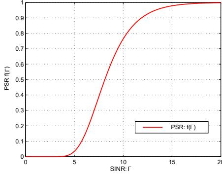
**Figure 4.9:** Packet Success Rate as a function of SINR
