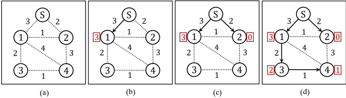
**Figure 3.4:** Mechanism Design with Potential Game for Energy-Efficient Data Dissemination in D2D Networks: (a) step 1: analyzing network scenario; (b) step 2: costs computation and  $S \rightarrow 1$  association; (c) step 3:  $S \rightarrow 2$ ; (d) final broadcast tree,  $1 \rightarrow 3$  and  $3 \rightarrow 4$ .
