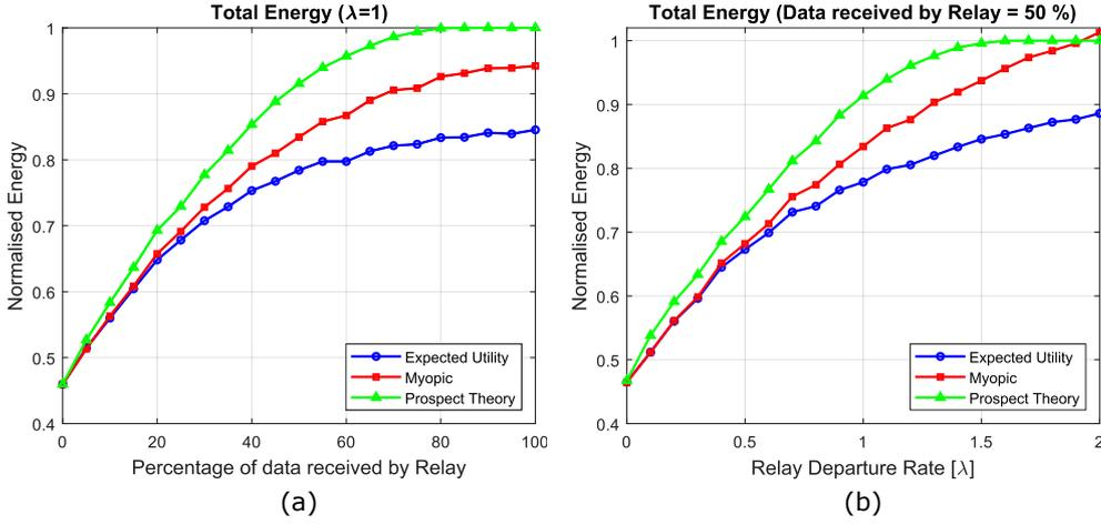
**Figure 6.2:** Total transmit energy in the network normalized by the energy spent if both the new agent select the fixed source as parent node.
