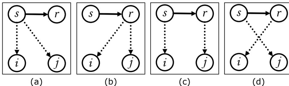
**Figure 5.1:** System model with all possible transmission scenarios for the two new vertices  $i$  and  $j$ . (a): multicast connection from the source node  $s$ ; (b): multicast connection from the relay node  $r$ ; (c) and (d): unicast connections when two different parent nodes are selected.
