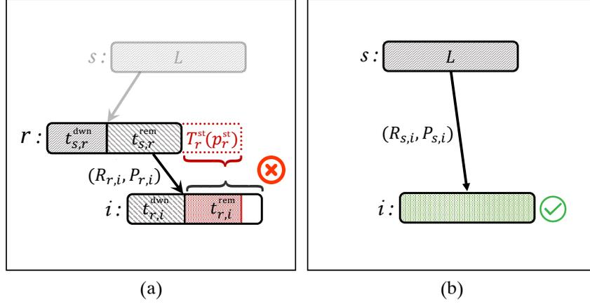
**Figure 4.7:** Failure: (a) node  $r$  leaves the network before the time needed to accomplish the whole transmission with node  $i$ ; (b) a new connection with the source  $s$  must be established to allow the message to be received.
