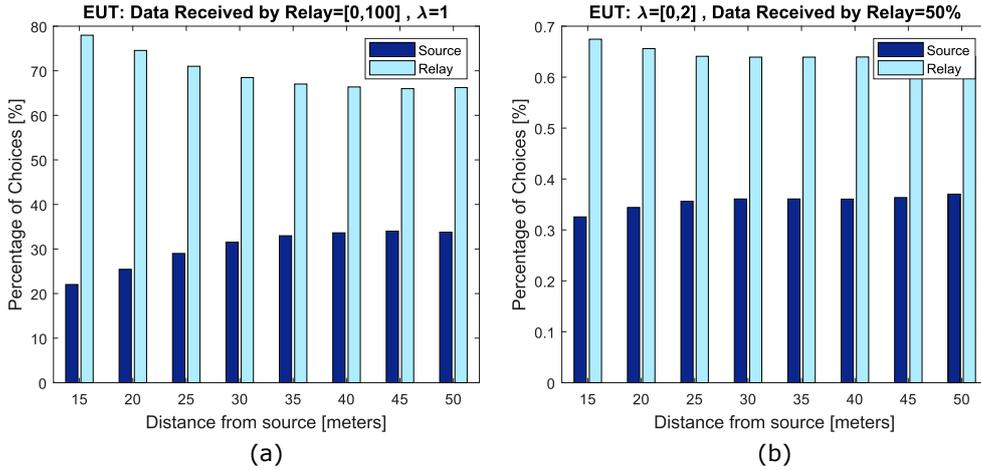
**Figure 6.5:** Number of times the passive users (decision based on EUT) select node  $s$  or node  $r$  for receiving the message in function of the distance from the fixed source.
