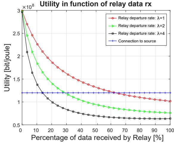
**Figure 4.12:** Utility that the new node  $i$  would get in function of the data received by the relay node  $r$ . The straight line represents the utility that the child node  $i$  would get by selecting the source  $s$  as its parent node.
