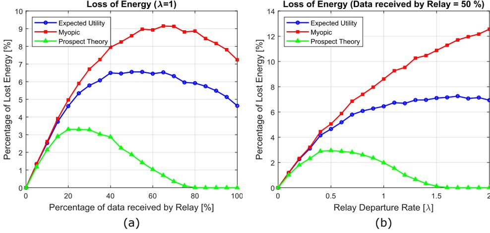
**Figure 6.4:** Energy loss, caused by the relay node departure, with respect to the total transmit energy in the network.
