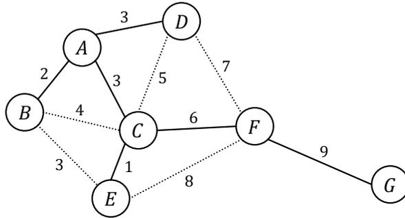
**Figure 3.1:** Minimum Spanning Tree application: non-dashed edges represent the final shape of the tree
