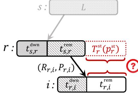
**Figure 4.5:** Transmission times between node  $r$  and node  $i$ . Red indicates the additional probabilistic time the relay remains in the network after its full reception. The question mark indicates the uncertainty over the duration of that time.
