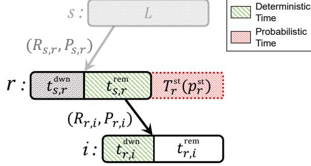
**Figure 4.11:** Transmission times between node  $r$  and node  $i$ . Red indicates the additional probabilistic time the relay remains in the network after its full reception. Green indicates the time needed by node  $r$  to complete its reception, which correspond to the period it will surely remain in the system.
