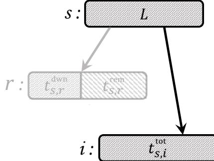
**Figure 4.8:** Selection of the source for receiving the message. The relay is present in the network, but it is put in background because it does not participate in the dissemination.
