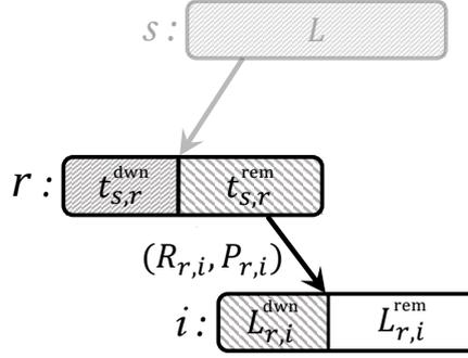
**Figure 4.4:** Selection of the relay  $r$  for receiving the message. The source is present in the network, but it is put in the background because node  $i$  does not receive information from  $s$ .
