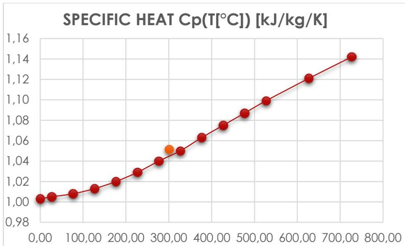
**FIGURE 15 SPECIFIC HEAT AT CONSTANT PRESSURE FOR THE AIR VARYING WITH TEMPERATURE. THE MEAN VALUE USED FOR THE MASS FLOWRATE CALCULATION IS SHOWN IN THE GRAPH.**
