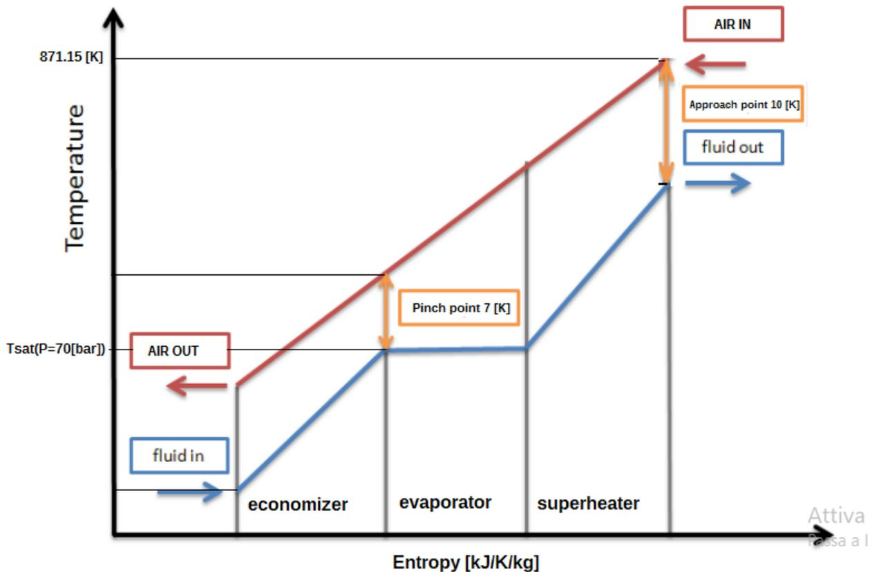
**FIGURE 20 PINCH POINT SCHEME.**
