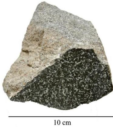
**FIGURE 5 A SAMPLE OF DIABASE WITH A POLISHED SURFACE ON ONE SIDE; THE WHITE MINERALS ARE PLAGIOCLASE FELDSPAR AND THE BLACK ARE CLINOPYROXENE.<sup>10</sup>**
