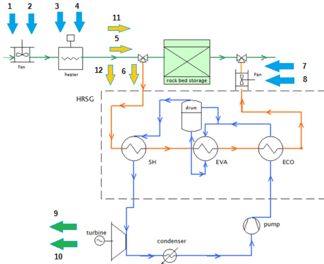
**FIGURE 106 ENERGY FLUXES INVOLVED IN OPTIMIZATION ALGORITHM. 1ST OPTION, ONLY ELECTRICITY PRODUCTION.**
