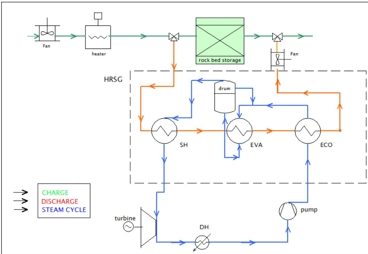
**FIGURE 12 TYPE TWO - SIMPLE STEAM TURBINE AND STEAM TURBINE WITH DISTRICT HEATING IN DISCHARGE PHASE.**
