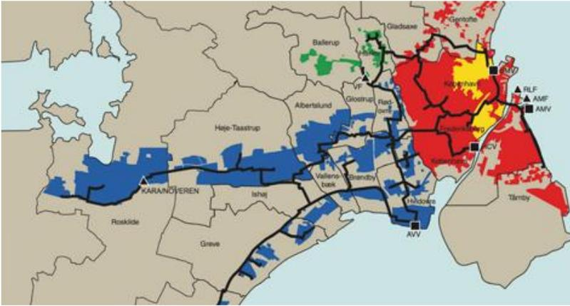
**FIGURE 86: THE GREATER COPENHAGEN DH SYSTEM (REFERENCE - REGULATION AND PLANNING DISTRICT HEATING IN DENMARK)**
