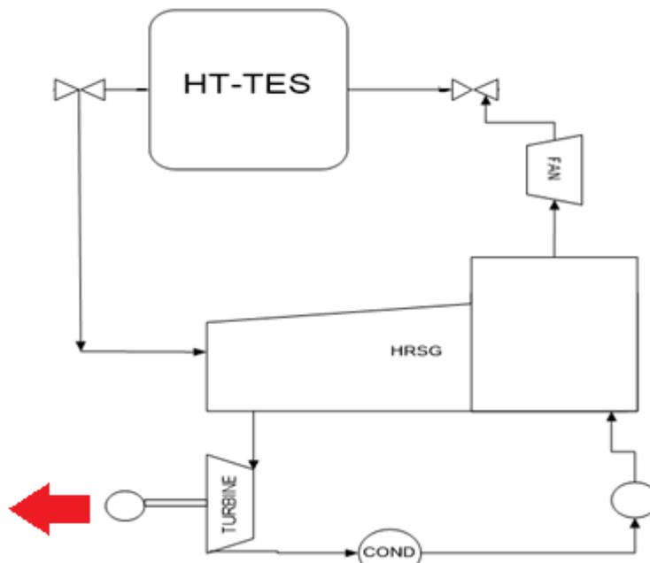
**FIGURE 21 1<sup>ST</sup> OPTION DISCHARGE PHASE SCHEME**
