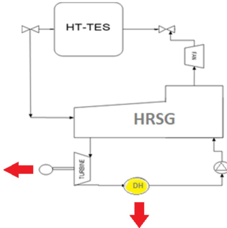
FIGURE 23 2<sup>ND</sup> OPTION DISCHARGE PHASE SCHEME.
