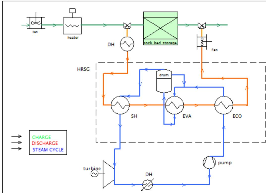
**FIGURE 13**TYPE THREE - SIMPLE STEAM TURBINE AND STEAM TURBINE WITH DISTRICT HEATING AND HEAT EXCHANGER FOR DISTRICT HEATING IN DISCHARGE PHASE.
