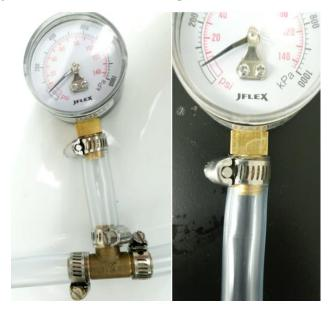
Figure 17: Pressure meter sub-assembly.
