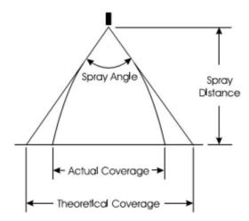
Figure 15: Actual vs theoretical coverage area (Relab Spray & Purification Technology Ltd.).
