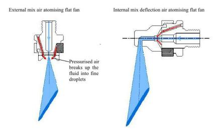
*Figure 12: External (left) vs internal (right) mixing nozzles (SNP the Spray Nozzle People, retrievable at: http://www.spray-nozzle.co.uk/spray-nozzles/air-atomising-nozzles/external-mix-variant).*
