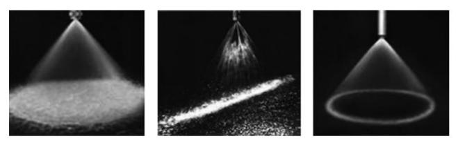
Figure 13: Full cone, flat fan and hollow cone. Respectively from left to right.
