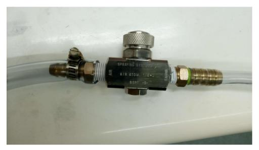
Figure 18: Spraying System Co. Air atomising nozzle used for the experiments.
