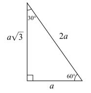
Figure 14: Spray aperture angle, one side. Note that the nozzle is supposed to be at the top of the triangle, and that the real spray shape will be the cone obtained by revolving the above image around its vertical axis.
