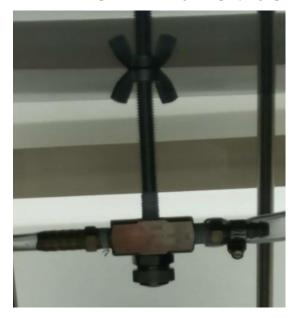
Figure 16: Threaded rod and nozzle used in the prototype.
