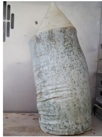
Figure 5.7: M5 - collapsed frozen sample
