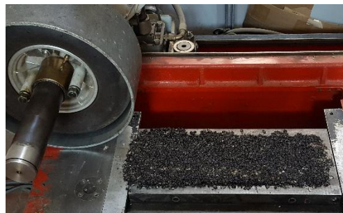
Figure 5.10: Slab compaction problem
