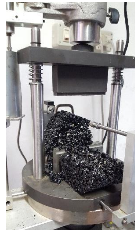
Figure 4.5: M4 - ITS test failure
