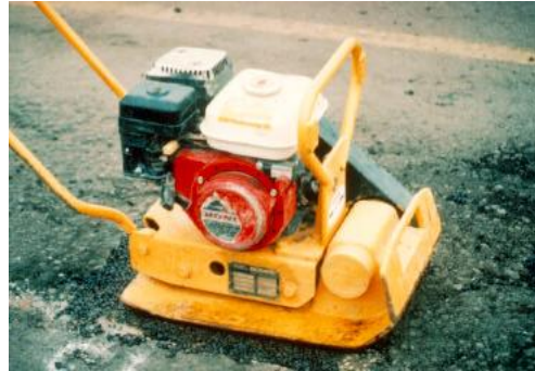
Figure 2.8: Semi-permanent procedure, compaction - Wilson P & Romine R, 2001
