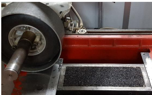
Figure 5.9: Slab well compacted
