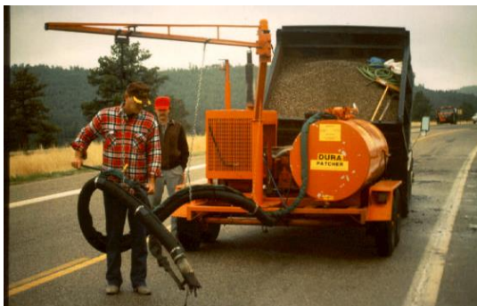
Figure 2.9: Spray-injection device, truck and trailer unit - Wilson P & Romine R, 2001
