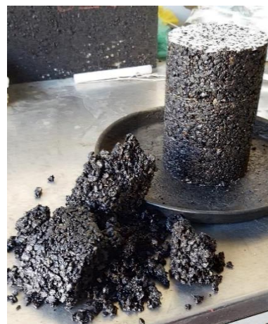
Figure 5.5: M5 - collapsed sample
