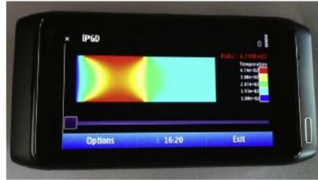
FIGURE 1.7: Online phase: the user is able to choose the temperatures  $\theta_1$  and  $\theta_2$  and get in real time the temperature in any point of the system [8].
