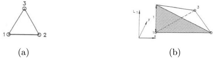
FIGURE 3.1: (a) Linear triangular element, (b) Shape function  $N_1^e$  of a triangular element.
