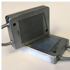
Figure A.2: A planar fuel cell
