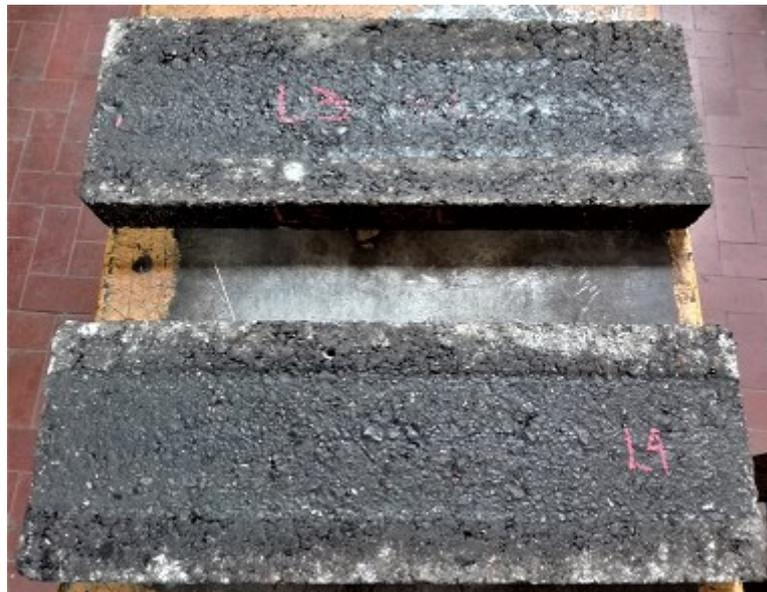
Figura 4-8: Lastre L<sub>3</sub> e L<sub>4</sub> dopo Wheel Tracking Test a 40°C
