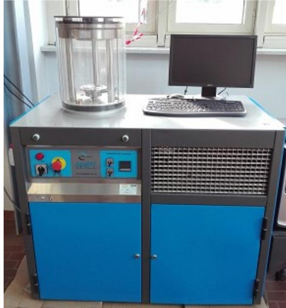
Figura 3-24: Asphalt Mixture Performance Tester
