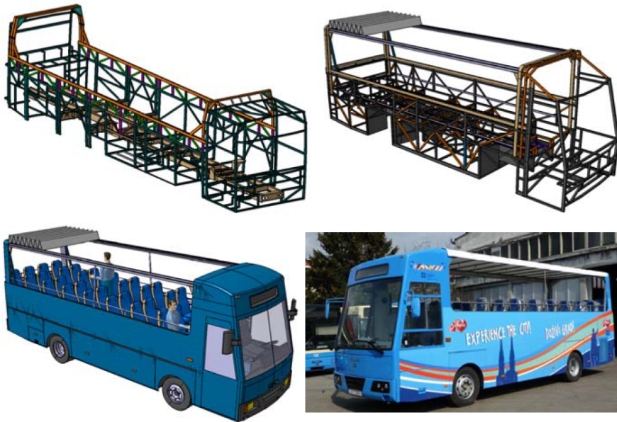
Figure 1.3: The space frame and the design solution of the panoramic bus for city sightseeing.
