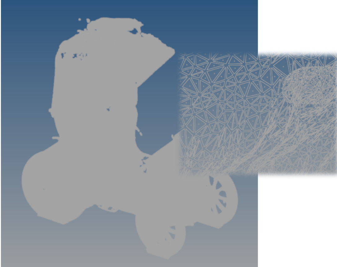
Figure 3.1: Imported model from PhotoScan to HyperMesh, with zoom to see triangular division of surface.
