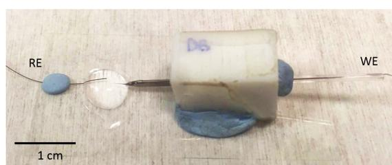
**Fig. 3.4 Customised coverslip set-up:** the custom-made PTFE holder is secured on a glass coverslip, containing a droplet of KCl, within a glue boundary, hosting the RE. The tip penetrates the KCl droplet, and the open barrel, where the WE is placed, is filled with the solution of DNA and KCl.
