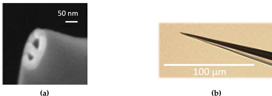
**Fig. 4.1 Characterisation of the fabricated dual-barrel nanopipettes, before and after pyrolytic carbon deposition:** (a) SEM image highlighting the two pores at the tip of a plain dual-barrel nanopipette; (b) Bright-field optical micrograph of the pipette after carbon deposition, demonstrating the successful deposition within one barrel (shown in black), while the other remains unmodified.
