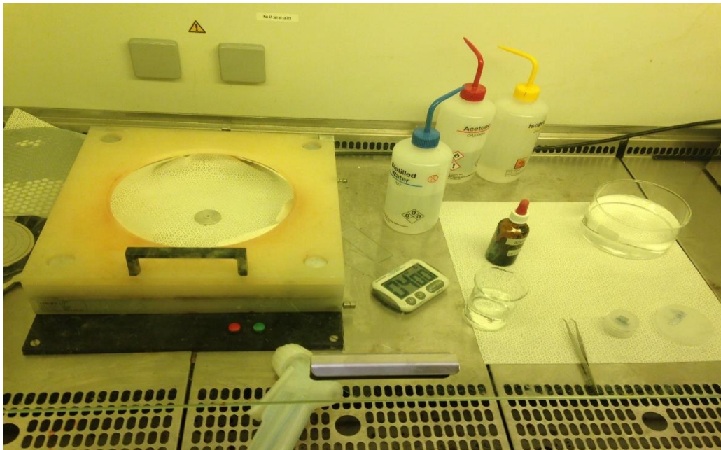
Figure15: spin coating tool and the plastic gun are placed inside the LAF-HOOD
