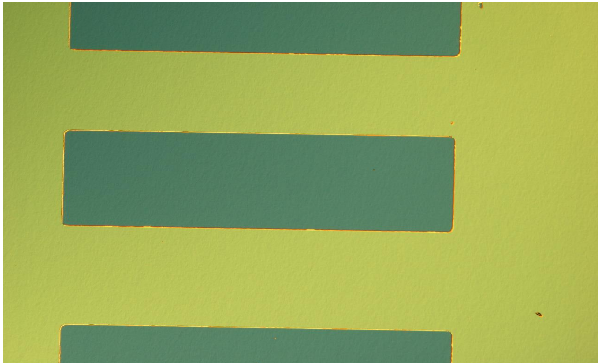
Figure 19: Optical microscopy from the lifted-off sample deposited by titanium and gold, the windows for etching selection are colored in dark green, the background
