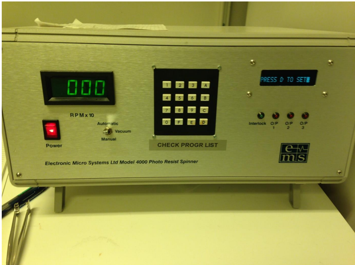
Figure 14: spin coater programming system for adjusting the speed and modules of rotation
