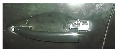
Figure 7 Damages to door lock
