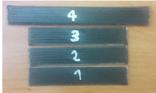
Figure 4.13. 0 ° carbon fiber specimens for 3pb test.
