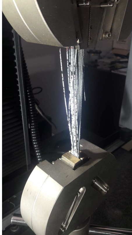
Figure 5.2. Carbon fiber specimen after traction test.
