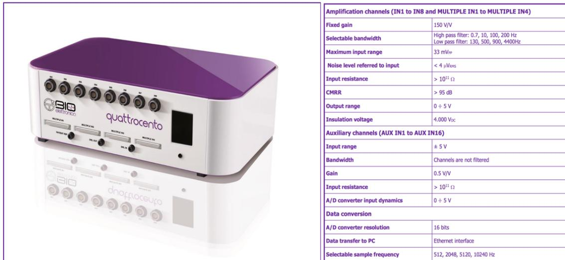
Figure 15: Quattrocento amplifier for the acquisition of surface/intramuscular monopolar or bipolar EMG signals and technical specifications. Taken from [15]
