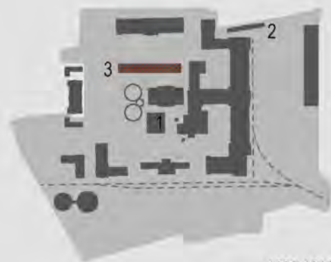
1909-1914 1. smithy was redesigned; was added 2nd floor for rectification dep. (1909-1911); 2. fence (1914); 3. redesigned for urotropin factory; pond buried
