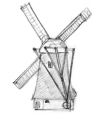
Dutch mill with a revolved cup
