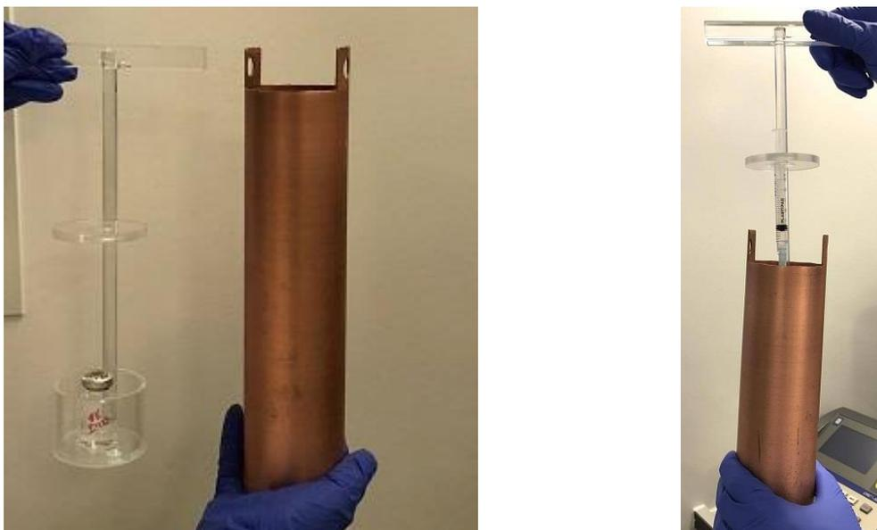
*Fig. 16 Copper filters for Capintec CRC 55tR, used to test the effect of the copper in the reduction of geometric effect on the sample due to its capacity to absorb mostly low energy photons.*
