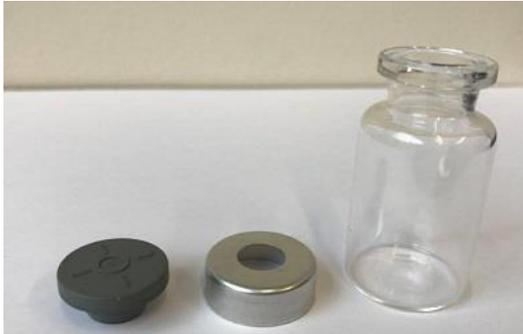
Fig. 10 - 10R Type 1+ Schott 10 ml vial, plastic and Al caps
