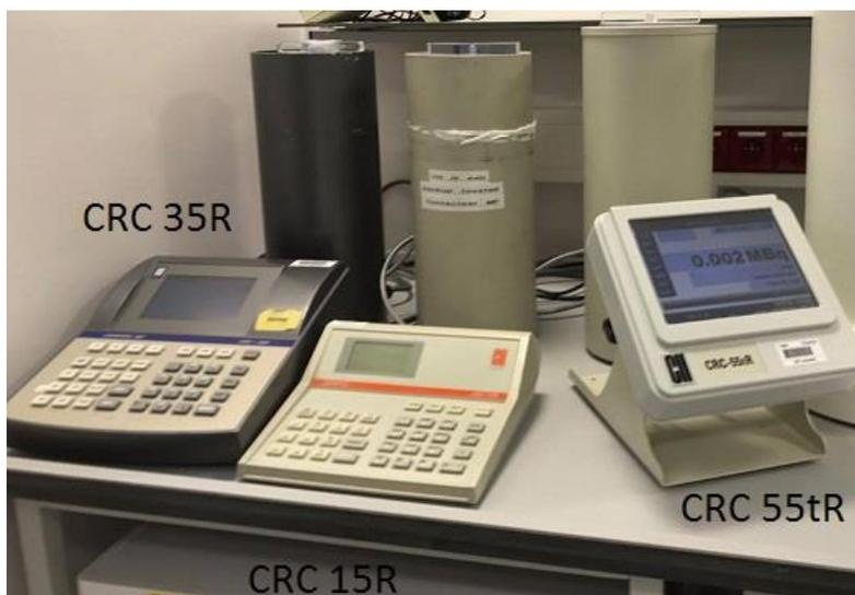
Figura 6 – Capintec RCs available in UZ Leuven in a medical room. From the left: CRC-35R RC, CRC 15R RC and CRC-55tR RC
