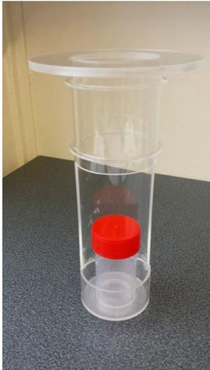
Fig. 8 – Perspex holder for NPL Fidelis Secondary Standard RC
