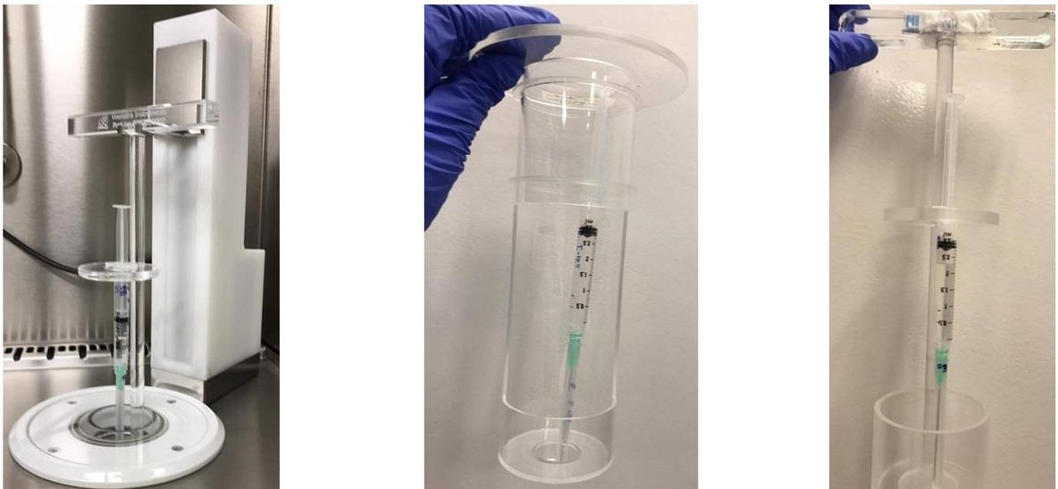
Fig. 15 Different holders for placing the sample inside the RCs. From the left 1. Plastic holder for Comecer VIK 202 RC, 2. Fidelis plastic holder, 3. Capintec plastic holder for CRC-55tR RC
