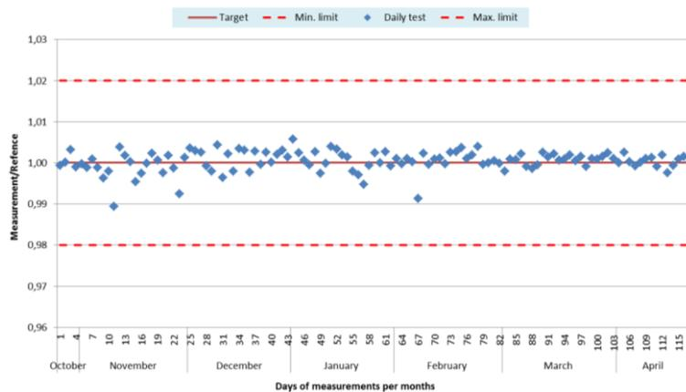
Figura 19 – Constancy test source for Fidelis, using  $^{137}\text{Cs}$  sealed source
