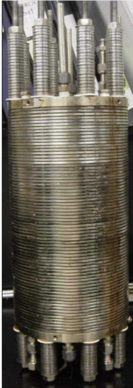
Fig 3.4- 64 cell stack tested by Nordic Power Systems AS
