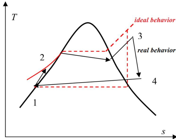
**Figure 3:** T-s diagram of an actual Rankine cycle
