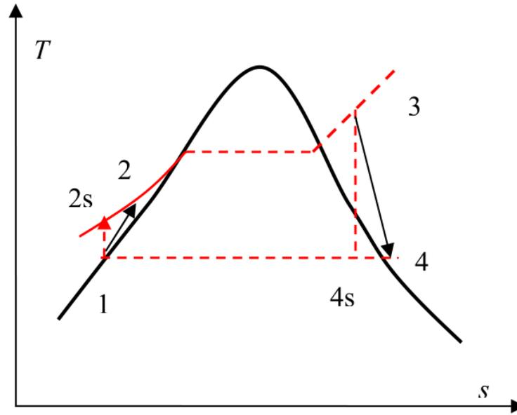
**Figure 4:** Real behavior of the pump and turbine compared to the isentropic behaviour (**Bahrami**)
