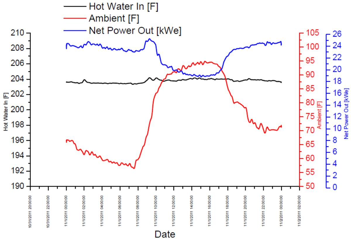
**Figure 18:** Net power output (blue); Brine inlet temperature (black); Ambient temperature (red) (kW<sub>e</sub> stands for kilowatt electric and is equivalent to kW) (ElectraTherm, 2012)
