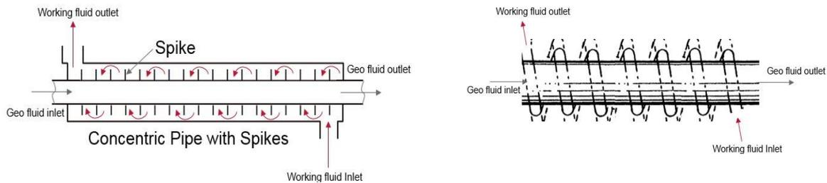
**Figure 14: Improved Designs of the Double Pipe Heat Exchanger (Falcone et al., 2017)**
