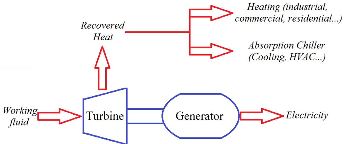
**Figure 5:** CHP configuration with heat recovered from the exit gas
