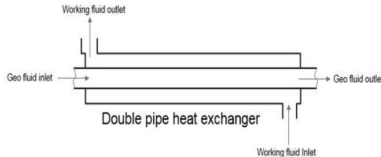
**Figure 13: Simple Clamp-on Double Pipe Heat Exchanger (Falcone et al., 2017)**
