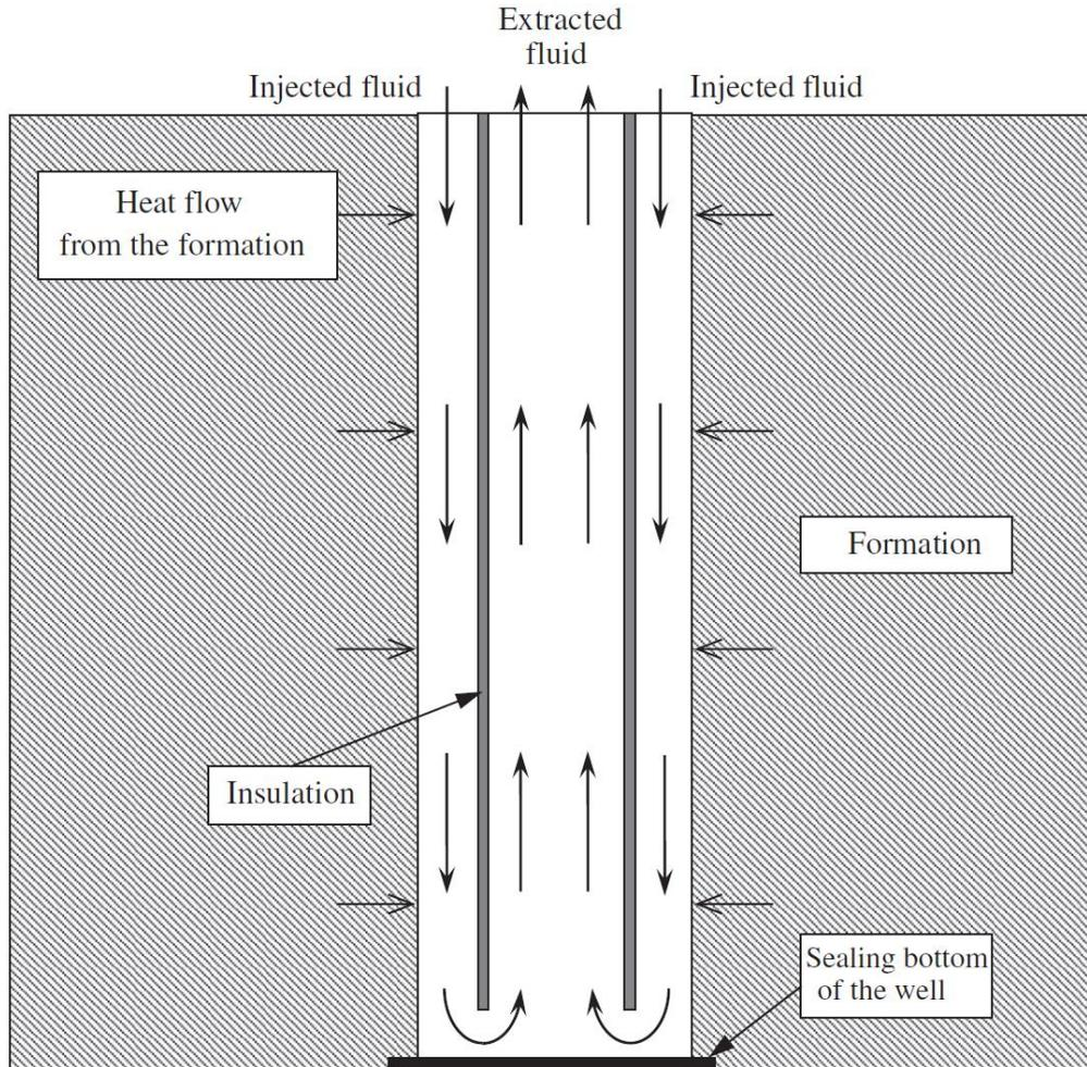
**Figure 6:** Heat extraction through a sealed abandoned well (Cheng et al., 2014)
