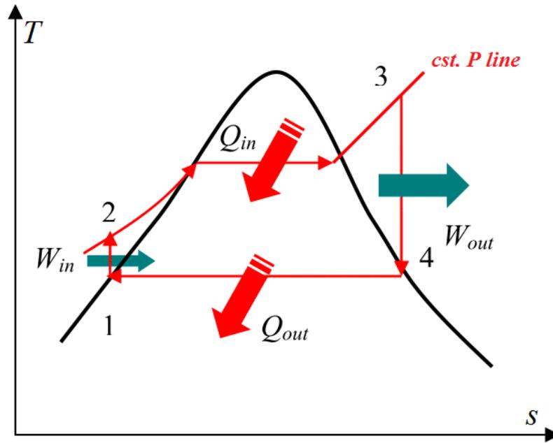
**Figure 2:** T-s diagram of an ideal Rankine cycle (**Bahrami**)
