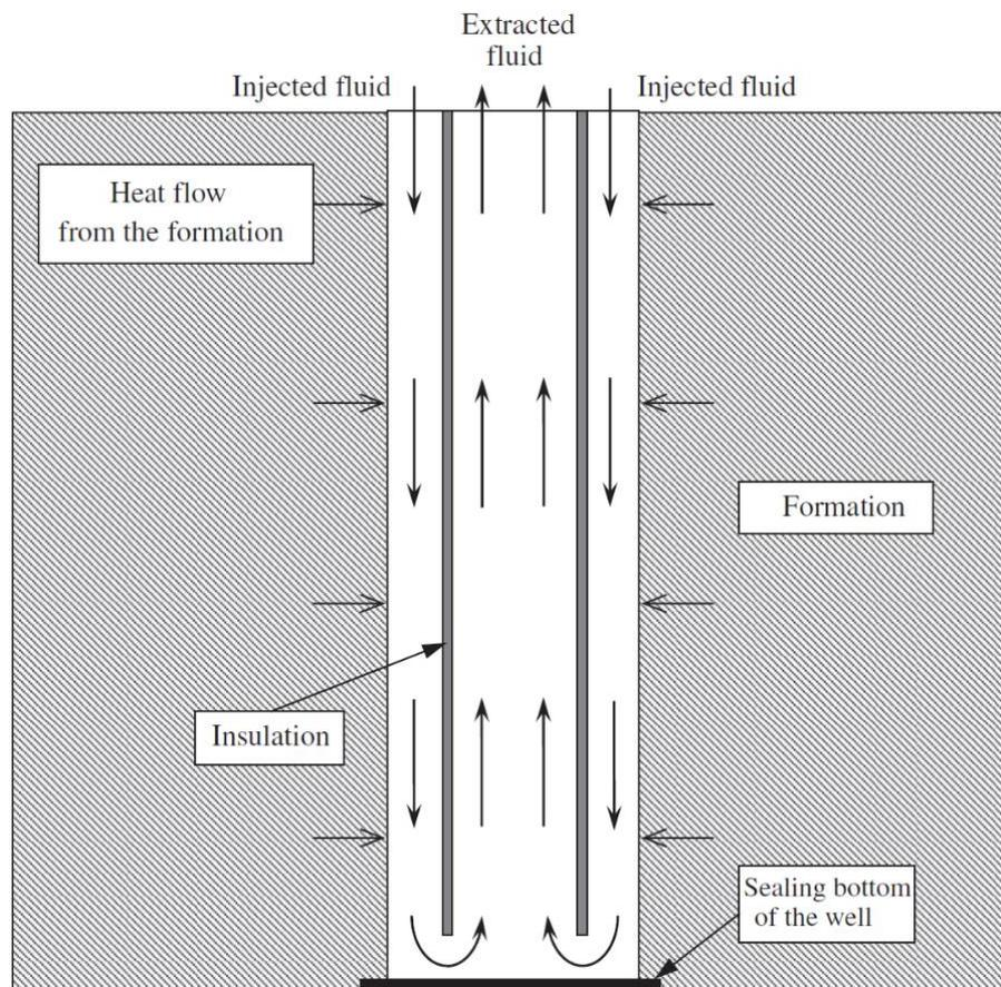
**Figure 19: Heat extraction through a sealed abandoned well (Cheng et al., 2014)**
