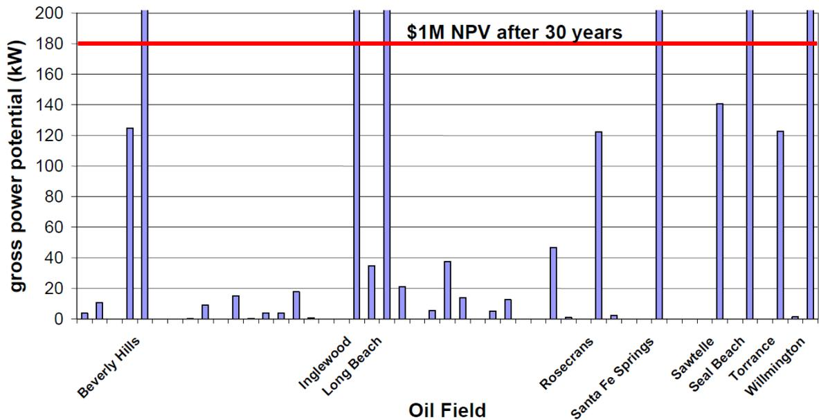
**Figure 10:** The profitability threshold for the NPV is at 1 million \$ (The graph was cut off at 200 kW to fit the smaller fields) (Bennett et al., 2012)
