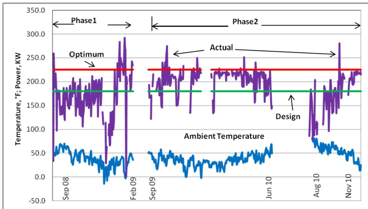
**Figure 17: Net power output (in purple) and ambient temperature (in blue) over the test duration (Johnson et al. 2011)**
