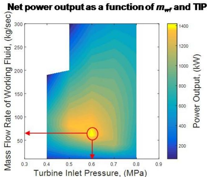
**Figure 12: Optimized TIP and Mass Flow Rate (Falcone et al., 2017)**
