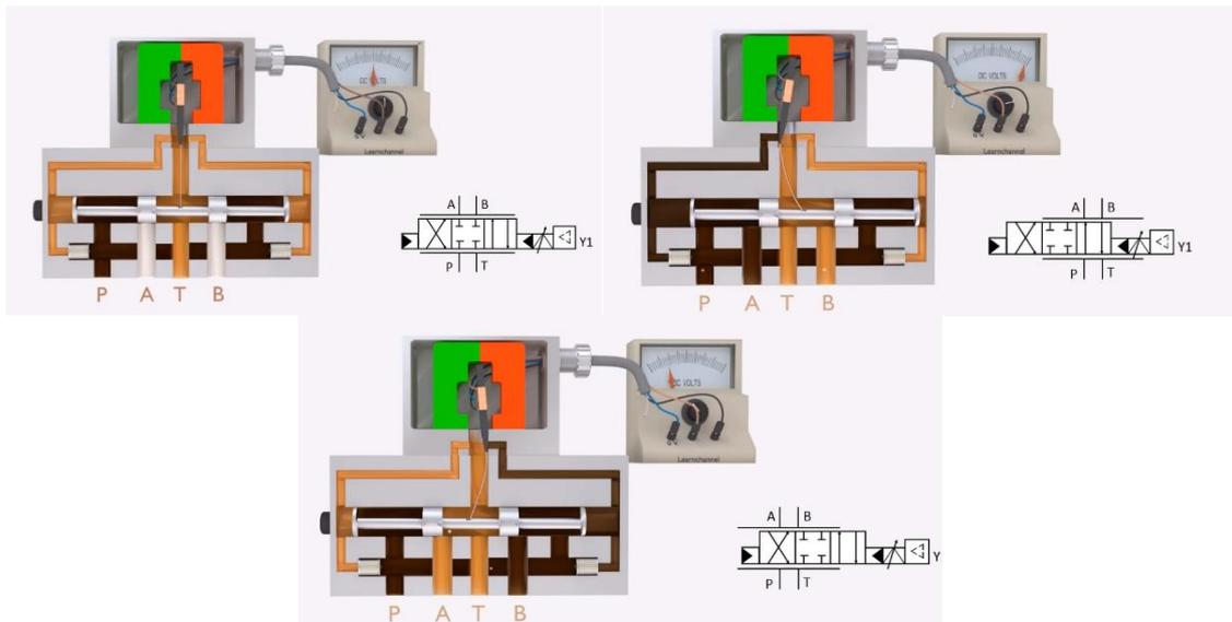
Figure 4.10 Operation scheme of a servo valve.
