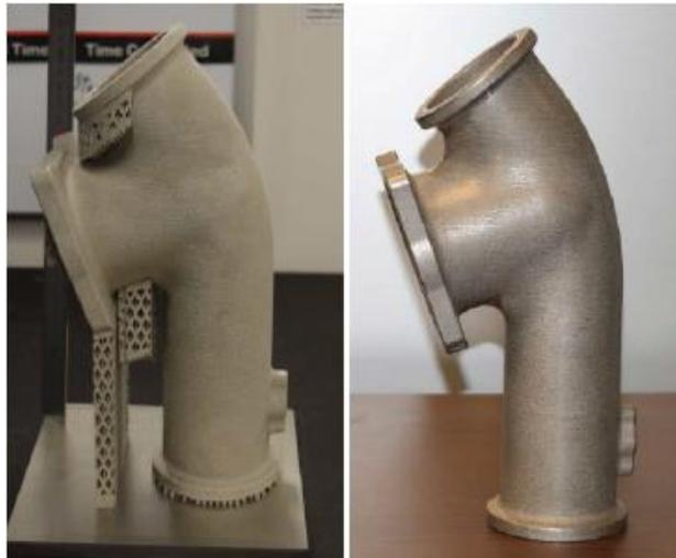
*Figure 2.10 Pre- and post-processed part printed with AM.*
