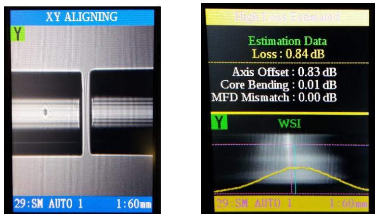
Figure 39: Splicing Process - Visualization and Estimation Loss
