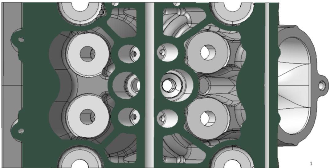
Figure 2.32: Competitor J ribs layout
