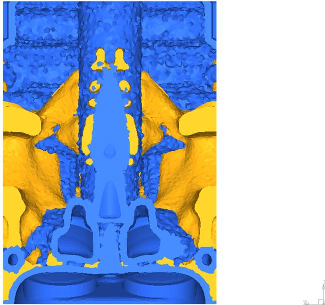
**Figure 3.9:** *Optimal shape result, with 0.35 density threshold view. XZ mid plane section view*
