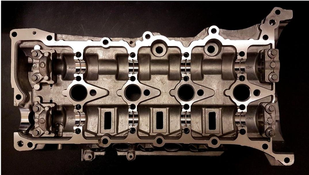
**Figure 1.7:** Top view of a cam carrier of a 2.0 litres diesel engine
