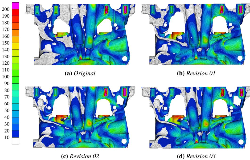
**Figure 4.11:** Hot analysis results, yz midplane section view
