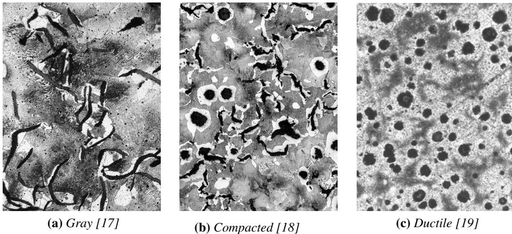
**Figure 1.10:** Different types of cast iron for cylinder head production
