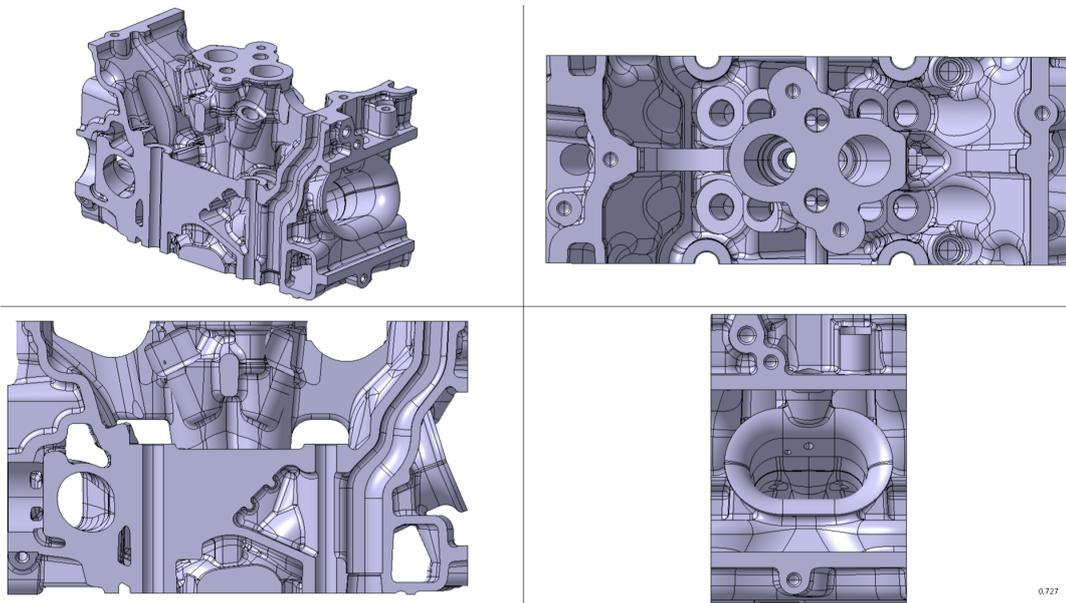
**Figure 2.25:** *Competitor H cylinder head*
