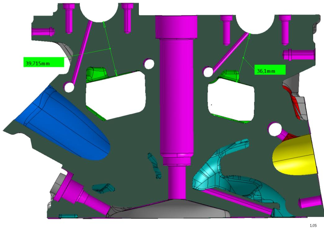
**Figure 2.15:** *Competitor D camshaft bridge section view*
