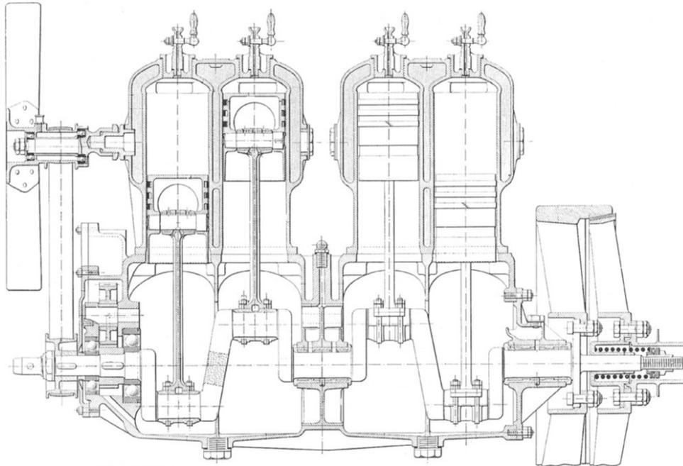
**Figure 1.3:** A four cylinders engine of the 1910s featuring two blocks, with cylinders and head obtained in a single cast piece. [6]
