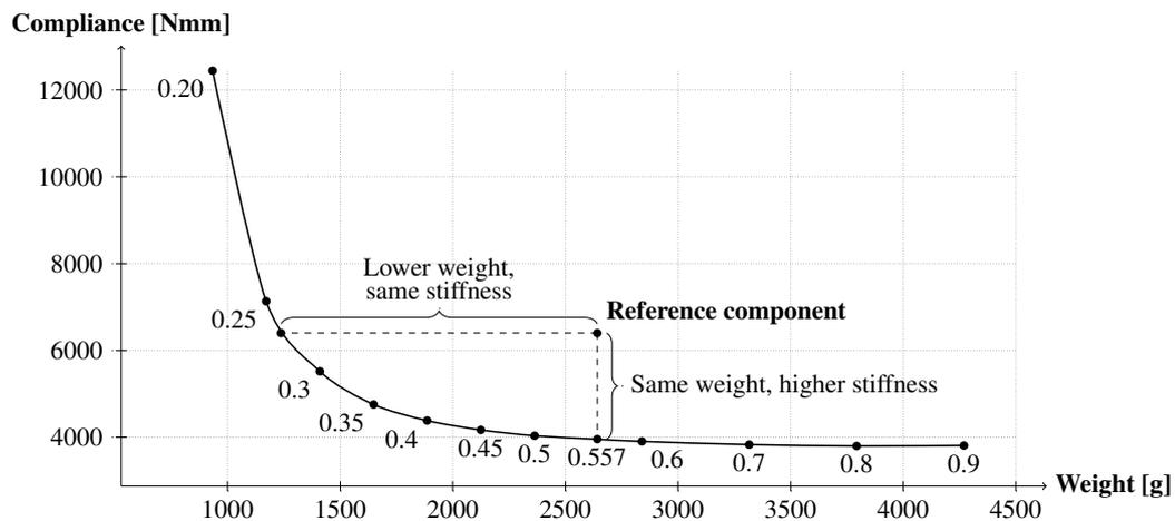
**Figure 3.6:** Optimum optimization curve, with each point labelled with the maximum mass fraction of the overall component
