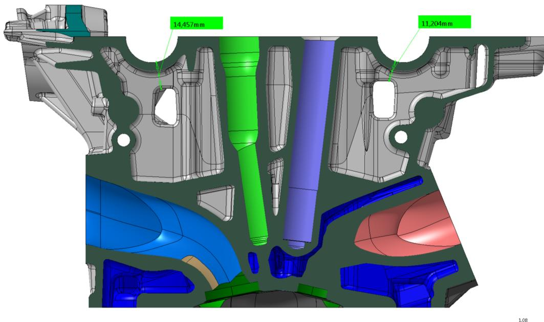
**Figure 2.9:** *Competitor B camshaft bridge section view*
