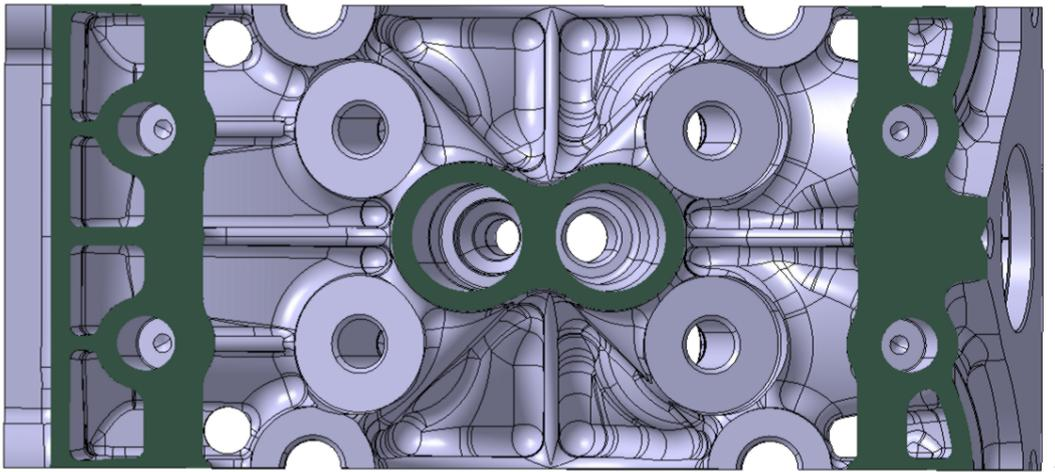
**Figure 2.2:** Reference ribs layout
