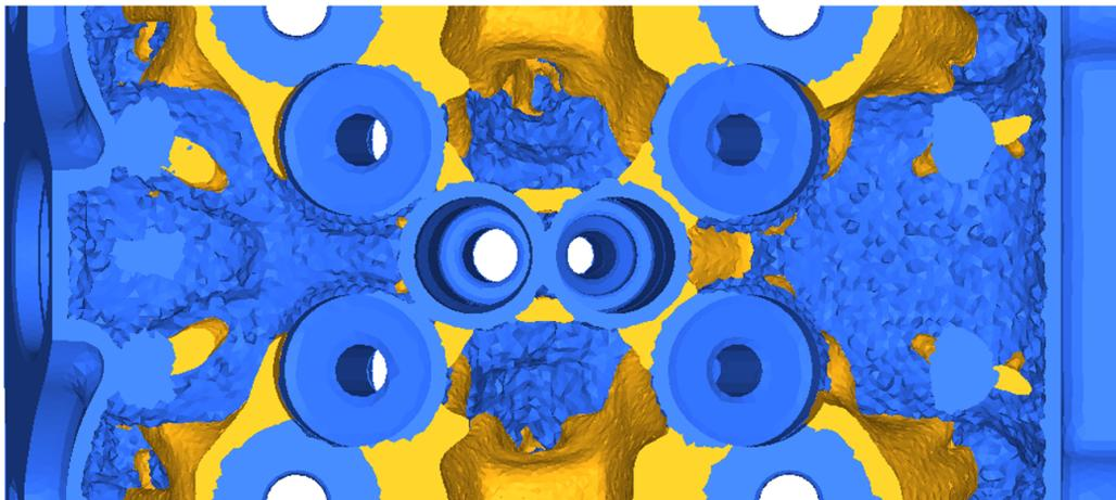
**Figure 3.10:** *Optimal shape result, with 0.35 density threshold view. XY mid plane section view*
