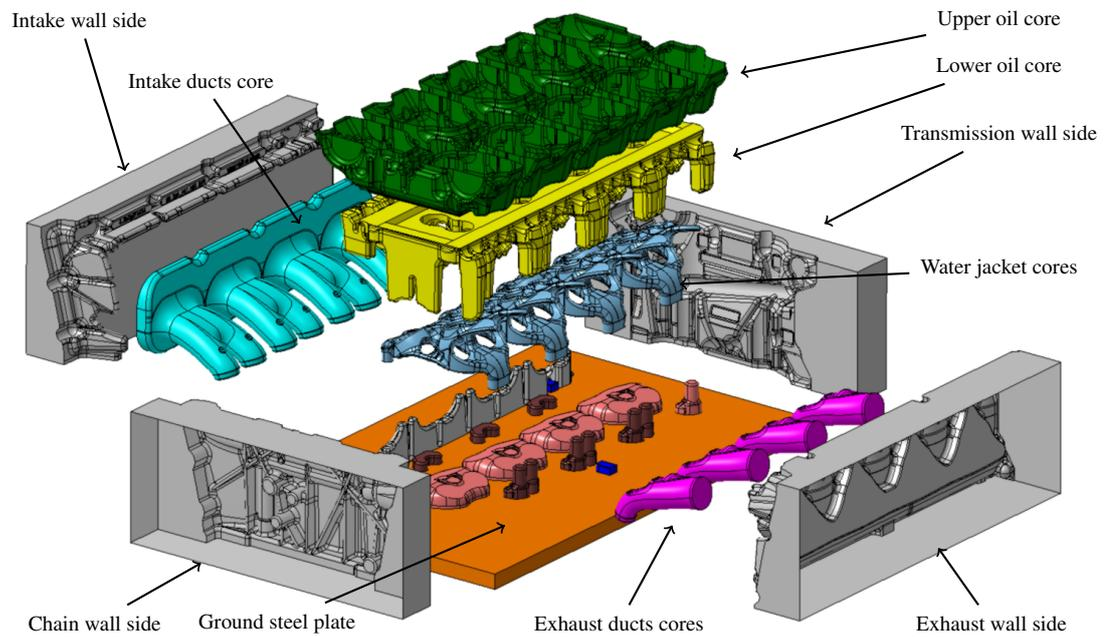
**Figure 1.15:** Exploded view of the cylinder head casting cores and components of the cylinder head protagonist of this thesis work
