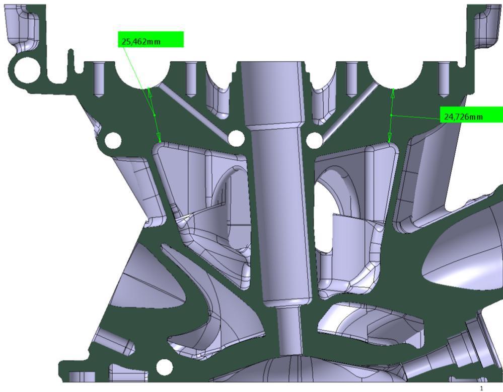
**Figure 2.24:** *Competitor G camshaft bridge section view*
