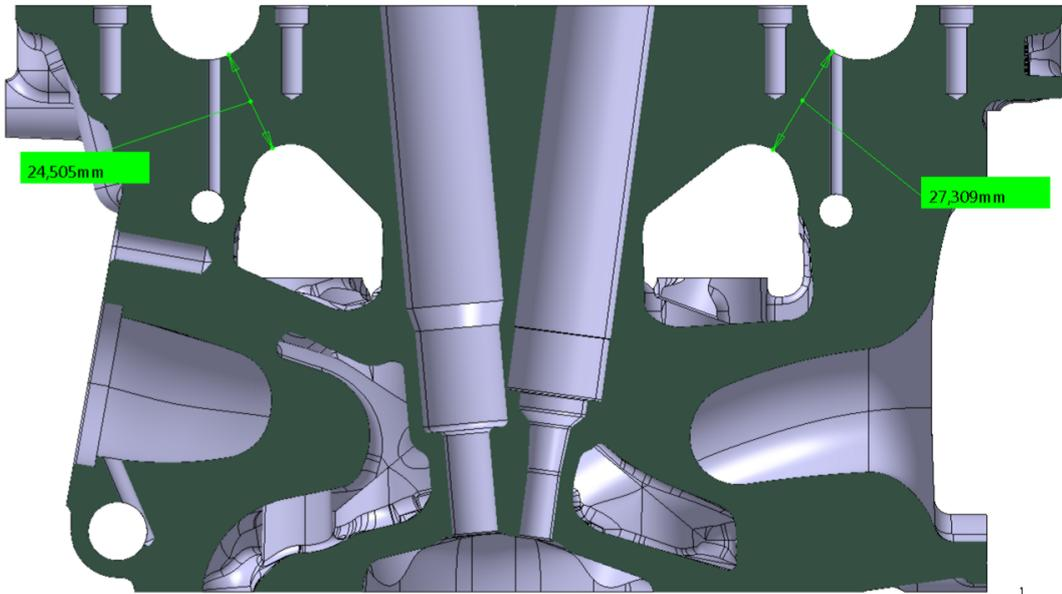
**Figure 2.3:** Reference camshaft bridge section view
