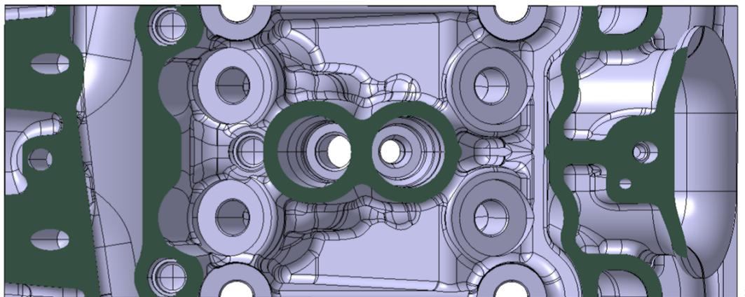
**Figure 2.26:** *Competitor H ribs layout*
