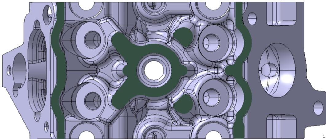
**Figure 2.38:** *Competitor L ribs layout*
