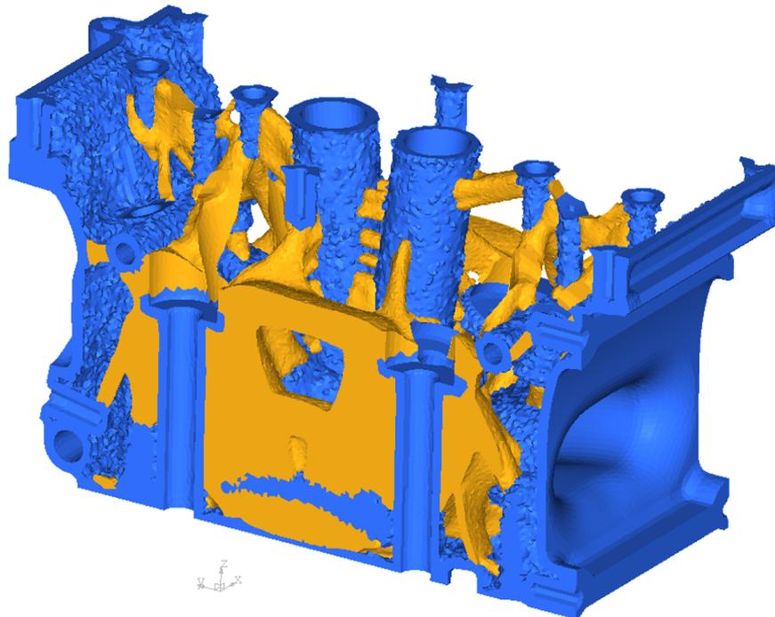
**Figure 3.7:** *Optimal shape result, with 0.35 density threshold view*
