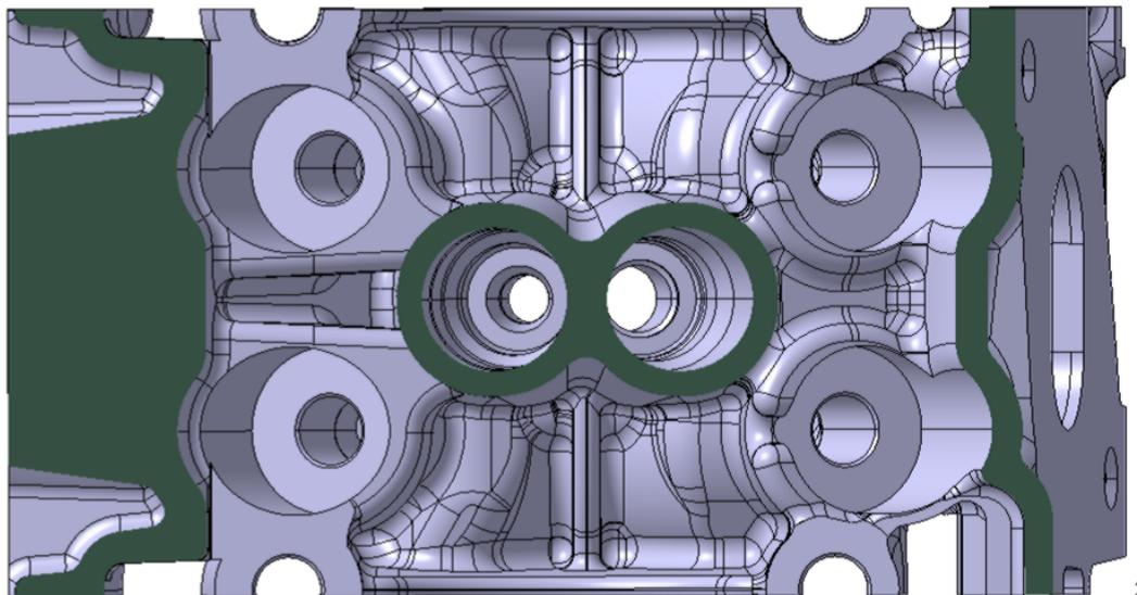
**Figure 2.29:** Competitor I ribs layout
