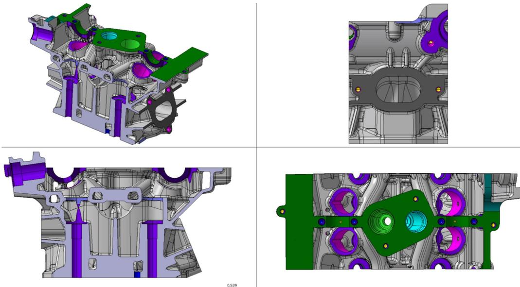
**Figure 2.4:** *Competitor A cylinder head*
