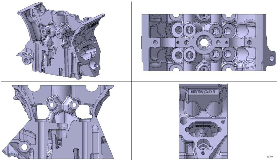
**Figure 2.37:** *Competitor L cylinder head*
