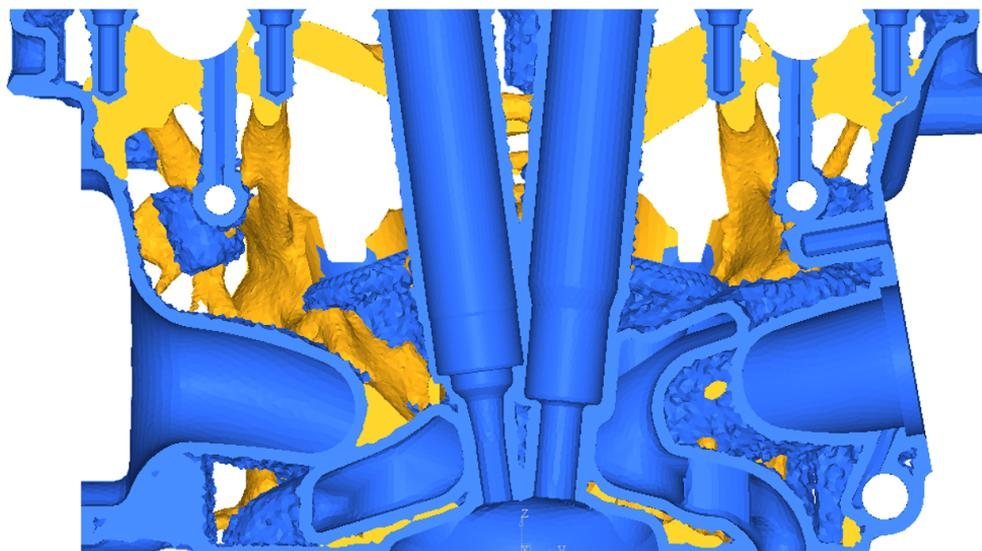
**Figure 3.8:** *Optimal shape result, with 0.35 density threshold view. YZ mid plane section view*
