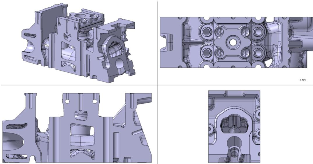
**Figure 2.34:** *Competitor K cylinder head*
