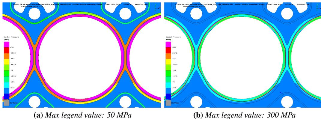
**Figure 3.4:** Gasket pressure analysis of the reference cylinder head
