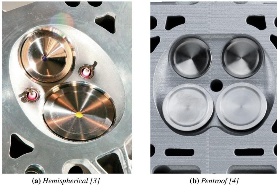
**Figure 1.1:** Different typologies of combustion chambers
