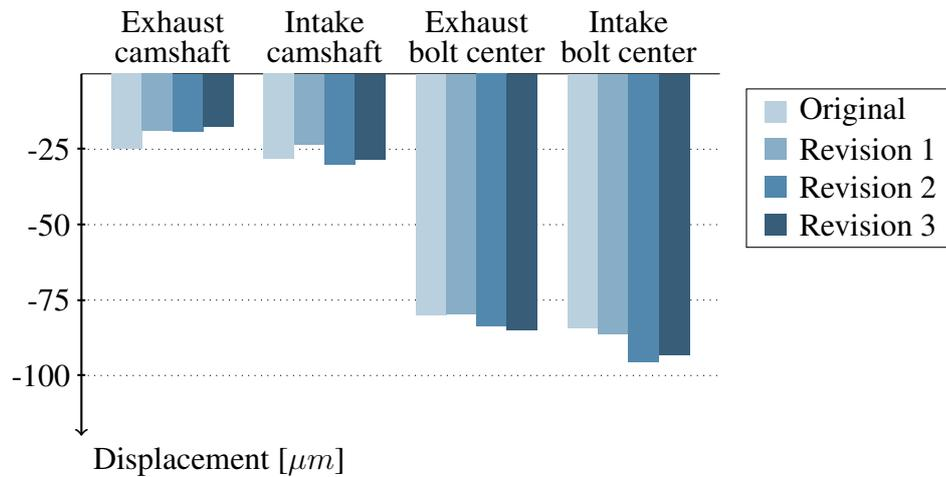
**Figure 4.9:** Cold analysis displacement results
