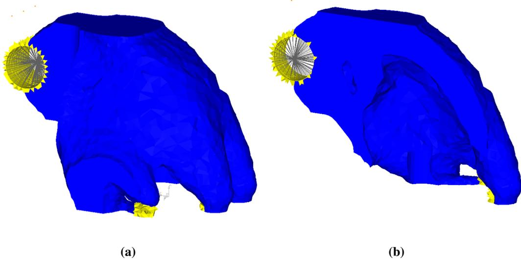
**Figure A.3:** *Hypermesh results for stiffness optimization*
