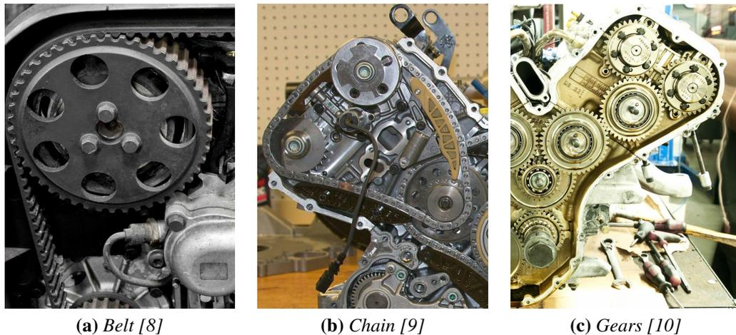
**Figure 1.5:** *Different types of distribution systems*
