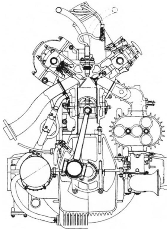
**Figure 1.4:** Alfa Romeo 8C 2900 B engine, with inclined overhead valves and hemispherical combustion chamber [7]
