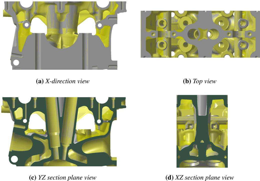
**Figure 4.2:** Revision 02, with the reference component overlay in transparent yellow
