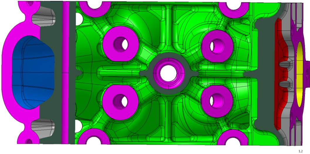
**Figure 2.14:** *Competitor D ribs layout*
