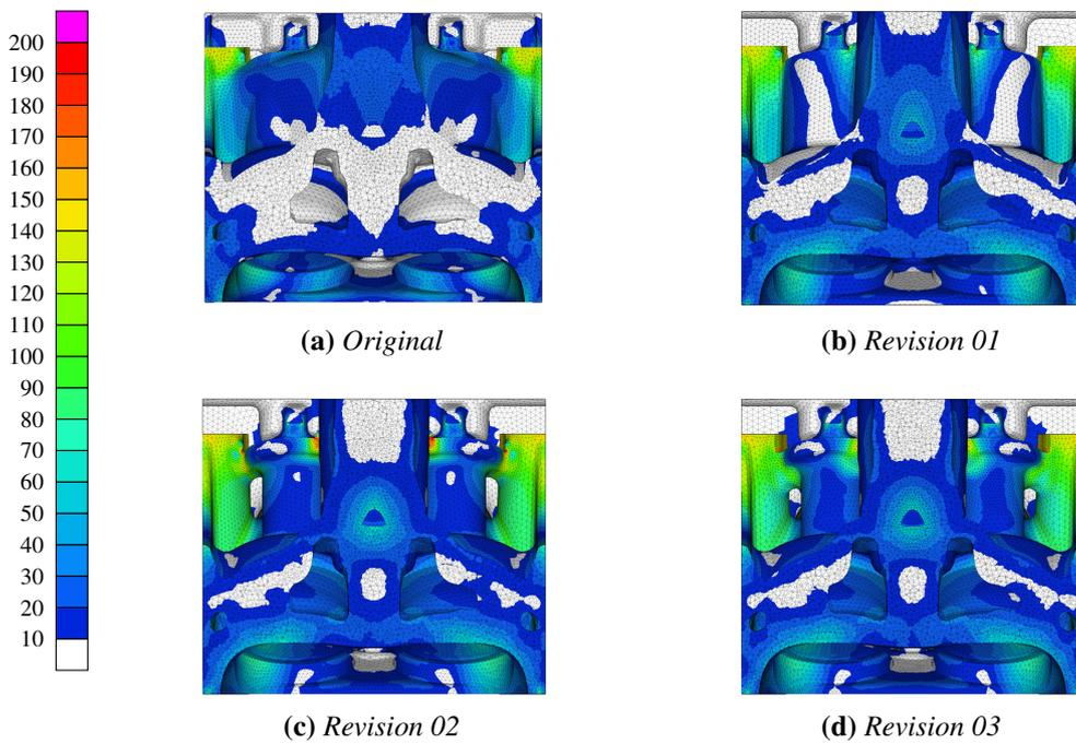
**Figure 4.8:** Cold analysis results, *xz* midplane section view
