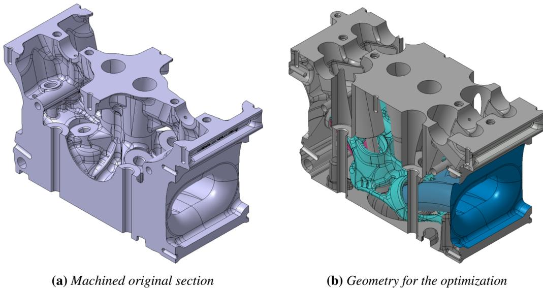
**Figure 3.3:** View of the sections of the reference cylinder head
