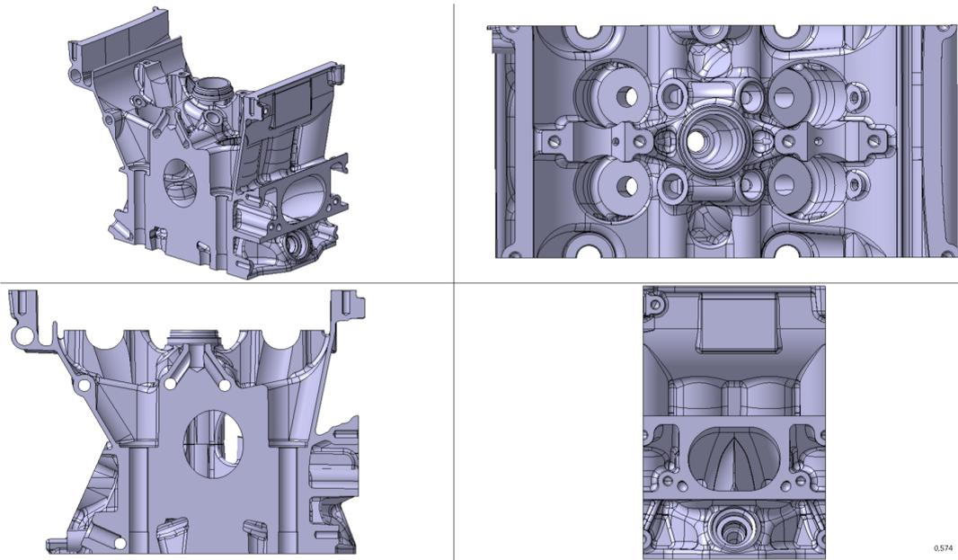
**Figure 2.22:** *Competitor G cylinder head*
