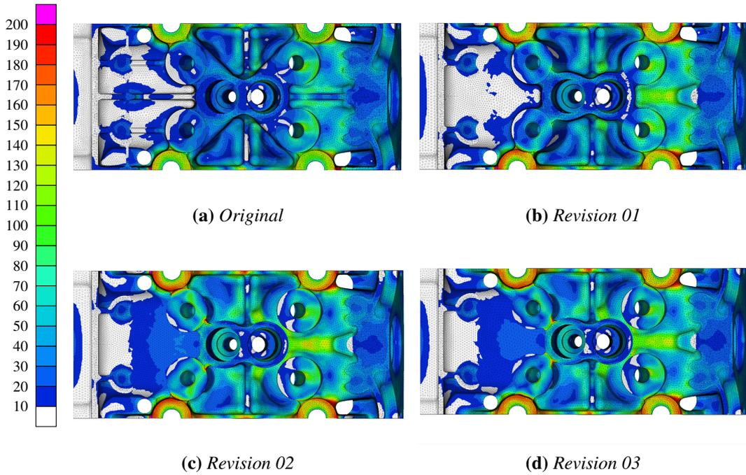
**Figure 4.12:** Hot analysis results, *xy* plane section view
