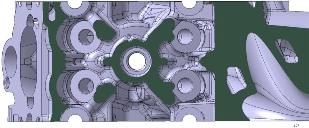
**Figure 2.20:** *Competitor F ribs layout*
