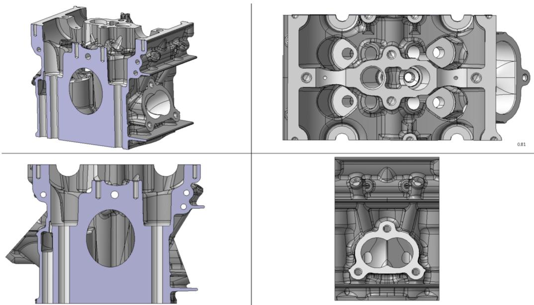
Figure 2.31: Competitor J cylinder head
