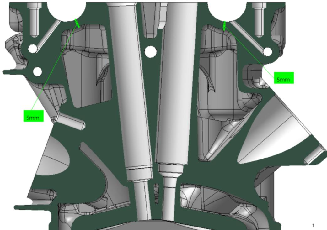
**Figure 2.33:** *Competitor J camshaft bridge section view*
