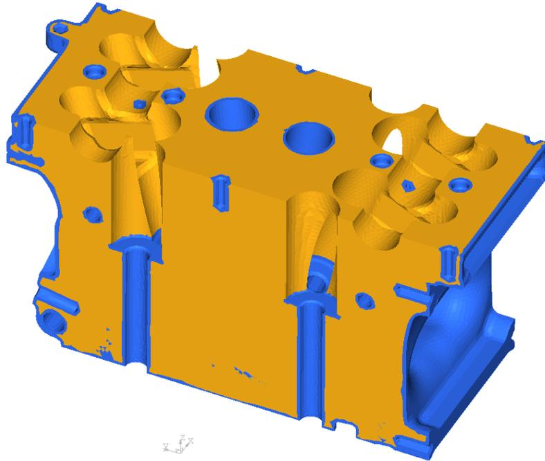
**Figure 3.5:** Model after the meshing process and the design space definition (in yellow). One single layer of non-design elements
