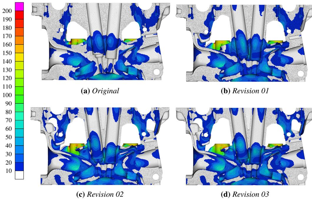
**Figure 4.6:** Cold analysis results, yz midplane section view
