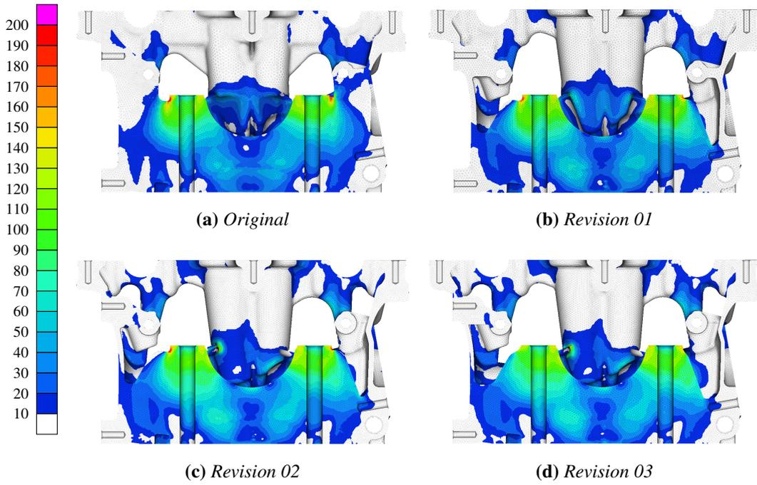
**Figure 4.5:** Cold analysis results, bolt interface plane view
