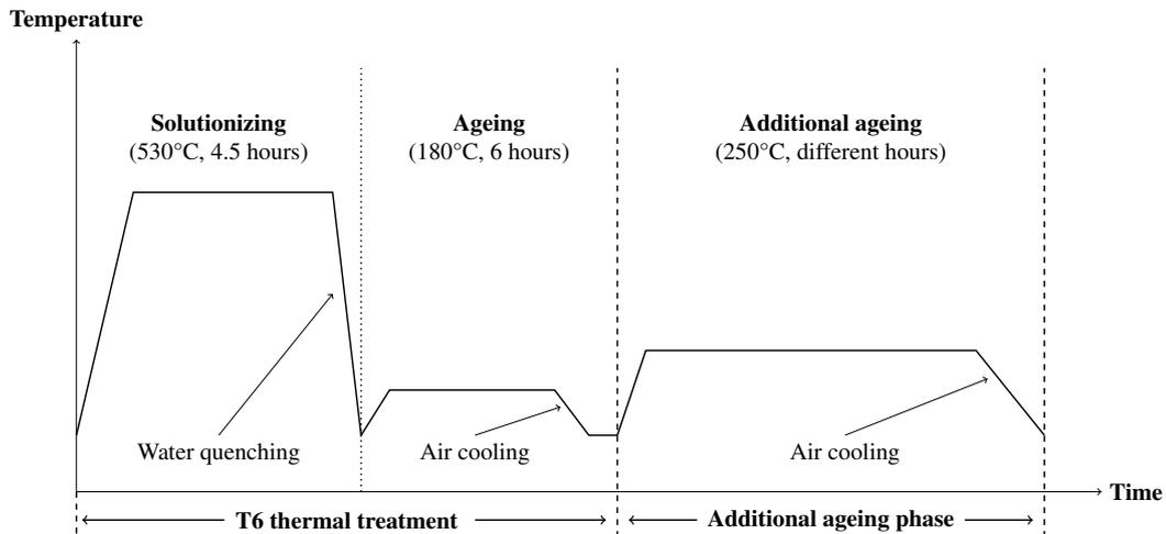
**Figure 1.11:** Time evolution of a T6 thermal treatment plus an additional ageing phase. The additional ageing time depends on the final desired material properties [20]
