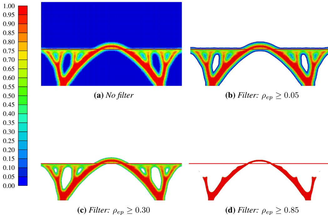
**Figure 3.2:** Topological optimization example of a bridge; element density result. Objective: maximization of the stiffness - Constraint: final mass 15% of the initial one
