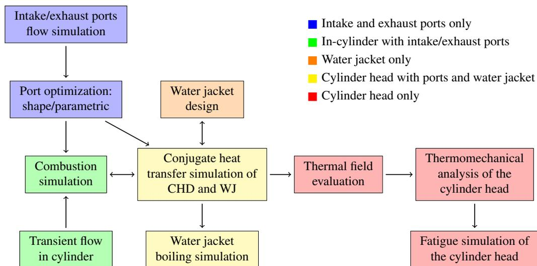
**Figure 4.4:** Example of workflow for the thermal analysis of a cylinder head [30]
