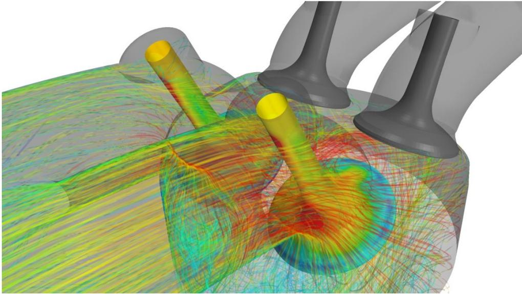
**Figure 1.9:** CFD analysis with streamlines view of intake ports [15]
