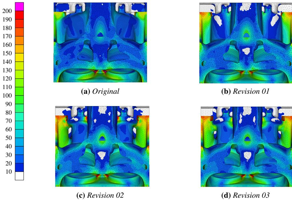
**Figure 4.13:** Hot analysis results, *xz* midplane section view
