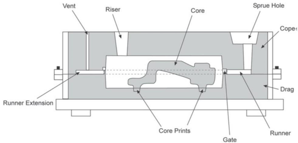
**Figure 1.14:** Schematic of the mold for sand casting and its parts [25]
