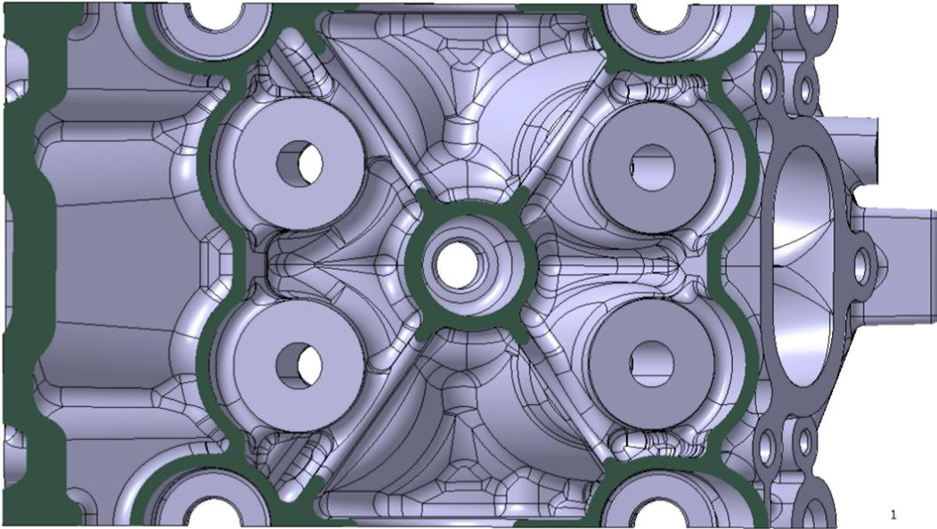
**Figure 2.23:** *Competitor G ribs layout*
