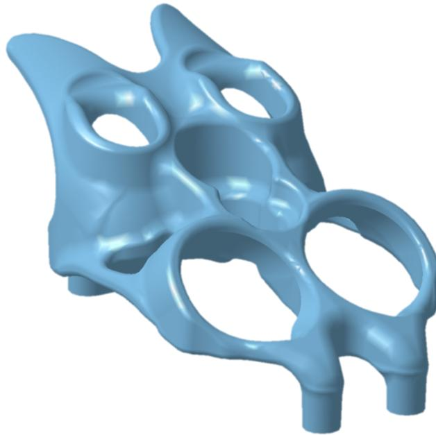
**Figure 1.2:** CAD drawing of a cylinder head water jacket, seen from the intake ports
