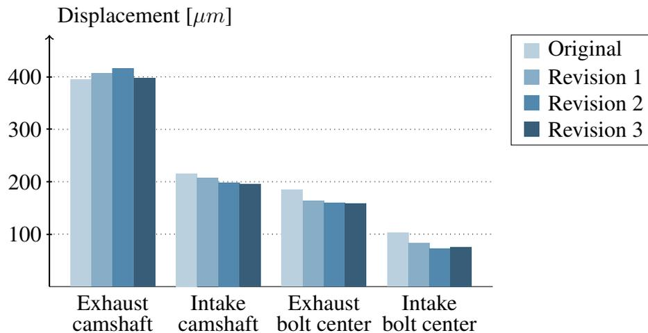
**Figure 4.14:** Hot analysis displacement results
