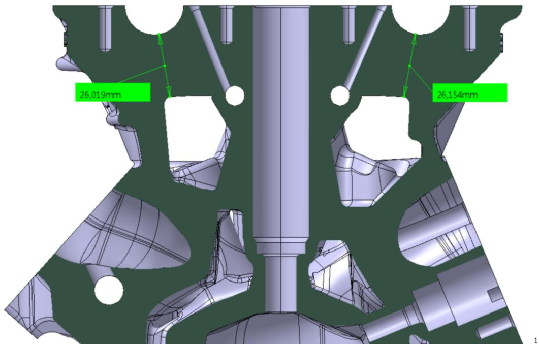
**Figure 2.39:** *Competitor L camshaft bridge section view*
