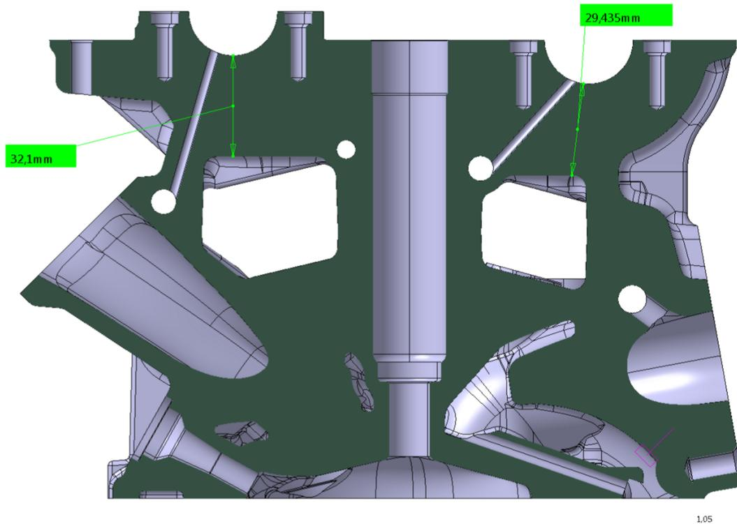
**Figure 2.12:** *Competitor C camshaft bridge section view*
