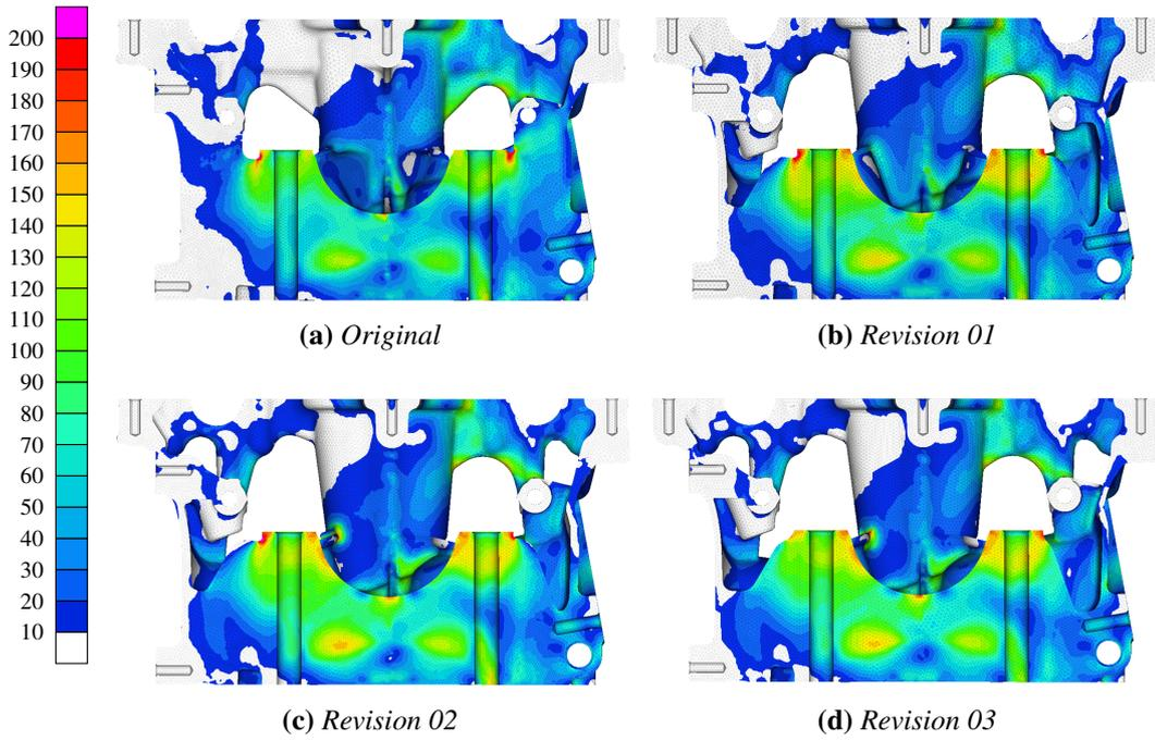
**Figure 4.10:** Hot analysis results, bolt interface plane view
