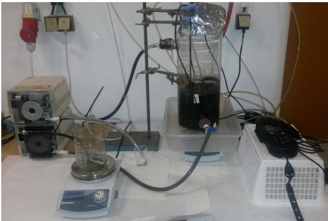
Figure 3.2 - Sequencing Batch Reactor used for the experiments
