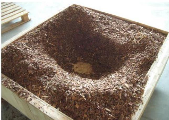
*Figura 17: Provino di materiale (Fonte: Kain et al., Bark as Heat Insulation Material. University of Applied Sciences Salzburg. 2013.)*
