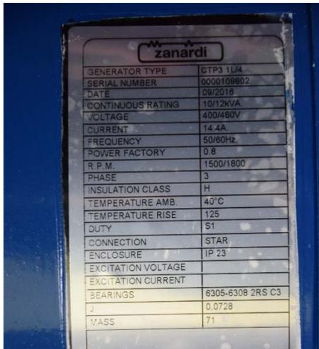
A technical data plate for a Zanardi generator, mounted on a blue metal surface. The plate is titled 'zanardi' and lists various specifications in two columns.
