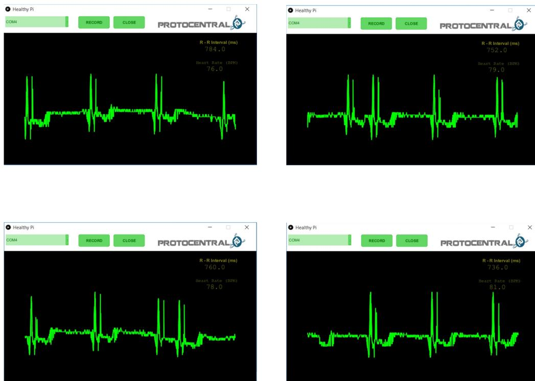
Figure 5.2: First results with bluetooth mode and wet-contact electrodes.
