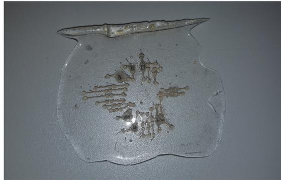
Figure 4.24: Final test circuit with resistors on zPDMS.
