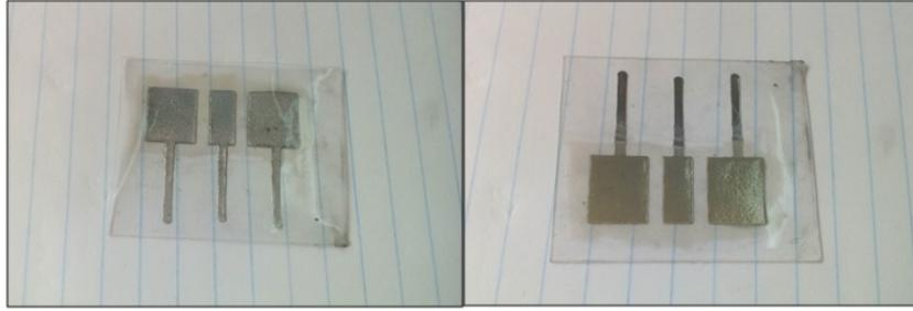
Figure 2.9: Top view (left) and bottom view (right) of the final zPDMS electrodes [21].
