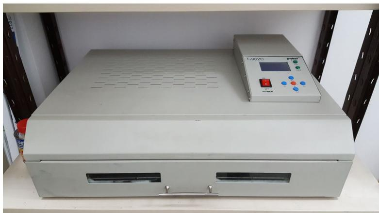
Figure 3.8: T962C Reflow oven
