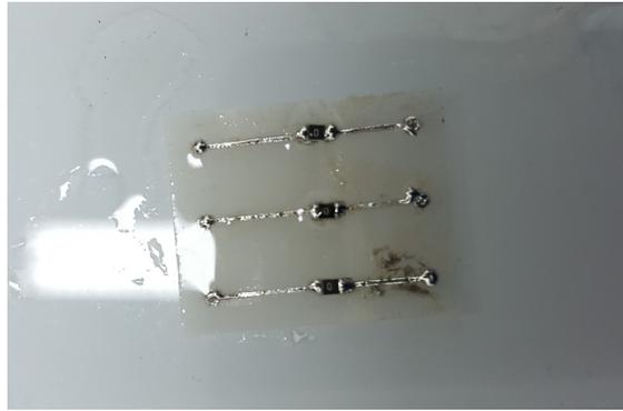
Figure 3.5: Conductivity test with liquid metal on the resistors path
