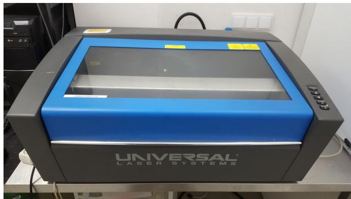
Figure 3.6: Laser cutter
