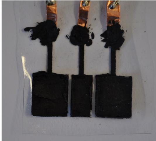
Figure 2.11: Top view of the final cPDMS electrodes [21].
