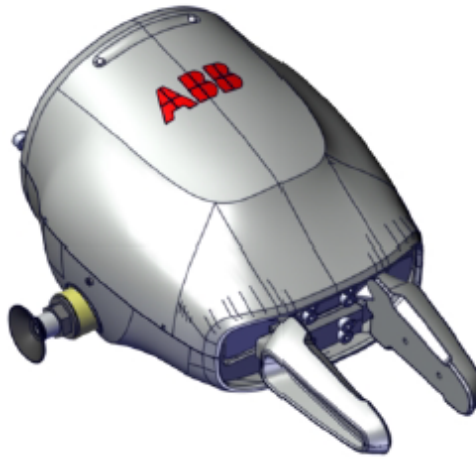
Figure 7.2: YuMi ABB gripper with suction and servo-assisted modules
