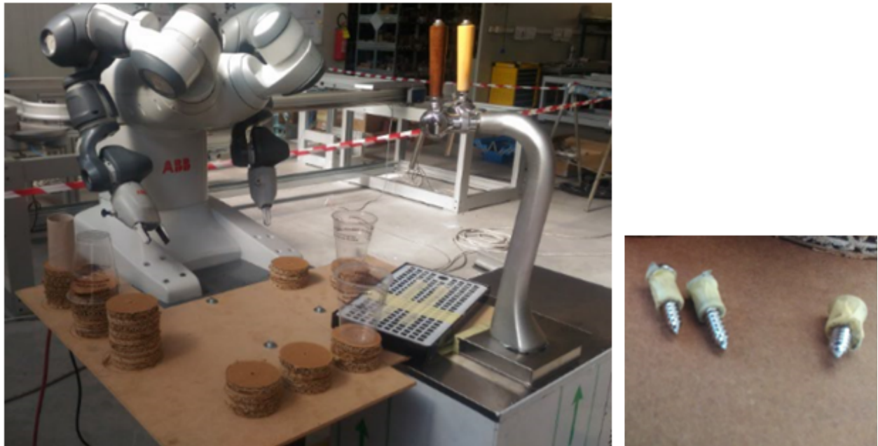
Figure 10.1: A first phase of real prototype system building and the elements used to maintain the plastic cup fixed before the withdrawal
