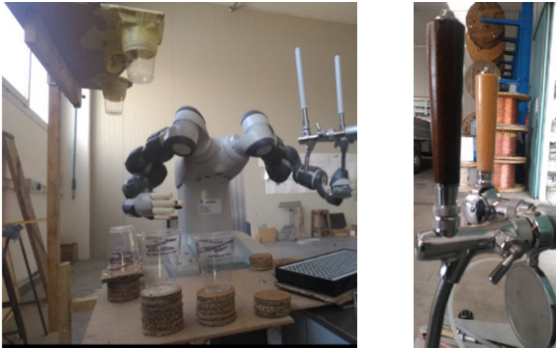
Figure 10.2: The final real prototype system, with the final delivery position at growing high from left to right (from the YuMi point of view) and the new knob to give a bigger lever; on the right, a comparison between the two taps used in the different development phases
