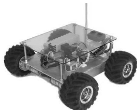
**Figure 1.1 a** -Example of wheeled robot
