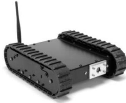
**Figure 1.1 b** -Example of robot fitted with Caterpillar tracks
