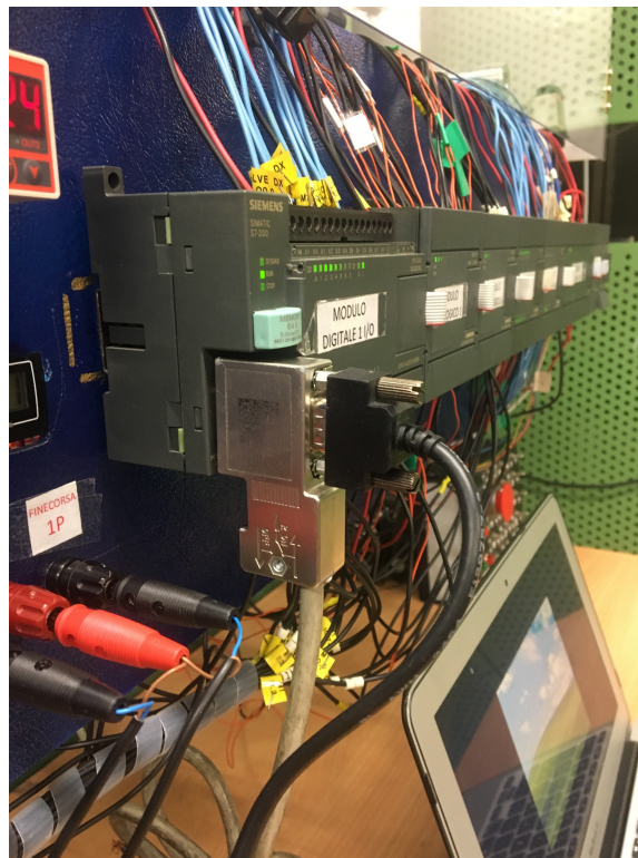
Figure 71: Connection with computer and TD 200 pad due to the NETlink Profibus cable.
