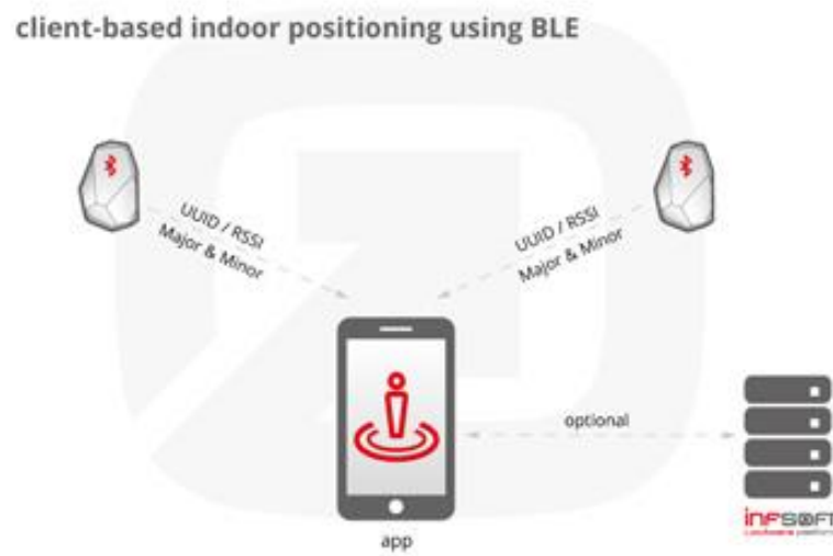
Figure 12: Client-based indoor position using BLE [32]
