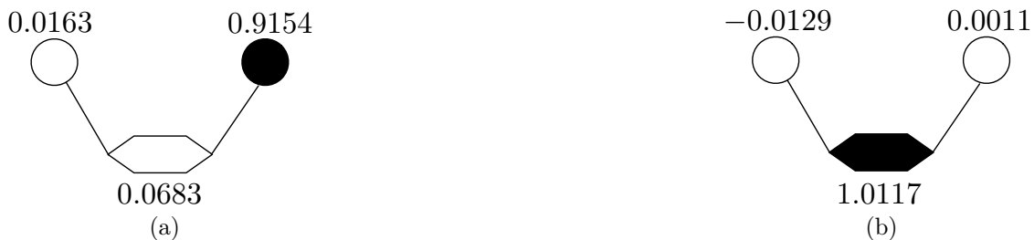
Figure 6.19: Bis-ferrocene oxidized scheme: at the equilibrium (a), with a clock field of 10 V/nm (b).
