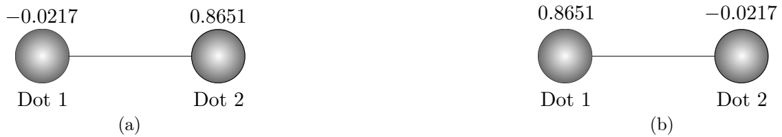
Figure 3.5: Displacement of the charge with an external electric field of: (a) -5 \text{ V/nm} ; (b) 5 \text{ V/nm} .
