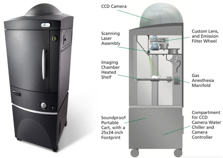
Figure 3.10: Picture of IVIS and schematic of its more important components.
