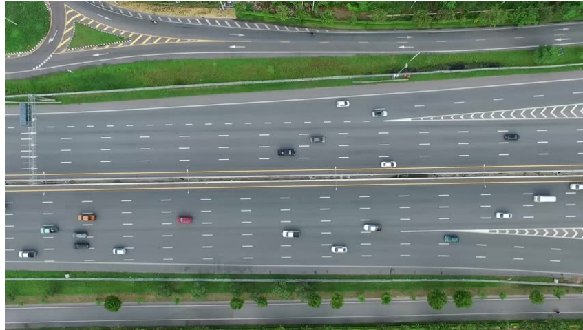
Figure 3.6: Slip road with multiple lanes and close separated roads [32]
