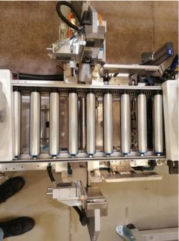
The first tests demonstrated that some inaccuracies in the process were still present as the final orientation was not perfectly oriented. Another solution proved functional and reliable, giving no further issues during the project: the clamping device has been substitute with two independently actuated jaws, controlled by the analog reading of an analog sensor that verifies the exact position at which the jaws have to be at the end of the operation.
