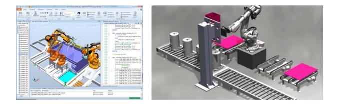
RobotStudio is a tool that can be useful at every stage of a project. It allows to pick the robotic arm that best suit the requirements of the project, and allows to recreate the environment in which it is going to be deployed. The modeling and simulation tools it contains, allow to create a realistic 3D version of the layout even at early stages: furing step 2 the layout is still not completely defined, but it is however possible to verify the actual
