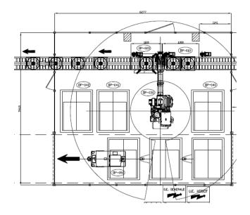
The third supplier is again from the Marche region and, again has some past experience of working with the plant for previous installations. The proposed concept involves the use of a pantograph automation, placed above the conveyor and across it laterally, that is able to move above it to pick up the carton, open it and insert it on the product.
