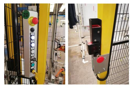
Additional emergency stop "mushroom" buttons are located outside of each door, on the main panel, and inside the barriers so that in any case in which a person is at a risk of being harmed the automation can be instantaneously halted and blocked completely.
