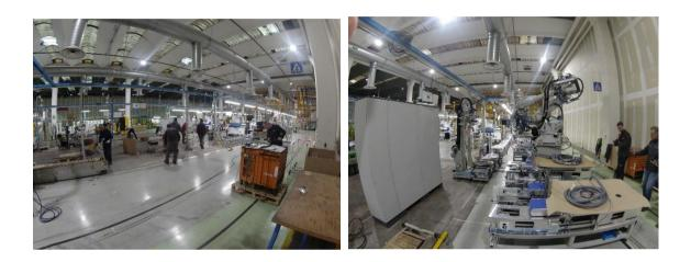
The next step consisted in the electrical wiring of all the components to the robot controller and to the PLC. Similarly, tubing for compressed air and vacuum were predisposed.
