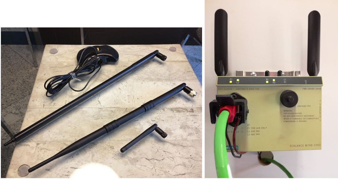
(a) From top to bottom: 9-7-5 dBi omnidirectional antennas. (b) Scalance W 788-2 PRO with directional 3 dBi antennas (in lab n. 201).
