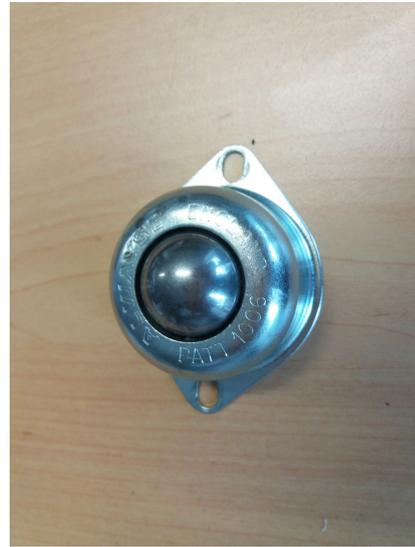
Figure 1.5: The ball bearing omni-directional wheels used to enable the rospo to move
