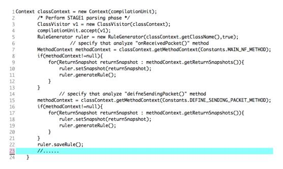
Figure 5.7. Code for generating rules from each return snapshot
