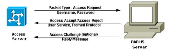
Figure 6.2. Traffic Flow in Radius Authentication Process.
