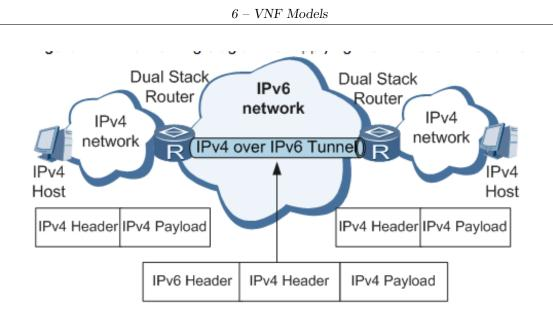
Figure 6.14. Networking diagram for applying the IPv4 over IPv6 tunnel)
