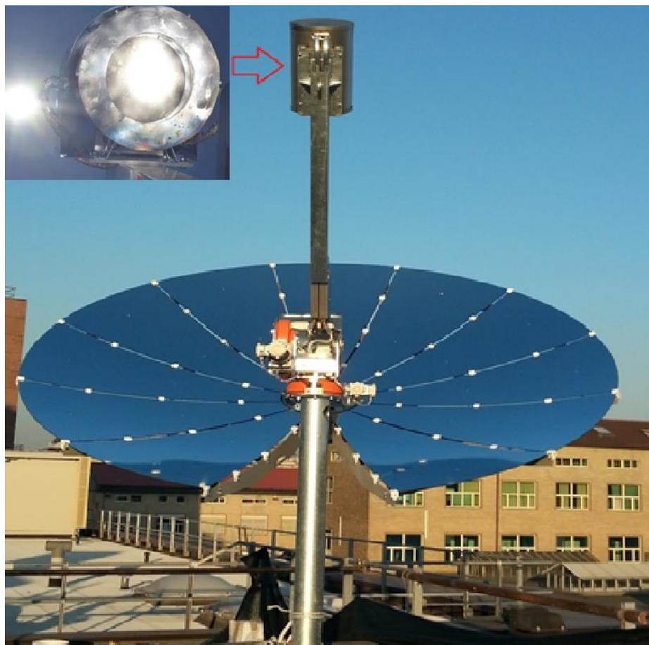
Figure 3.6: External view of both installed collector and receiver.
