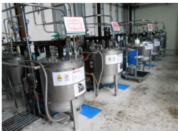
Figure 20 - Photo of buffer tanks, mixers and tanks for paint preparation
