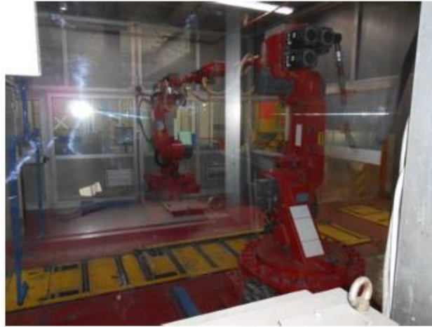
Figure 17 - Photo of the flame cabin and robots
