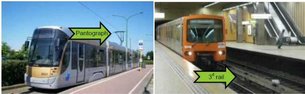
Figure 18 Different power supply systems for urban rail vehicles. Source: [7]
