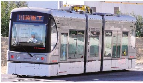
Figure 24 SWIMO by Kawasaki Heavy Industry Ltd (left) and ALSTOM Citadis (right) in catenary-free operation in Nice (France) and Sapporo respectively. Source:[7, 25]
