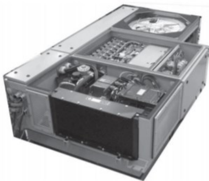
Figure 41 Roof-mounted flywheel on the Citadis operating in Rotterdam. Source: [44]
