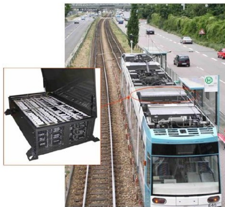
Figure 38 Roof-mounted MITRAC Energy Saver on LRV in Mannheim. Source:[76]
