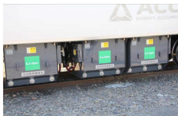
Figure 35 On-board battery pack for the Series EV-E301. Source: [66]
