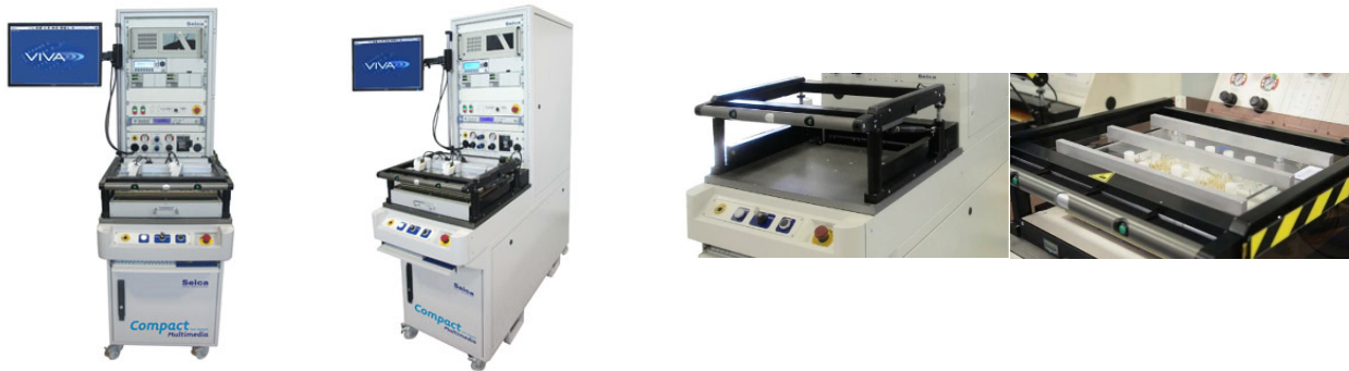
FIGURE 46- COMPACT SERIES OF PRODUCTS WHICH ARE USING FIXTURES AND CANNOT OPERATE WITHOUT FIXTURES THE RIGHT-SIDE PICTURE ILLUSTRATES A COMPACT WITH FIXTURE LOADED INSIDE
