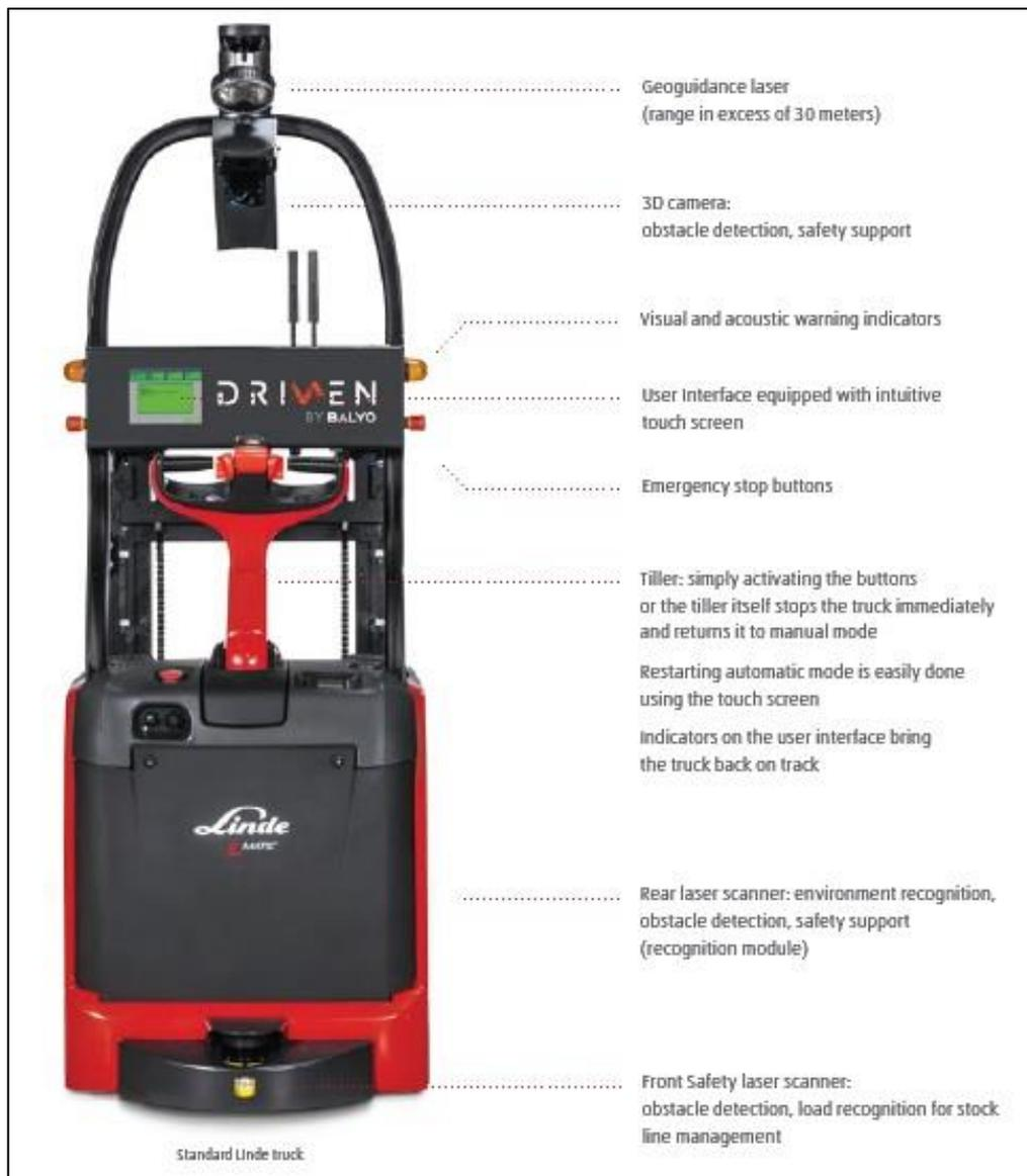
Figura 3.8 : AGV L-MATIC (LINDE, 2017)
