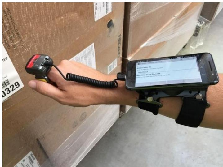
**Figura 3.6 Ring barcode scanner**
