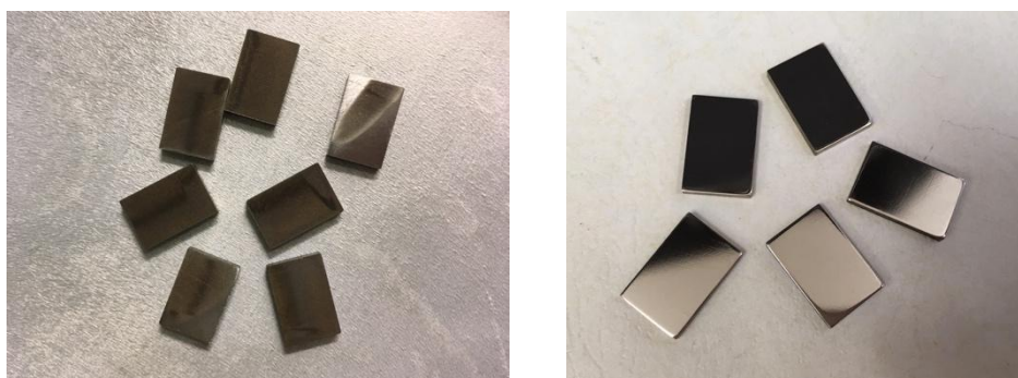
Figure 4.4: dirty samples as received vs mirror polished samples
