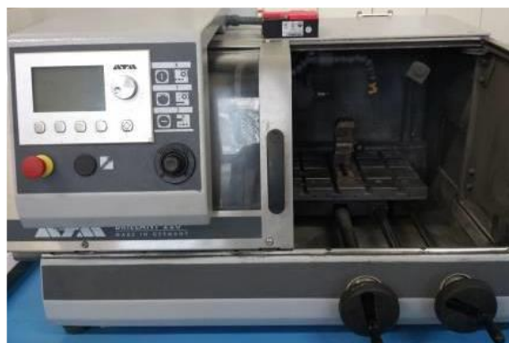
Figure 43. Cutting Machine for cutting samples in disks with 2mm thickness
