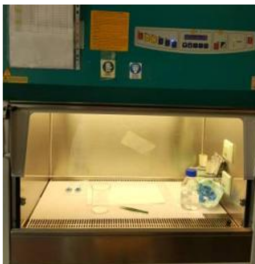
Figure 57. Laminar flow hood and jars containing the samples immersed in the corresponding \text{AgNO}_3 solution
