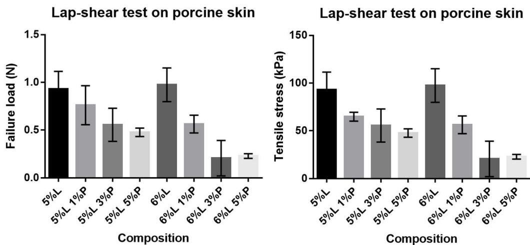
FIGURE 2.38: Failure load and tensile stress vs composition using porcine skin. Bar chart representing the changes in adhesiveness versus the composition. Increasing the amount PEO is not convenient in term of adhesion: the failure load and the tensile strength are lower.
