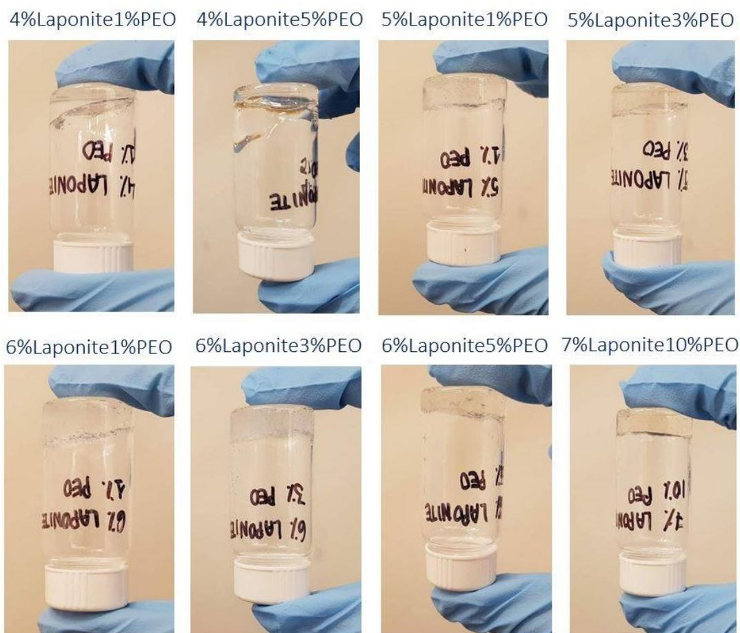
FIGURE 2.2: Tube inversion test applied to determine if gelation occurred so to identify the lower limit of Laponite/PEO nanocomposites. After 30 min from the material synthesis, the 4% Laponite with 0%, 5% and 10% of polymer is not a gel whereas all the other materials were gels.
