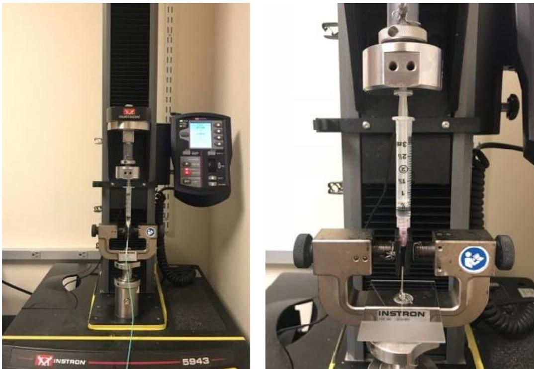
FIGURE 2.3: *Experimental setup for injection force measurements. In the left picture, a 4F catheter is used, in the right one, a 18G needle is used. The mechanical tester, its accessories and the catheter positioning are visible.*
