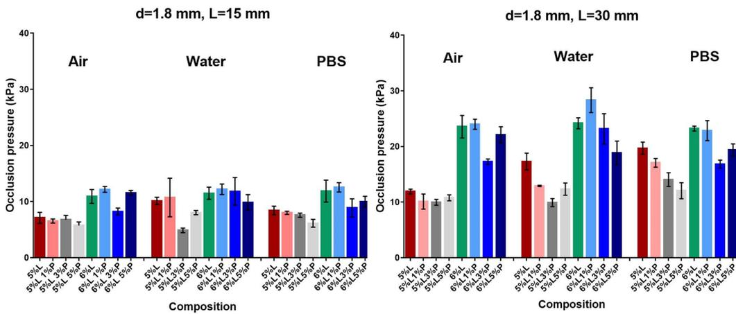
FIGURE 2.8: Occlusion pressure measurements in 1.8 mm tube, putting 15 mm (left figure) and 30 mm (right figure) of material inside the tube. Air, water and PBS were spilled against the blockage.
