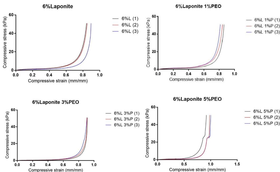
FIGURE 2.34: Stress versus strain curves of Laponite/PEO gels use to calculate Young's Modulus, fitting the linear region of the stress-strain curve between 0% and the 10% of the maximum strain measured, and calculating the ratio.
