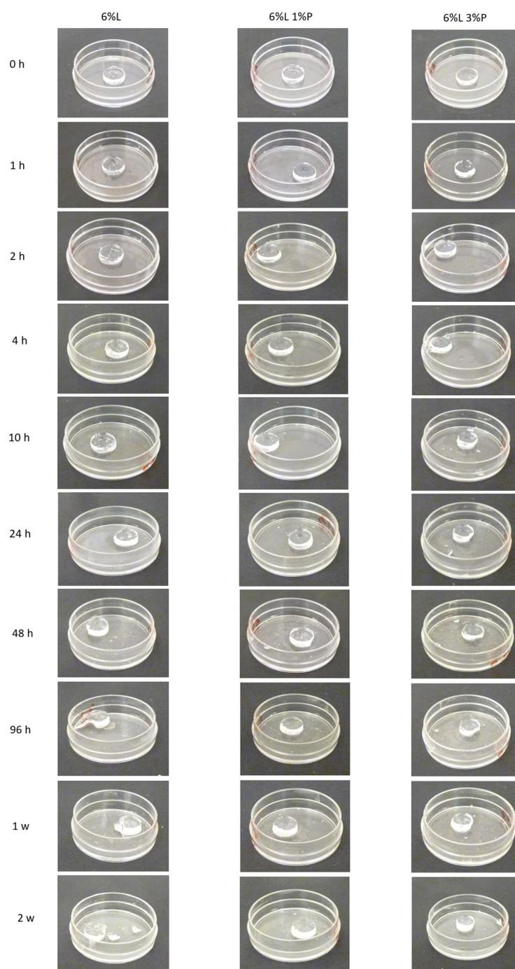
FIGURE 2.21: *Stability in HTF. Changes in weight were observed at the showed timepoints (obviously once the medium is removed) and at each time-point pictures were taken. Four samples for each composition were prepared and between them the most representative was chosen to be plotted. The more stable material in HTF seems to be 6% Laponite 1% PEO.*
