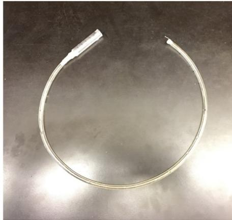
FIGURE 2.17: – *Homemade connector created taking off the plunger from a 10 mL syringe and cutting the part closer to it, reducing the length of the syringe of 1 cm. This was then connected to a soft and flexible Tygon tube.*
