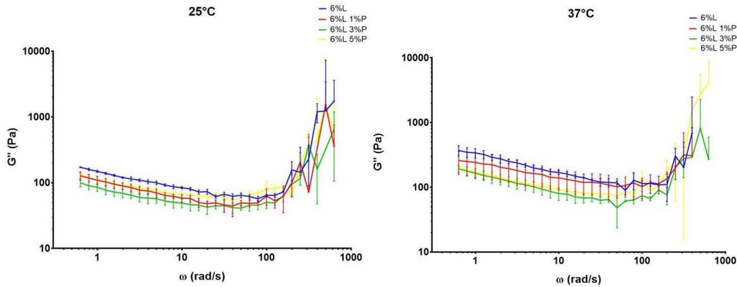
FIGURE 2.45: Loss modulus vs angular frequency at 25°C and 37°C. Oscillatory frequency sweep was conducted at 0.1-100 Hz and 10 Pa. The curves are plotted on log-log plot. Gel moduli were not so dependent on oscillatory deformation frequency and were a bit more elastic at high shear rates but also more viscous at low shear rates.
