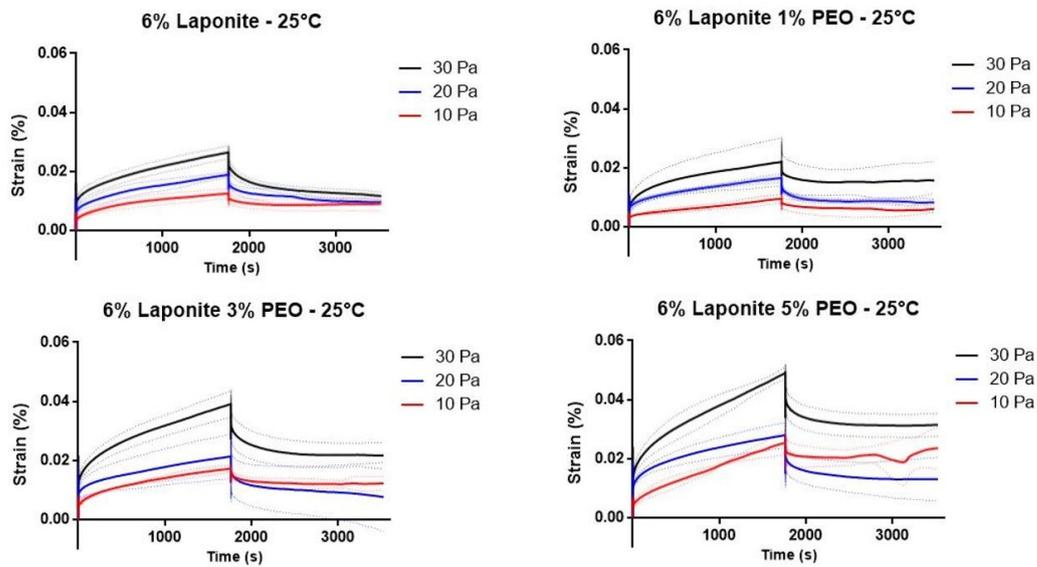
FIGURE 2.46: Rheological creep and recovery test: strain vs time. Four gels were tested at 25°C and three different loads were applied: 10 Pa, 20 Pa, 30 Pa.
