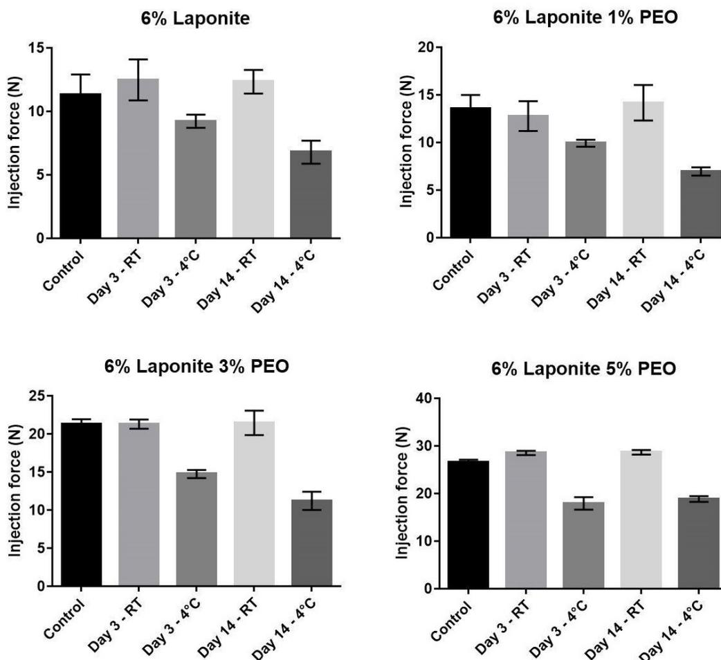
FIGURE 2.40: Aging effect on shear-thinning biomaterials. The evaluated compositions are, from the top left to the bottom right, with a percentage of laponite of 6% and increasing PEO. The temperatures of storage are 25°C (room temperature, RT) and 4°C, the observed timepoints are 3 days and 14 days. The materials look very stable at RT, even when they are stored for 14 days. However, their injectability decreases drastically when they stay inside the fridge.
