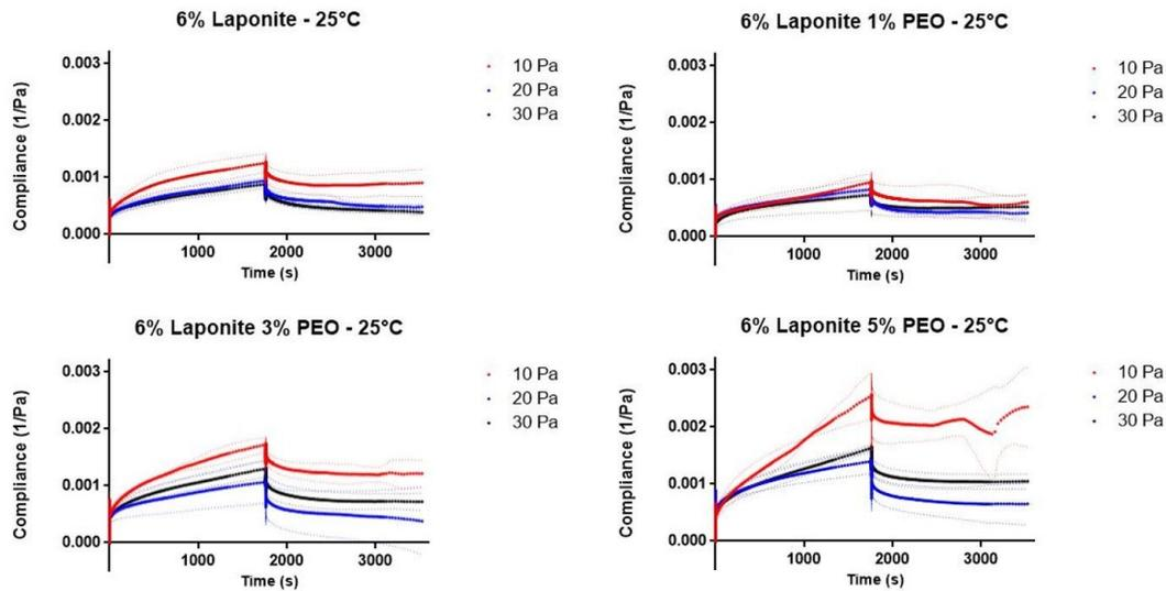
FIGURE 2.47: Rheological creep and recovery test: compliance vs time. Four gels were tested at 25°C and three different loads were applied: 10 Pa, 20 Pa, 30 Pa.
