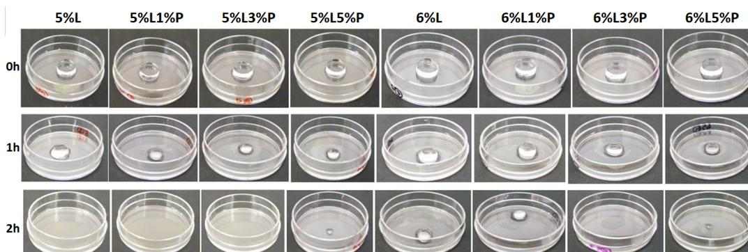
FIGURE 2.30: *Reversibility test. Changes in weight were observed at the showed timepoints (obviously once the medium is removed) and at each time-point pictures were taken. Four samples for each composition were prepared and between them the most representative was chosen to be plotted. There is a visible trend: the higher the PEO concentration, the more reversible is the gel formation over time. Moreover, materials with less Laponite dissolve faster and heavier.*
