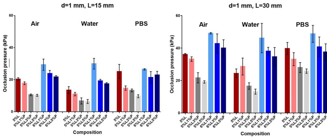
FIGURE 2.7: Occlusion pressure measurements in 1 mm tube, putting 15 mm (left figure) and 30 mm (right figure) of material inside the tube. Air, water and PBS were spilled against the blockage.
