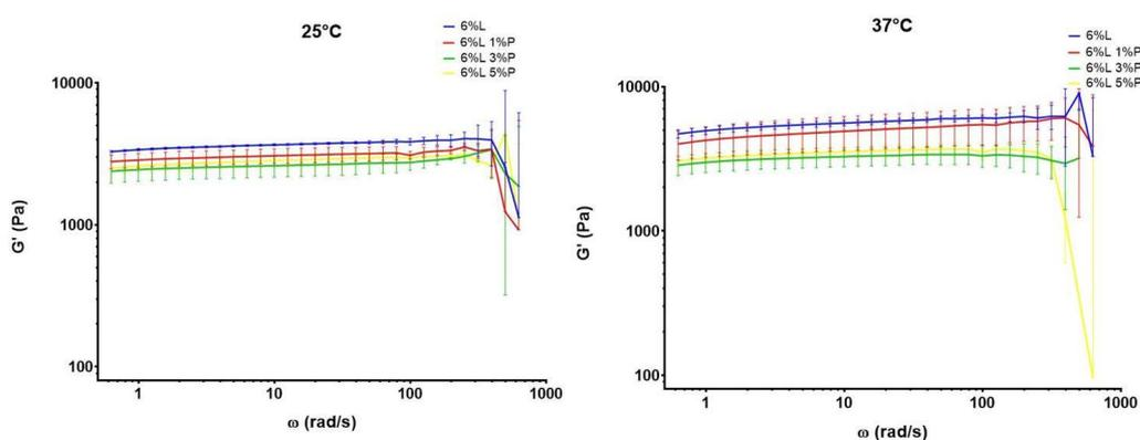
FIGURE 2.44: Storage modulus vs angular frequency at 25°C and 37°C. Oscillatory frequency sweep was conducted at 0.1-100 Hz and 10 Pa. The curves are plotted on log-log plot. Gel moduli were not so dependent on oscillatory deformation frequency and were a bit more elastic at high shear rates but also more viscous at low shear rates.
