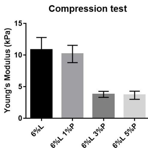
FIGURE 2.35: Young's compressive Modulus ( $E$ ) vs composition. It is clear that materials with less PEO have a higher  $E$  so higher mechanical properties.
