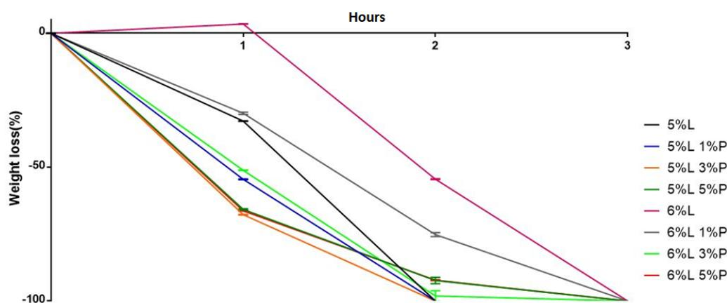
FIGURE 2.31: *Weight loss (%) vs time. The graphs are about changes in weight over time. Results match the pictures. After 3 h, all the samples were completely dissolved in water, starting from those with lower content of Laponite which after 2 h were around -100% of the initial weight.*
