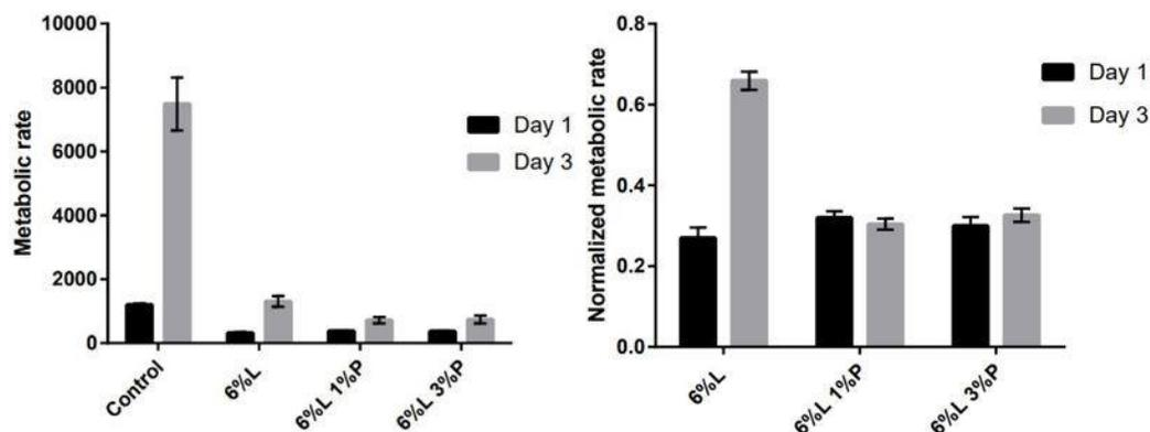
FIGURE 2.57: *Metabolic rate versus composition and normalized rate (normalized with the control) versus composition. The PrestoBlue analysis showed that cells on 6% Laponite are alive and have a higher metabolic rate than on the other 2 gels.*
