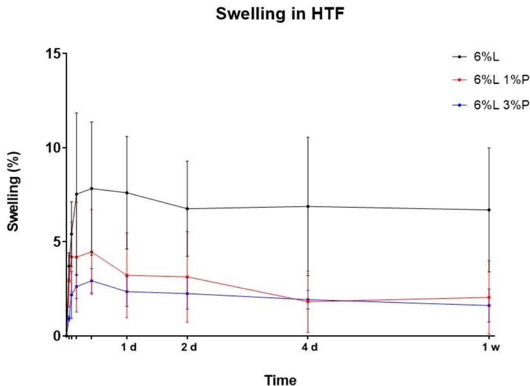
FIGURE 2.25: Swelling of reduced set of gels in HTF until 1 week. This experiment was done with Eppendorf tubes, putting three materials (6% Laponite, 6% Laponite 1% PEO and 6% Laponite 3% PEO) in contact with HTF for 1 week at 37°C. The 6% Laponite is the one that swells better compared to the others but, it is a very small swelling, irrelevant.
