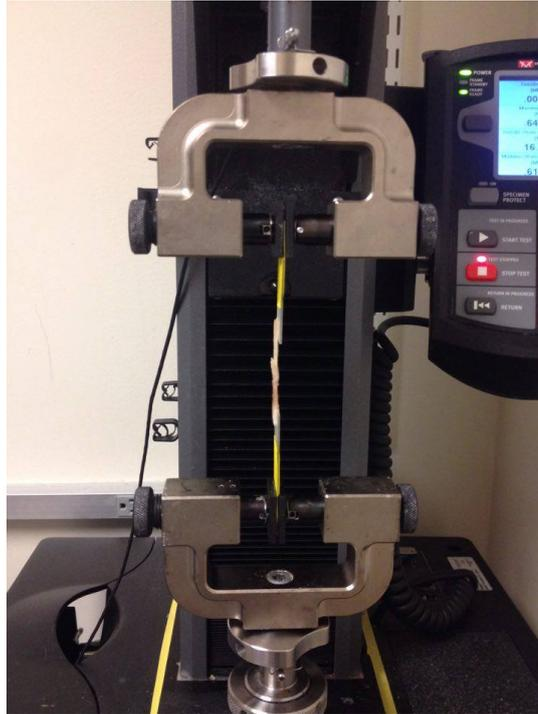
FIGURE 2.37: Experimental setup lap-shear test. The tensile test was performed using the mechanical testing unit INSTRON 5943 that pulled at 20 mm/min one of the samples until failure (the other one is fixed).
