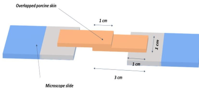
FIGURE 2.36: Preparation of the sample. After cutting the tissue in 3 cm x 1 cm strips, 0.01 ml of material was injected in an area of 1 cm x 1 cm of one of the two strips and they were pressed together, using a clamp for 3 min, to increase the contact force.
