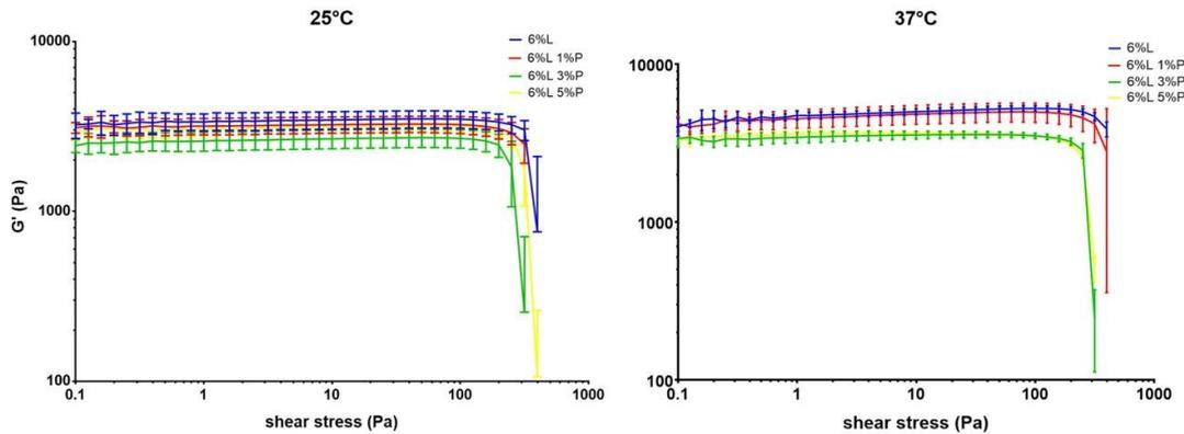
FIGURE 2.42: Storage modulus vs shear stress at 25°C and 37°C. Oscillatory stress sweep was conducted at 0.1-1000 Pa and 1 Hz. The curves are plotted on log-log plot. For all our materials  $G'$  is bigger than  $G''$  so the material behaves in theory like an elastic solid. 6% Laponite 3% PEO and 6% Laponite 5% PEO are softer materials but weaker than the other gels.
