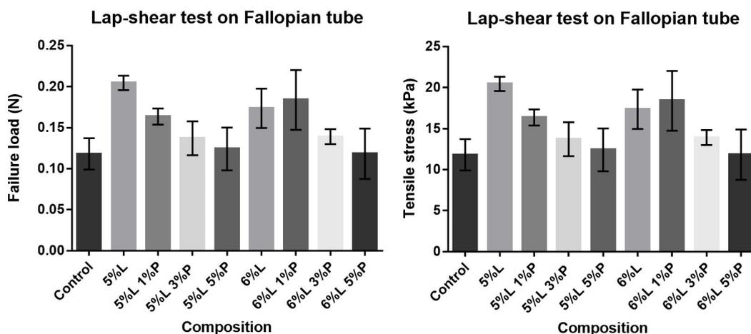
FIGURE 2.39: Failure load and tensile stress vs composition using porcine Fallopian tube. Bar chart representing the changes in adhesiveness versus the composition. In this graph values are lower and the decline due to the change in material is less evident. This might be since the Fallopian tube are generally more wet and "slippery" so the adhesion strength is weak.
