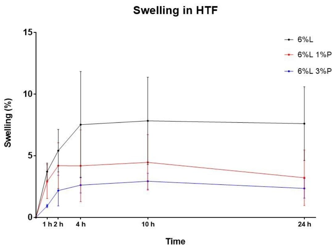
FIGURE 2.24: Swelling of reduced set of gels in HTF until 24 h. This experiment was done with Eppendorf tubes, putting three materials (6% Laponite, 6% Laponite 1% PEO and 6% Laponite 3% PEO) in contact with HTF for 24 hours at 37°C. The 6% Laponite is the one that swells better compared to the others but, it is a very small swelling, irrelevant.
