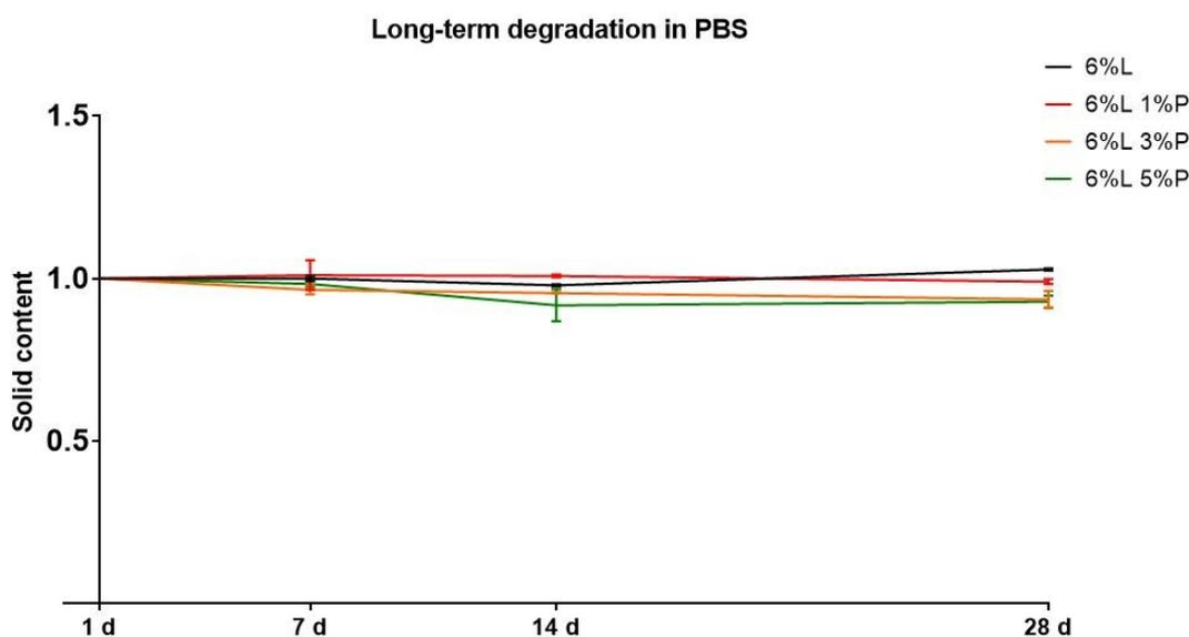
FIGURE 2.29: Degradation of gels with 6% Laponite in PBS until 28 days.
