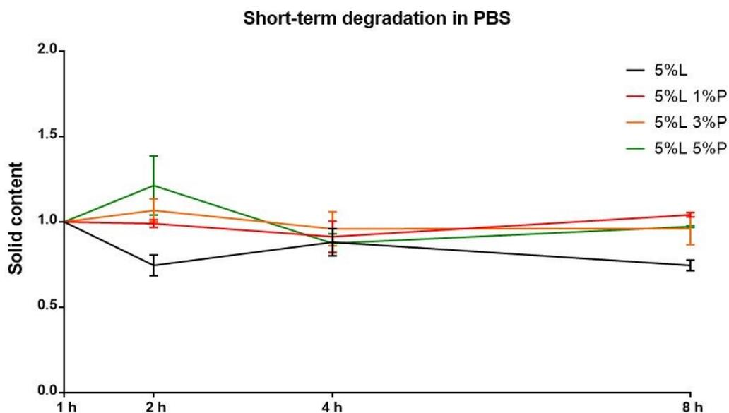
FIGURE 2.26: Degradation of gels with 5% Laponite in PBS until 8 h.
