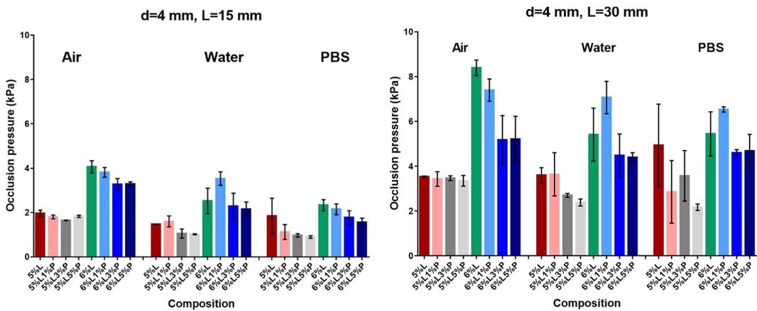
FIGURE 2.10: Occlusion pressure measurements in 4 mm tube, putting 15 mm (left figure) and 30 mm (right figure) of material inside the tube. Air, water and PBS were spilled against the blockage.
