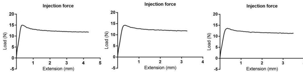
FIGURE 2.4: Example of load versus extension curves obtained from the injection force experiment. The material in study was the 5% Laponite 5% PEO. As it can be seen, all the curves have a peak and reach a plateau around the same values.
