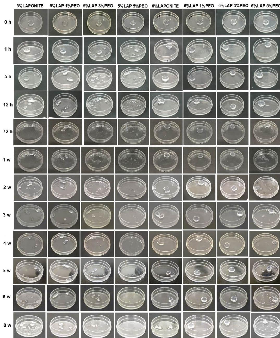
FIGURE 2.20: *Stability in PBS. Changes in weight were observed at the showed timepoints (obviously once the medium is removed) and at each time-point pictures were taken. Four samples for each composition were prepared and between them the most representative was chosen to be plotted. There is a visible trend: the higher the PEO concentration, the less stable is the material over time.*
