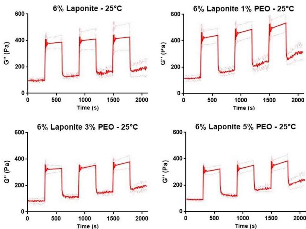
FIGURE 2.50: Multiple stress creep recovery test: loss modulus vs time. The test was performed at 25°C, for four compositions: 6% Laponite, 6% Laponite 1% PEO, 6% Laponite 3% PEO, 6% Laponite 5% PEO. For all of them  $G''$  is lower than  $G'$ , so the elastic portion is the main one compared to the viscous.
