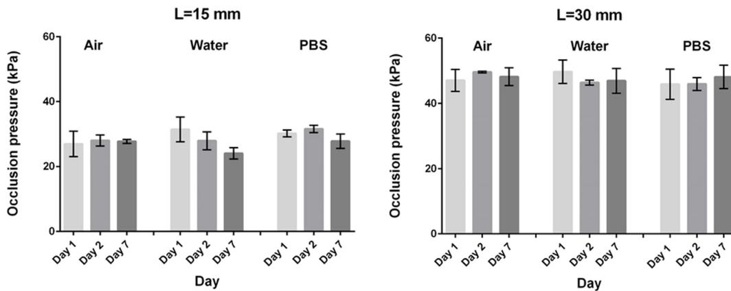
FIGURE 2.14: Occlusion pressure measurements in 1 mm tube, putting 15 mm (left figure) and 30 mm (right figure) of material inside the tube. The used media were air, water and PBS, the flow rate was 1 mL/min and the experiment was performed at 25°C. The occlusion pressure remained quite constant until day 7, except for the measurement in water, using 15 mm of 6% Laponite 1% PEO, for the last timepoint.
