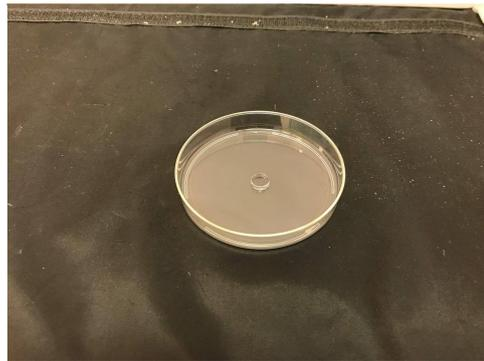
FIGURE 2.32: Final appearance of one of the cylindrical samples used for the compression test. The diameter is 1.5 cm, the height is 3.2 mm. The sample was prepared using a PMMA mold, made with the laser cutter.
