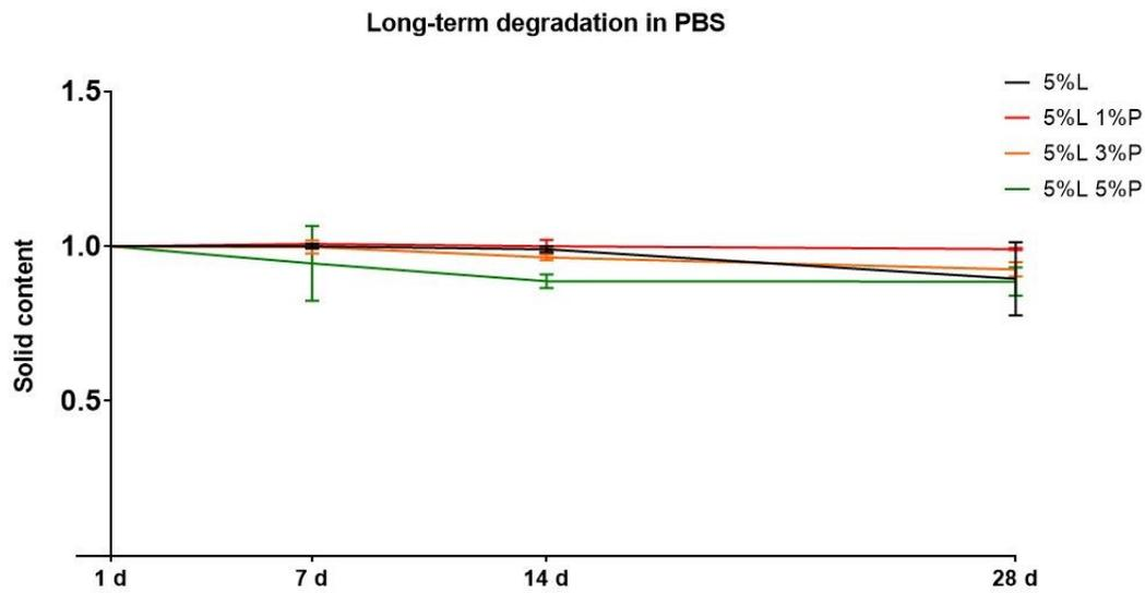
FIGURE 2.28: Degradation of gels with 5% Laponite in PBS until 28 days.
