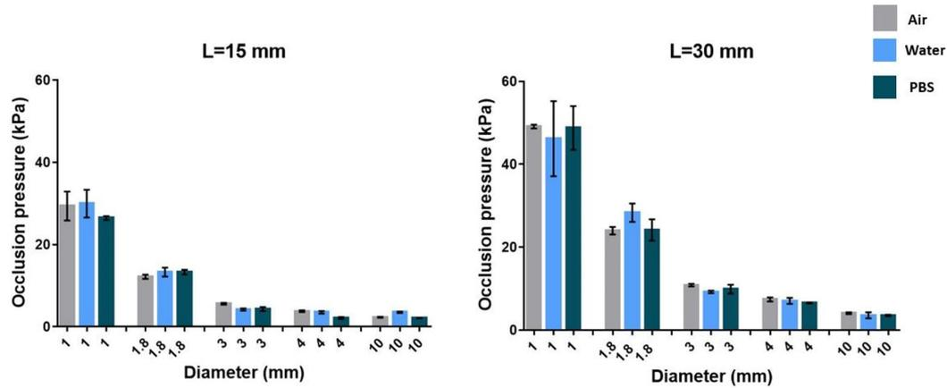
FIGURE 2.12: A summary of the values of occlusion pressure for 6% Laponite 1% PEO injecting two different lengths of material inside the tubes. The bar chart shows, as expected, that the occlusion pressure decreases for the larger tubes.
