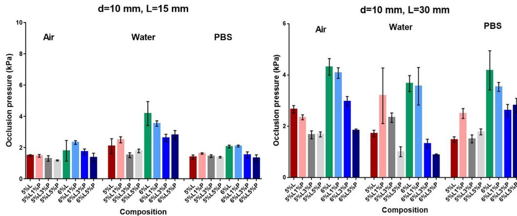
FIGURE 2.11: Occlusion pressure measurements in 10 mm tube, putting 15 mm (left figure) and 30 mm (right figure) of material inside the tube. Air, water and PBS were spilled against the blockage.
