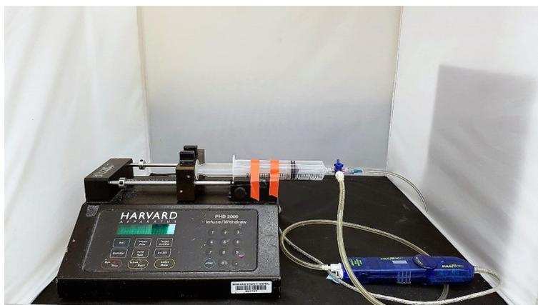
FIGURE 2.6: Experimental set up for occlusion pressure measurements. Syringe pump, Pasco Dual pressure sensor, transparent tube with the material inside to cause a blockage and all the connections are shown. The chosen flow rate for the medium that will flow against the material is 1 mL/min.
