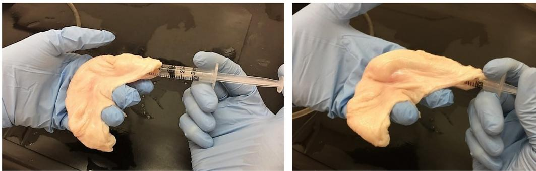
FIGURE 2.18: *Injecting the material inside a piece of Fallopian tube. The injection was done using a 3 mL syringe and pushing slowly the plunger to let the material be well distributed inside the tube.*
