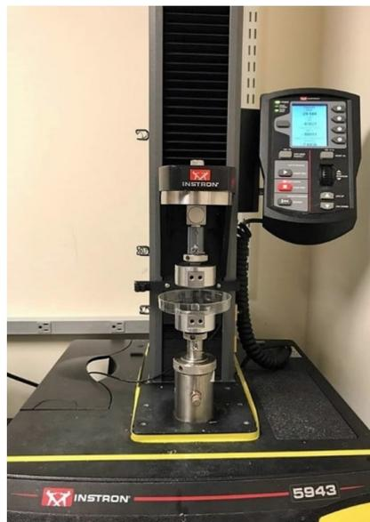
FIGURE 2.33: Experimental setup with the mechanical testing system, Instron 5943, and the Petri dish containing the sample under consideration.
