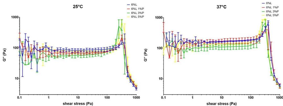
FIGURE 2.43: Loss modulus vs shear stress at 25°C and 37°C. Oscillatory stress sweep was conducted at 0.1-1000 Pa and 1 Hz. The curves are plotted on log-log plot. For all our materials  $G'$  is bigger than  $G''$  so the material behaves in theory like an elastic solid. 6% Laponite 3% PEO and 6% Laponite 5% PEO are softer materials but weaker than the other gels.
