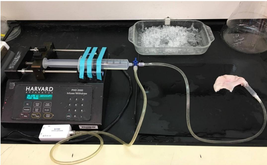
FIGURE 2.16: Experimental setup for ex-vivo occlusion pressure measurements. Syringe pump, Pasco wireless pressure sensor, homemade connector, piece of porcine oviduct and all the connections are shown. The chosen flow rate for the medium that will flow against the material is 20 ml/min, higher than the one used in vitro.
