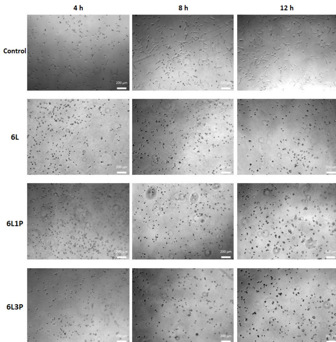
FIGURE 2.55: Bright-field images showing cells-material interaction. The biological effects of three different gels (6% Laponite, 6% Laponite 1% PEO, 6% Laponite 3% PEO) were tested. The control is only normal media. The time points are 4 h, 8 h, 12 h. A trend is visible: the higher the PEO content, the less cells adhere to the substrate.
