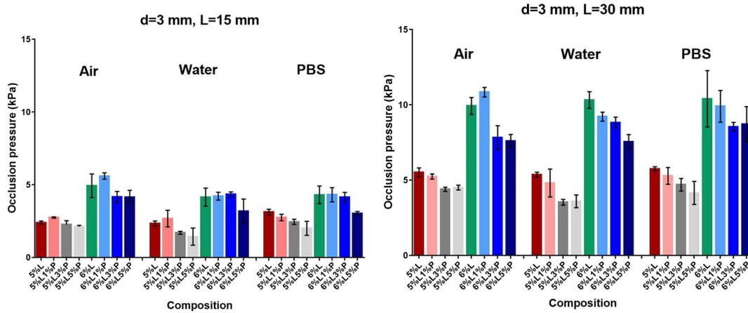
FIGURE 2.9: Occlusion pressure measurements in 3 mm tube, putting 15 mm (left figure) and 30 mm (right figure) of material inside the tube. Air, water and PBS were spilled against the blockage.
