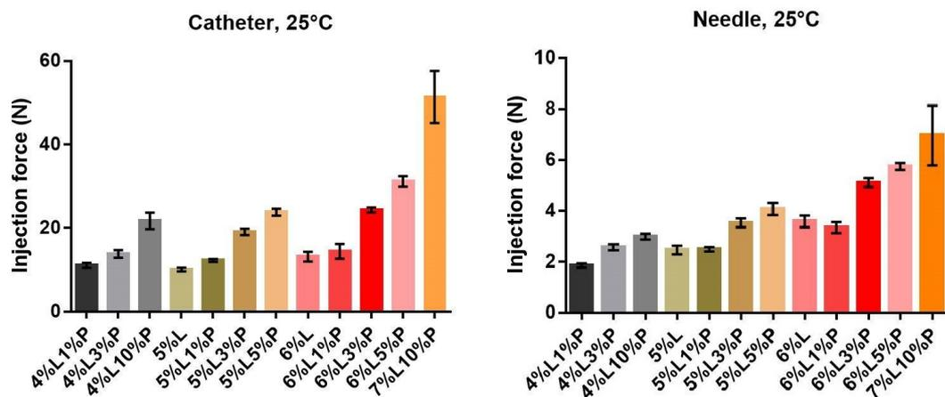
FIGURE 2.5: Injection force versus composition. Both for catheter and needle the trend is almost the same: the higher the percentage of Laponite, the less easy to inject. Additionally, from low to higher PEO concentration: the higher the PEO concentration, the higher the injection force
