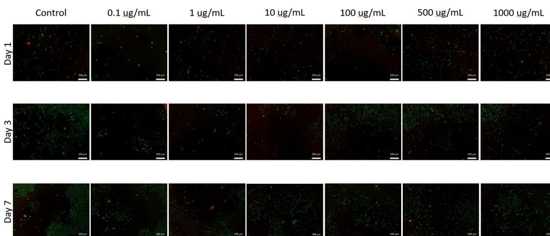
FIGURE 2.53: *Live/Dead Assay on 3T3 cells to evaluate the cytotoxicity of PEO putting directly the powder of the polymer inside the medium. These are the most representative pictures of all the wells. Unlike Laponite, the PEO gave us no problems of reflections and the live cells, in green, are easy to recognize from the red ones, which are dead cells.*
