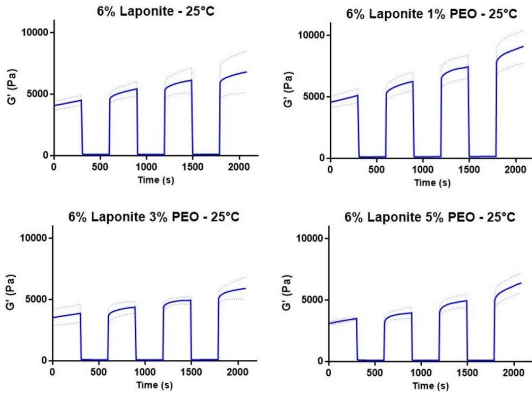
FIGURE 2.49: Multiple stress creep recovery test: storage modulus vs time. The test was performed at 25°C, for four compositions: 6% Laponite, 6% Laponite 1% PEO, 6% Laponite 3% PEO, 6% Laponite 5% PEO.
