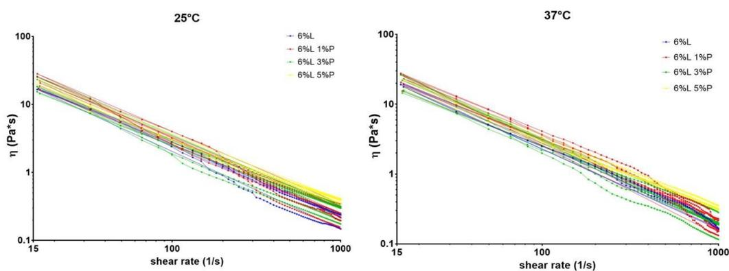
FIGURE 2.41: Viscosity profile of the evaluated gels at 25°C and at 37°C. These viscosity versus shear rate curves show the shear-thinning behaviour of our materials; this means that they can deform and behave like liquids when a stress is applied and fast recover their original nature.
