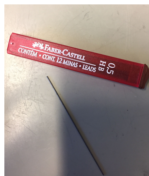
Figure 5.17: Pencil Graphite Electrode (PGE) (from Faber-Castell )
