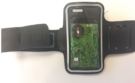
Figure 4.3: Wearable health monitoring device consisting of a flexible electronic PCB encapsulated in a arm-band case and connected to electrochemical sensors in direct contact with the subject's skin.
