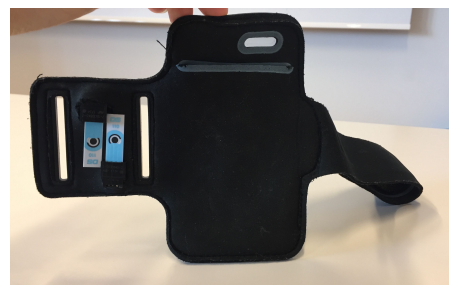
Figure 4.3: Wearable health monitoring device consisting of a flexible electronic PCB encapsulated in a arm-band case and connected to electrochemical sensors in direct contact with the subject's skin.
