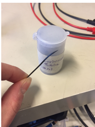
Figure 5.16: Pyrolyzes bamboo electrode (provided by Politecnico of Turin).
