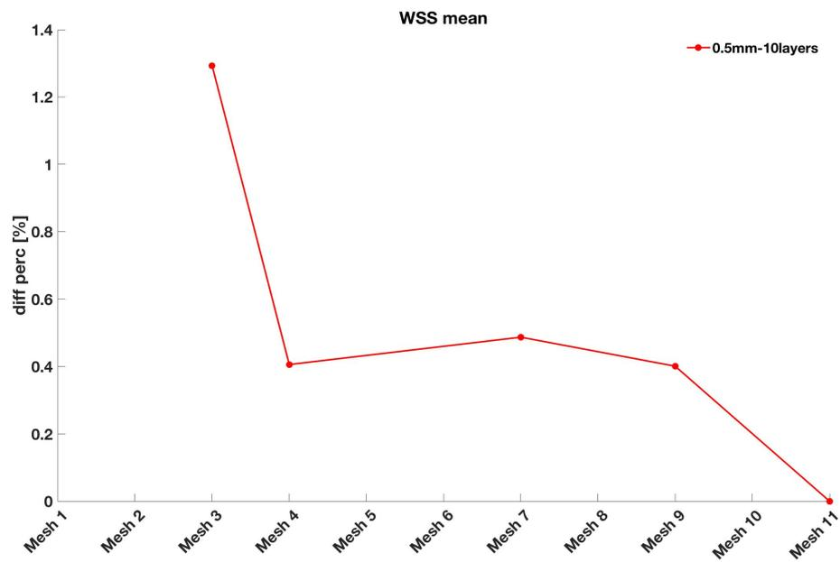
**Figure 2.6:** Percentage differences of mean WSS of only grids with 10 layers and thickness boundary layer of 0.5mm with respect to that of Mesh 11.
