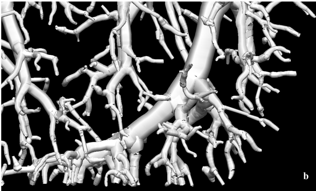
Figure 18: Effect of the smooth on CMGUI. (a) Venous tree before applying the smooth command; (b) Venous tree after the smooth
