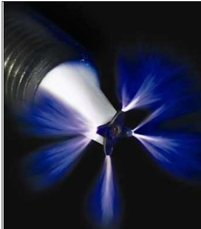
Figure 22. Corona charge igniter illustration [46]
