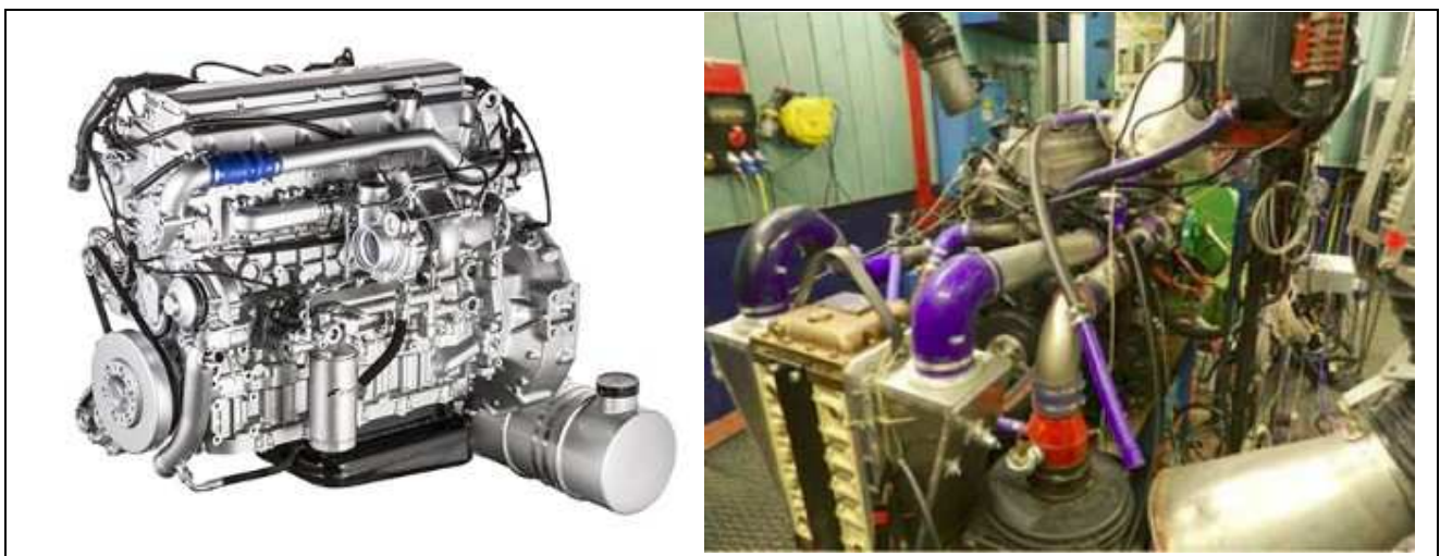
Figure 24. Currently available(on the left) and prototype version(on the right, test rig) FPT Cursor 8[32,50]
