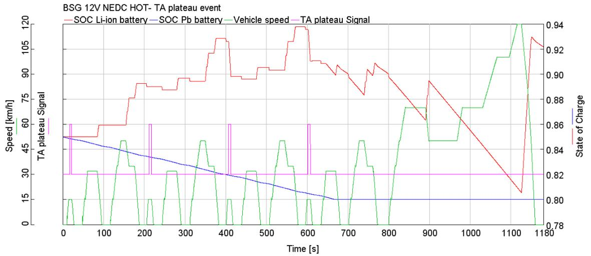
Figure 43: TA plateau event for BSG model in NEDC hot.
