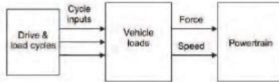
Figure 13: Flux diagram in a kinematic or backward simulator [22].
