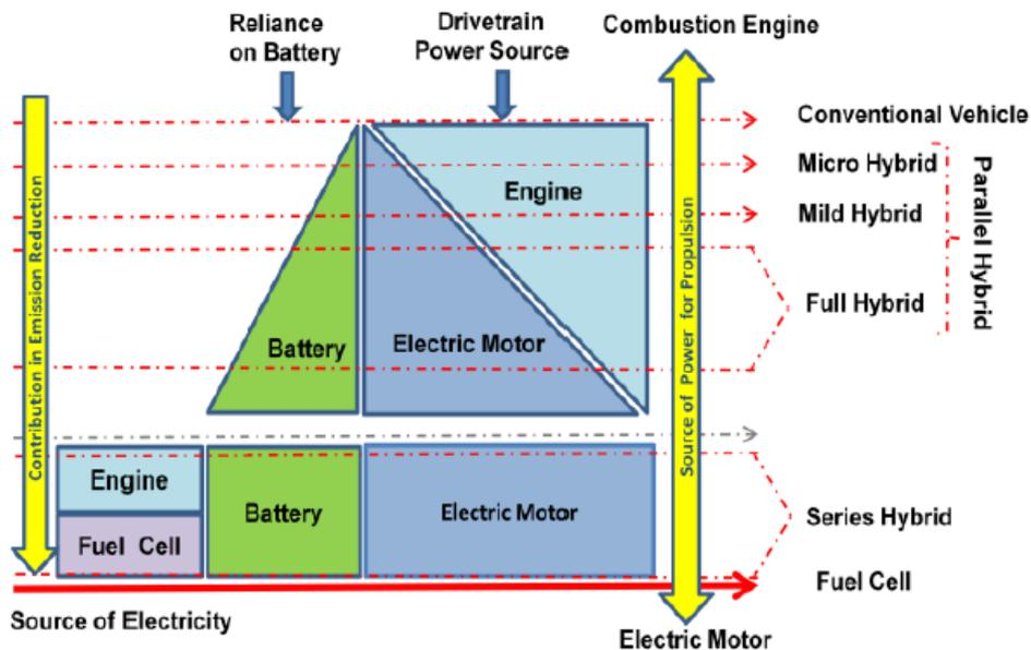
Figure 6: Classification of hybrid vehicles on degree of hybridization [15].
