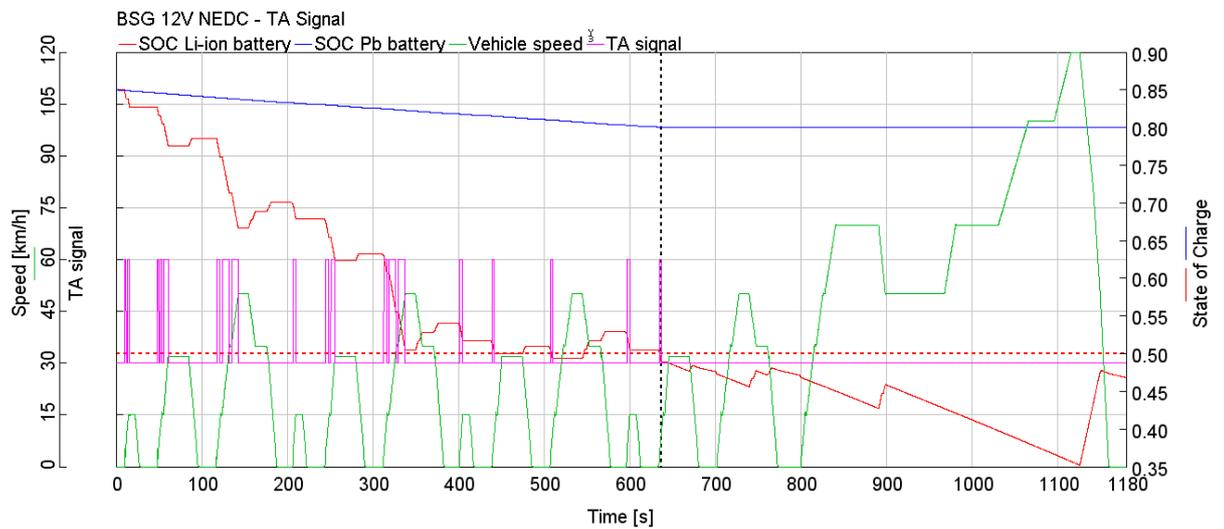
Figure 37: TA activation for BSG model (NEDC).
