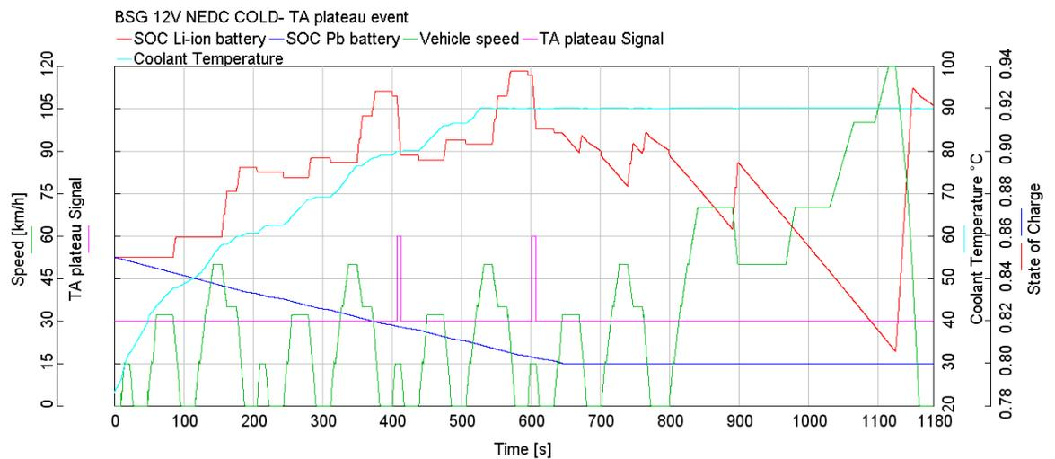
Figure 42: TA plateau event for BSG model in NEDC cold.
