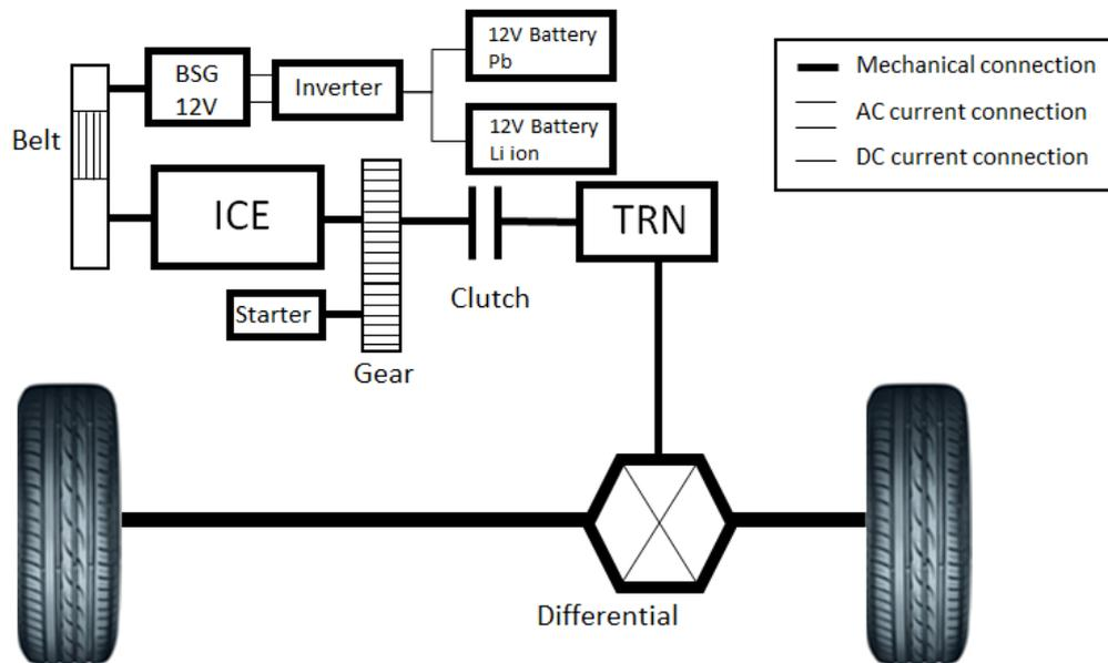
Figure 10: Architecture of BSG 12V.
