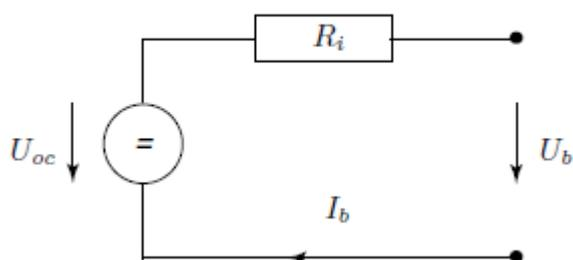
Figure 17: Open voltage circuit model, for the battery [17].
