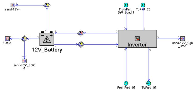
Figure 18: Battery subassembly for baseline and ESS model.
