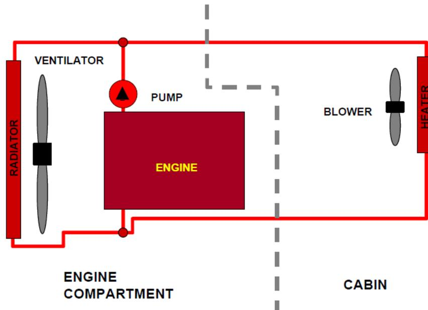
Figure 20: Scheme of the engine cooling system [23].
