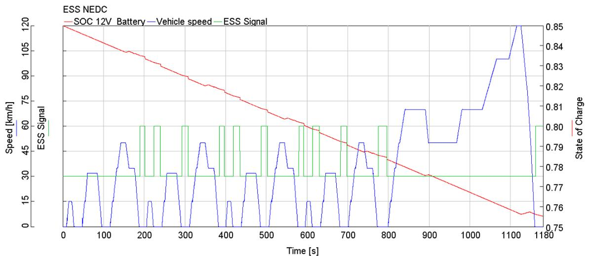
Figure 25: SOC, vehicle speed and ESS signal for ESS model (NEDC).
