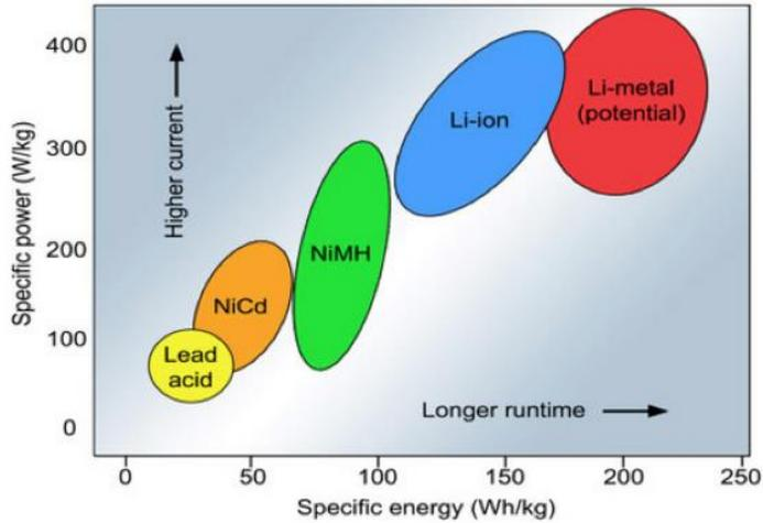
Figure 4: Energy density and specific energy for different type of batteries [14].
