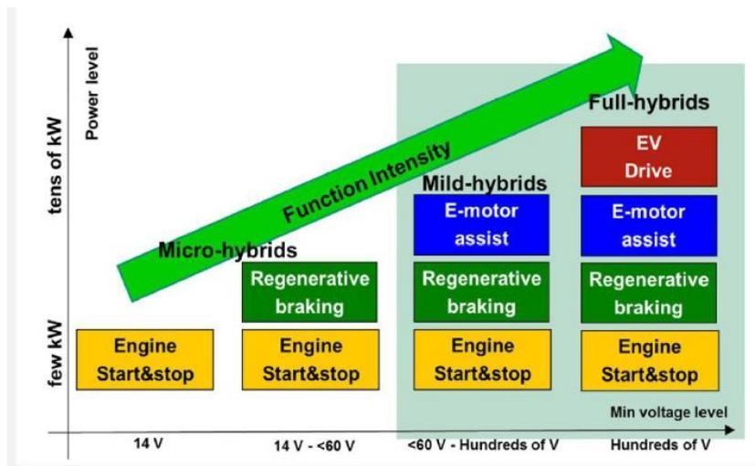
Figure 9: Hybrid functions and classification [2].
