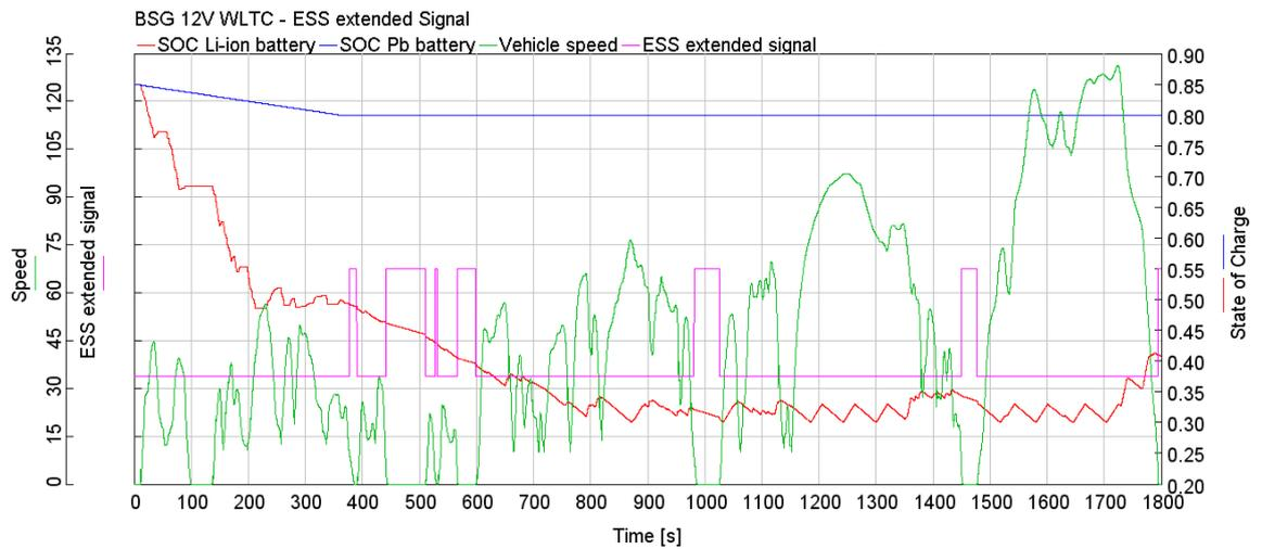
Figure 31: ESS events for BSG model (WLTC).
