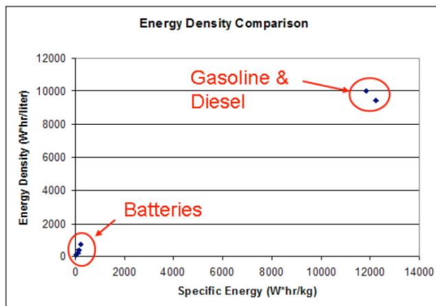
Figure 5 Comparison between batteries and hydrocarbon fuels, energy density and specific energy [14].
