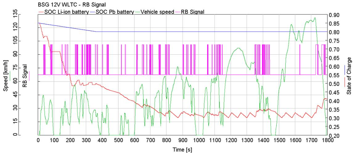
Figure 34: RB events for BSG model (WLTC).
