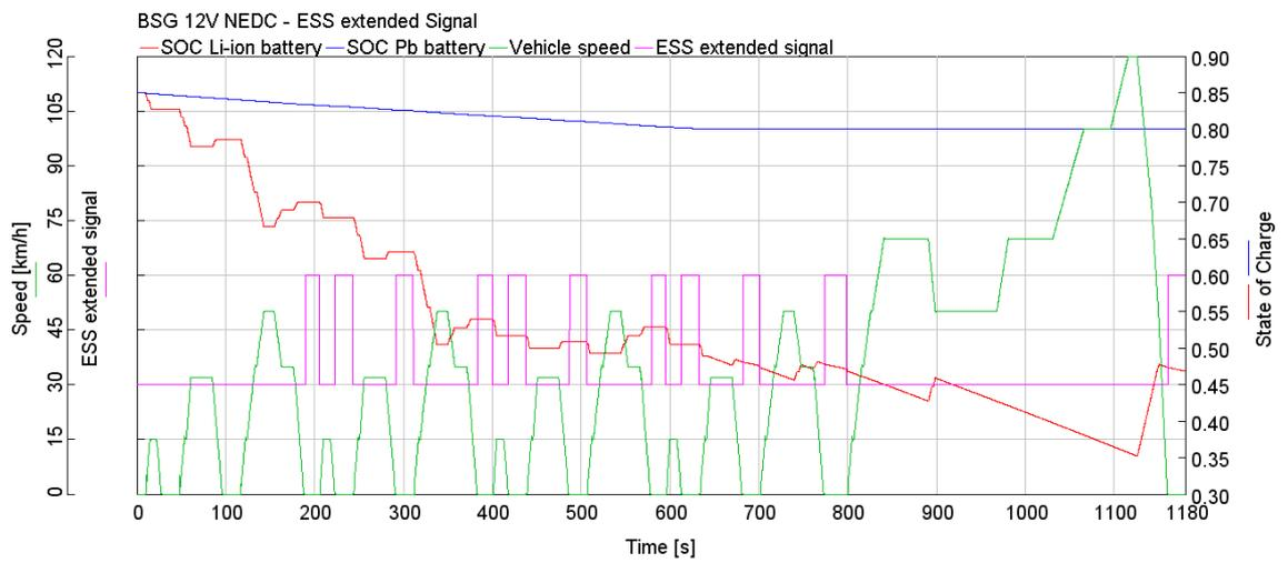
Figure 30: ESS events for BSG model (NEDC).
