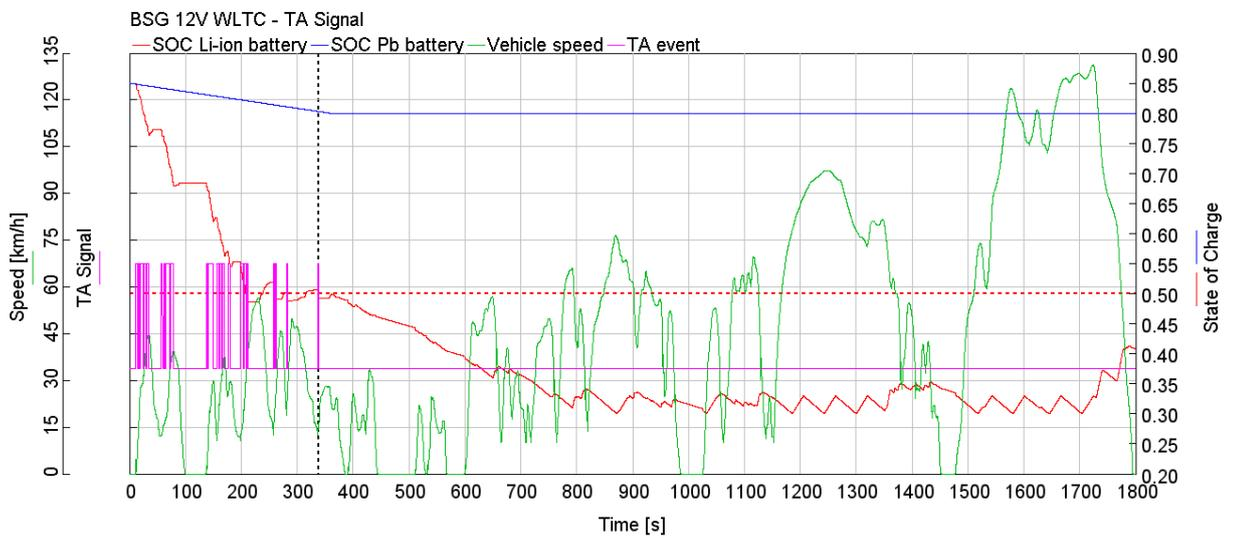
Figure 39: TA activation for BSG model (NEDC).
