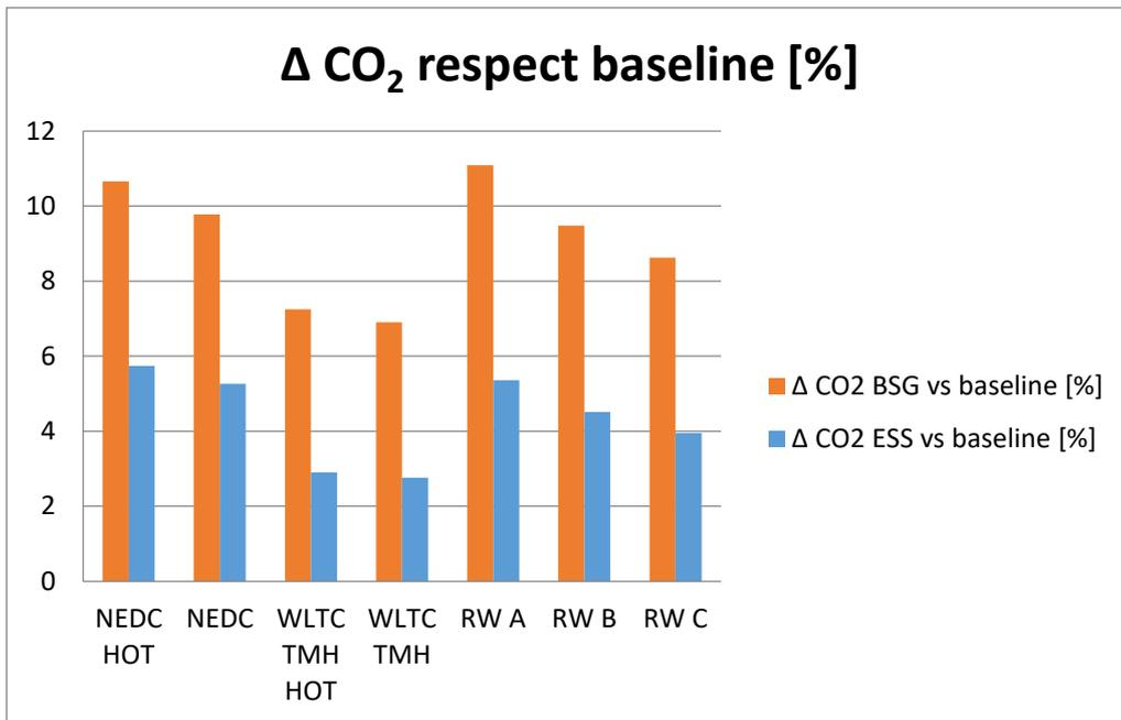
Figure 22: Differences in terms of CO<sub>2</sub> of ESS and BSG respect baseline, for each cycle.
