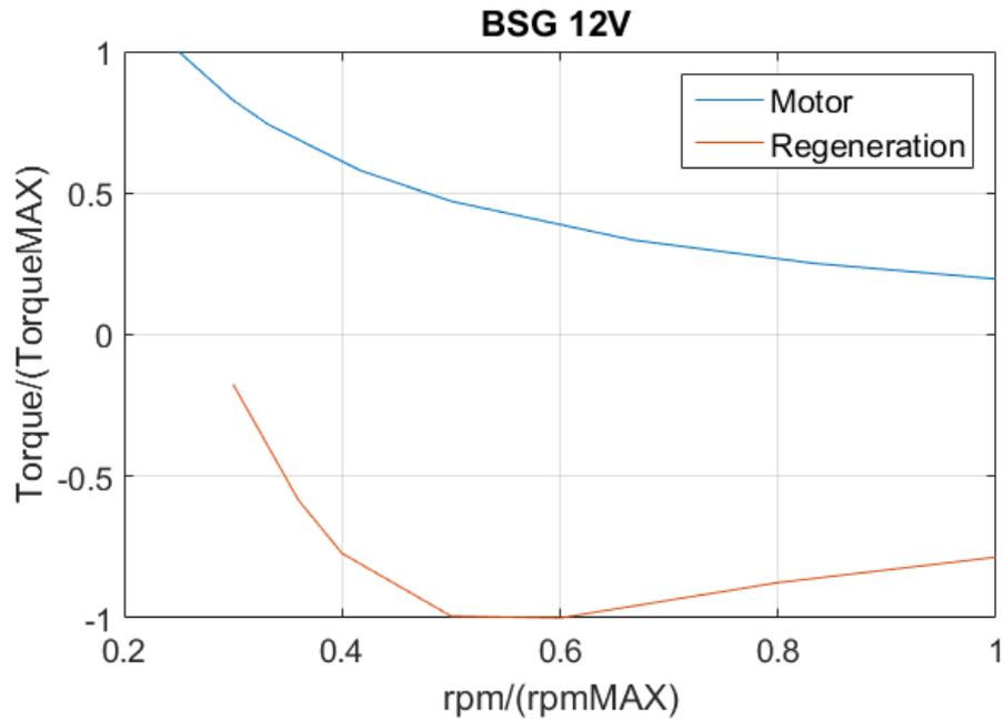
Figure 11: Characteristic of the EM normalized.
