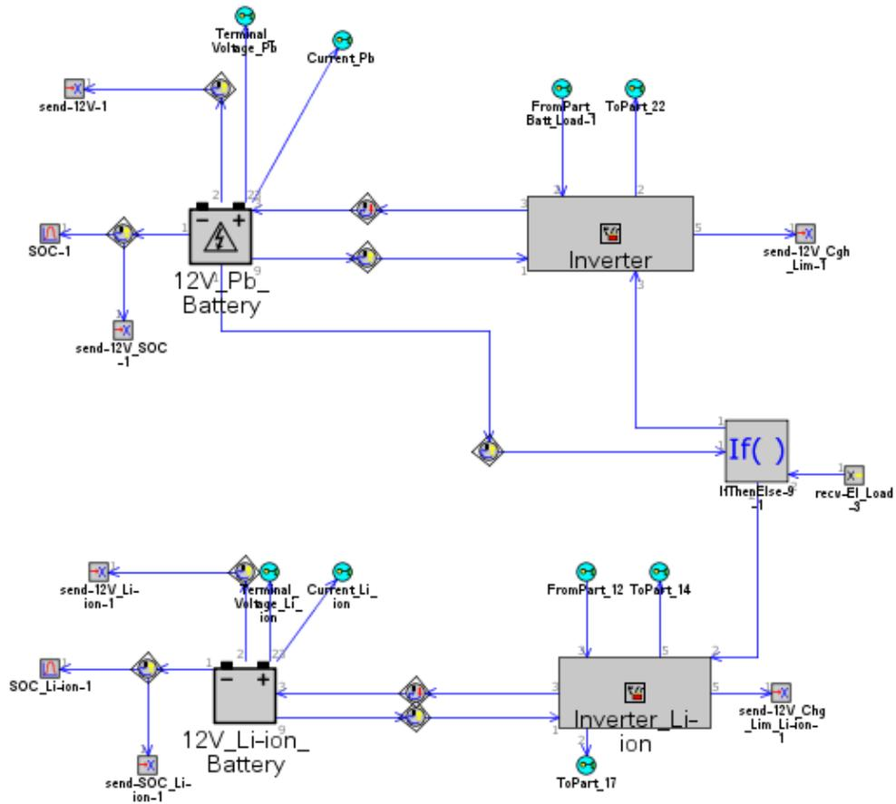
Figure 19: Battery subassembly for BSG model.
