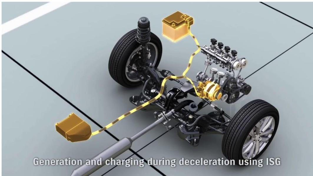
*Figure 12: SHVS system in generation mode.*
