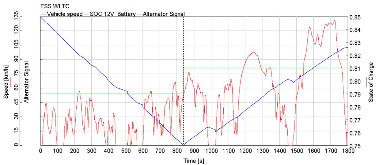
Figure 27: SOC, vehicle speed and alternator signal for ESS model (WLTC).
