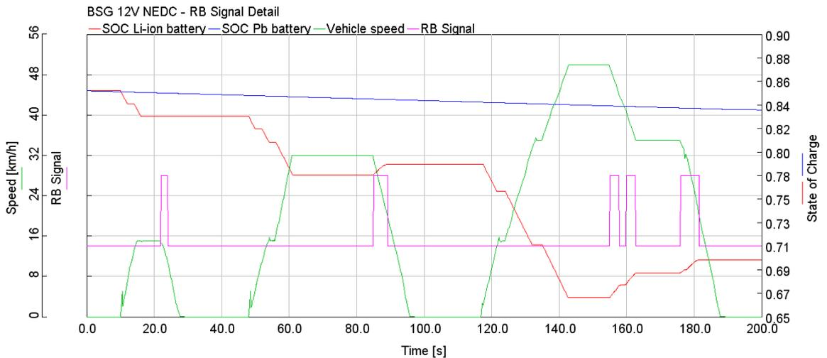
Figure 33: Detail for RB events for BSG model (NEDC).
