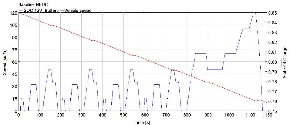
Figure 23: Vehicle speed and SOC for baseline model (NEDC).
