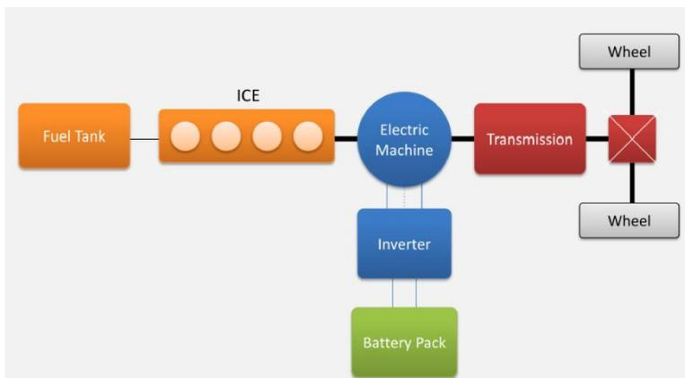
Figure 8: Parallel configuration for hybrid vehicle [2].
