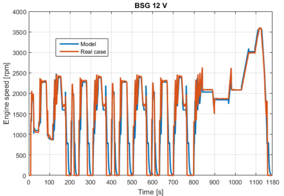
Figure 45: Engine speed real case and model for BSG (NEDC).
