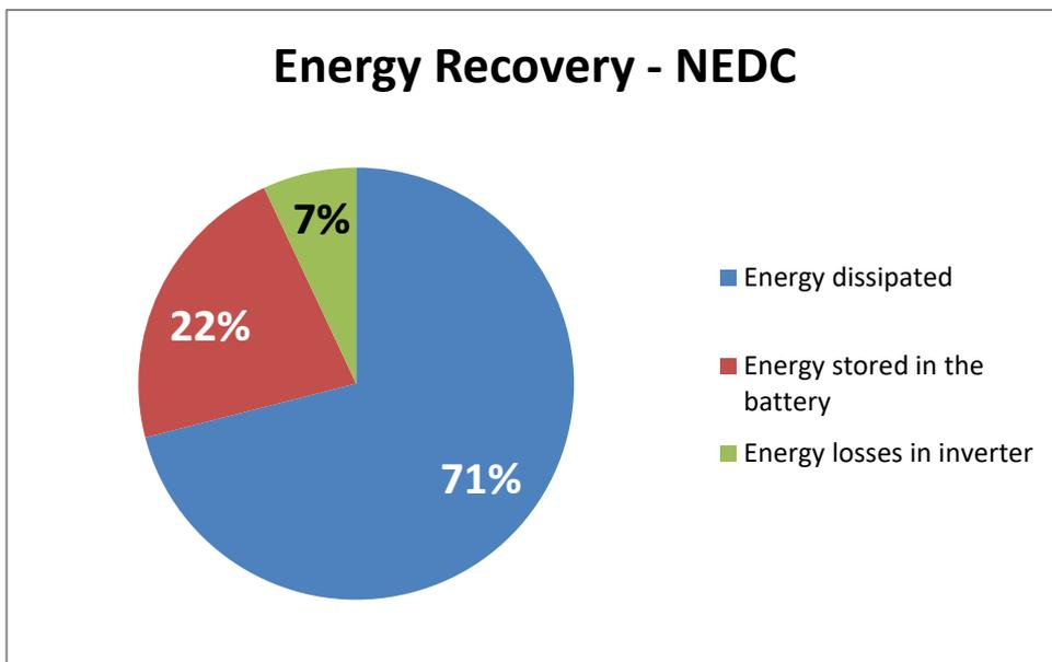
Figure 35: Pie chart of energy braking (NEDC).
