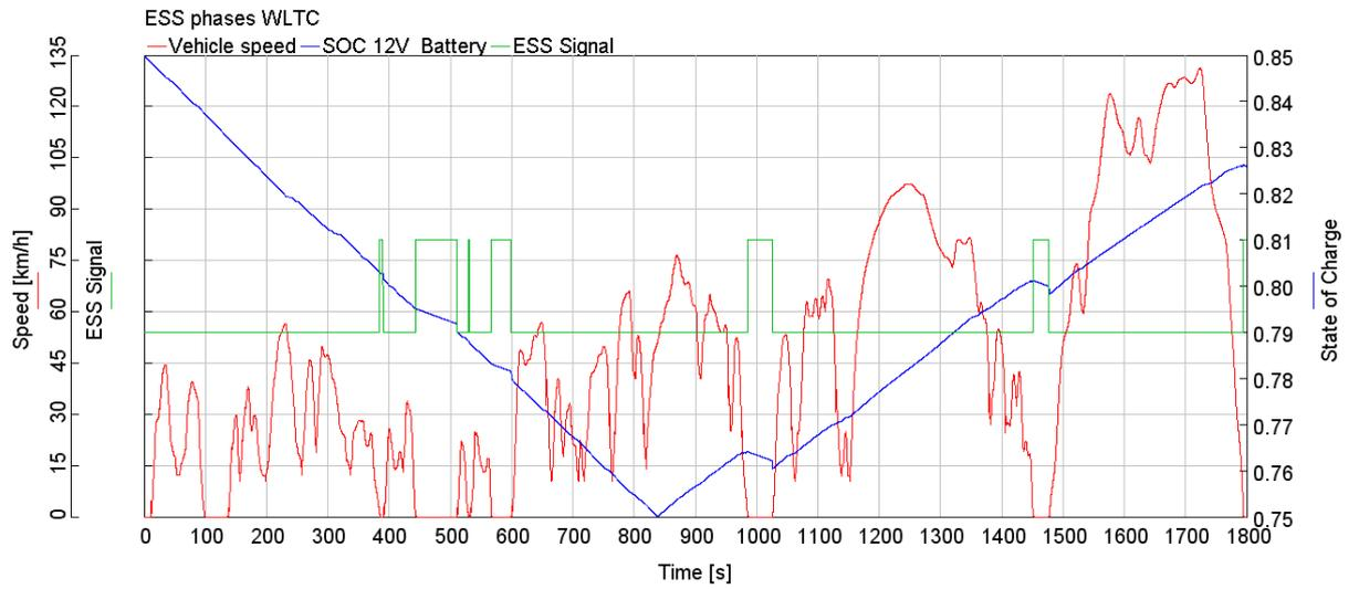
Figure 26: SOC, vehicle speed and ESS signal for ESS model (WLTC).
