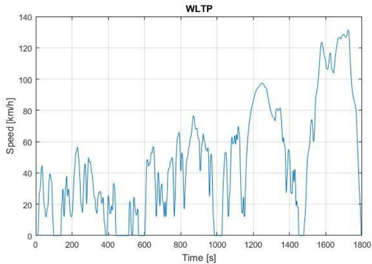
Figure 3: WLTC class 3 speed profile.
