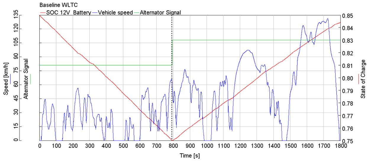
Figure 24: Vehicle speed, alternator signal and SOC for baseline model (WLTC).
