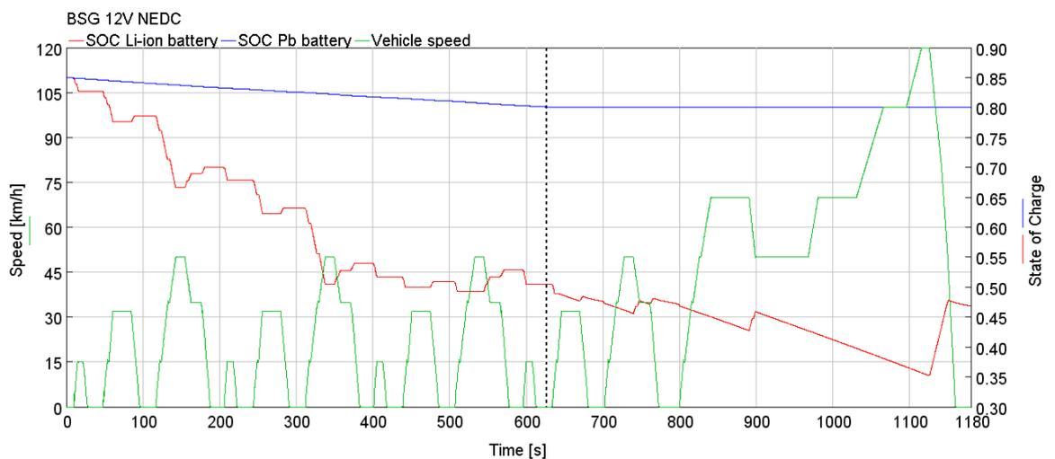
Figure 28: SOC, vehicle speed and alternator mode signal for BSG model (NEDC).
