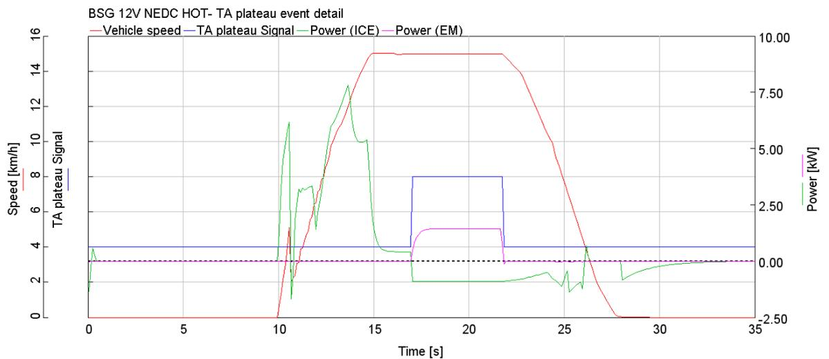
Figure 44: TA plateau event for BSG model in NEDC hot (detail).
