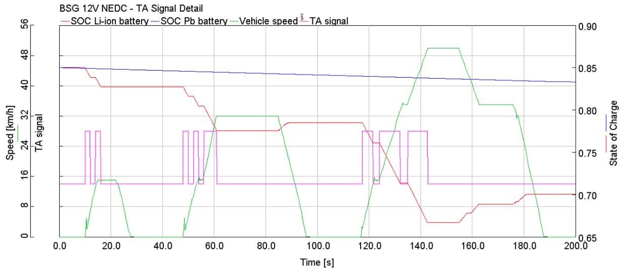
Figure 38: Detail for TA activation for BSG model (NEDC).
