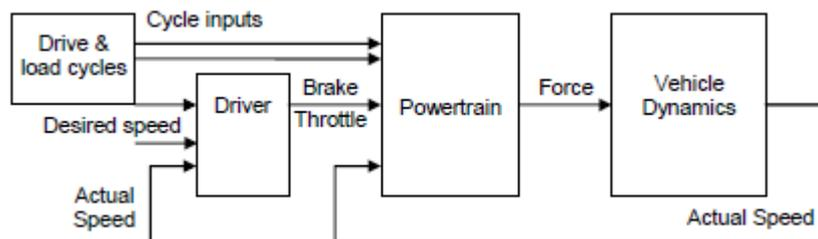
Figure 14: Flux diagram in a quasi-static approach simulator [22].
