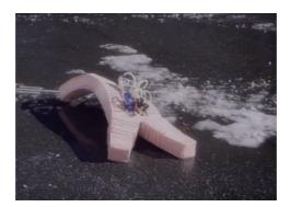
Figura 4.5: Soft robot in gomma siliconica
